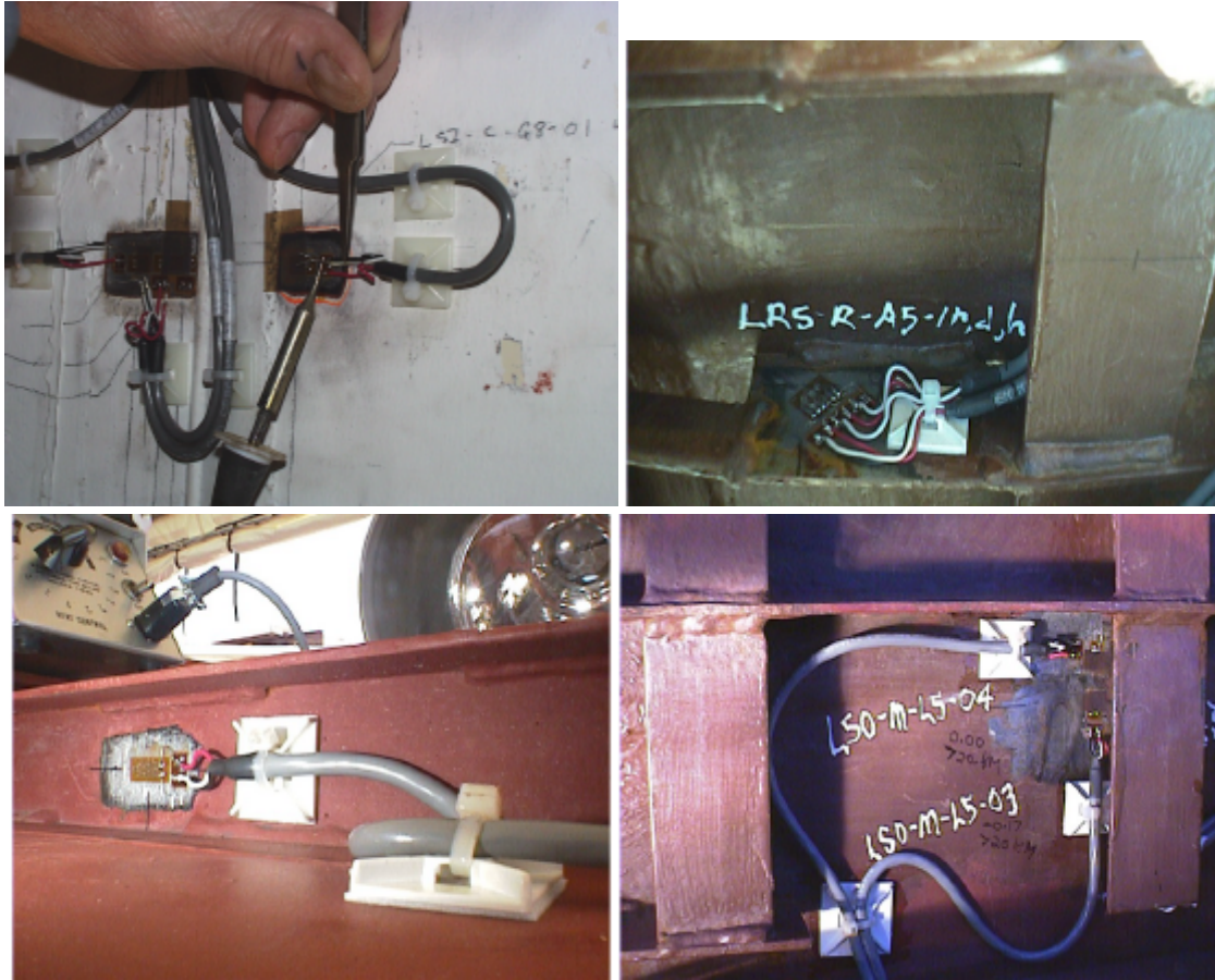
Figure 3.11 Liner and Liner Anchor Strain Gages
