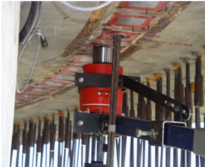
Figure 2.58 Tensioning Hardware Assembly and Load Cell
