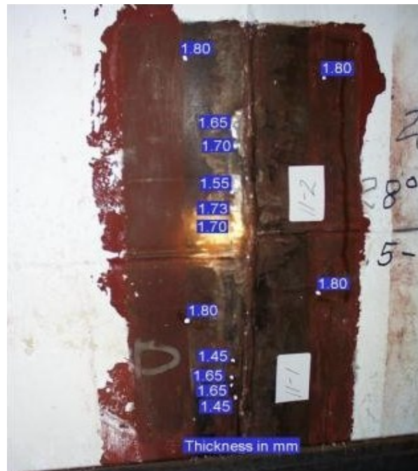
Figure 24. Liner thicknesses (in millimeters) measured ultrasonically in the vicinity of tear #11 (11-1 and 11-2).
