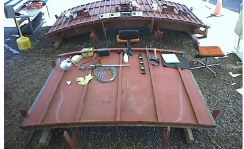
Figure 2.37 Liner Panel Instrumentation
