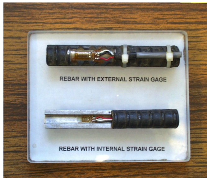
Figure 3.9 Sample Rebar and Gage Bar Strain Gages
