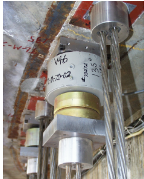
Figure 2.58 Tensioning Hardware Assembly and Load Cell
