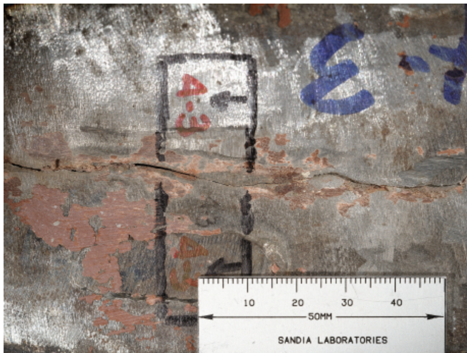
Figure 54. Details of inside (top) and outside (bottom) liner features in region of tear #4-3 metallographic cross-section (arrows begin at plane of section and indicate view direction).
