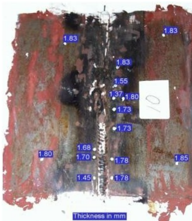
Figure 28. Liner thicknesses (in millimeters) measured ultrasonically in the vicinity of tear #10.
