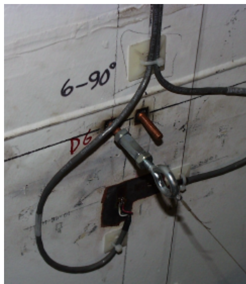
Figure 3.2 CPOT Mounted on Instrumentation Frame and Attachment to PCCV Liner
