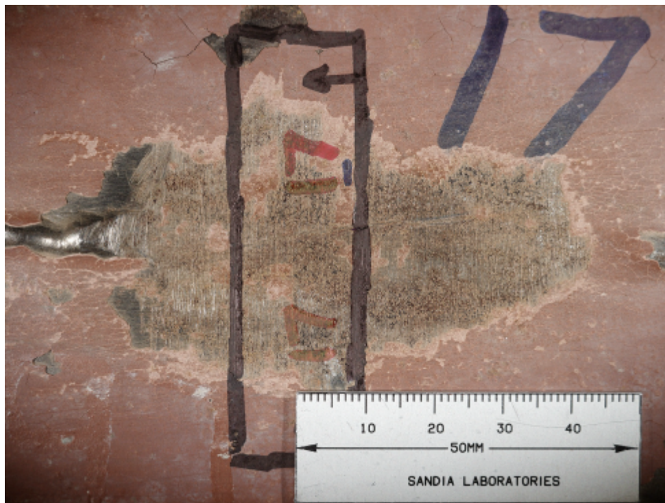
Figure 59. Details of inside (top) and outside (bottom) liner features in region of tear #17 metallographic cross-section (arrows begin at plane of section and indicate view direction).
