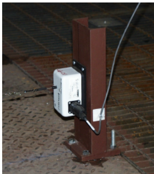
Figure 3.2 CPOT Mounted on Instrumentation Frame and Attachment to PCCV Liner
