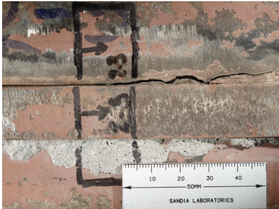
Figure 52. Details of inside (top) and outside (bottom) liner features in region of tear #2-3 metallographic cross-section (arrows begin at plane of section and indicate view direction).
