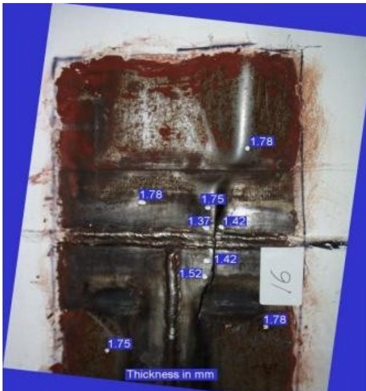
Figure 30. Liner thicknesses (in millimeters) measured ultrasonically in the vicinity of tear #16. Note distance of tear from vertical weld and extensive buckling above tear.
