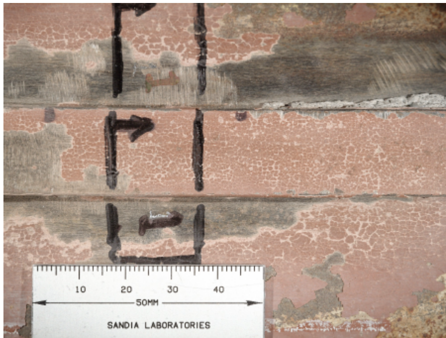
Figure 49. Details of inside (top) and outside (bottom) liner features in region of tear #1 metallographic cross-section (arrows begin at plane of section and indicate view direction).
