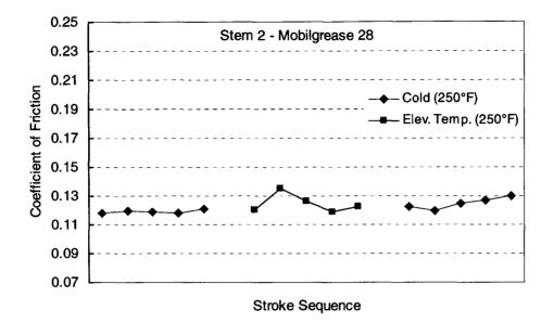
Figure 10. Elevated temperature test for Stem 2 with Mobil Mobilgrease 28.
