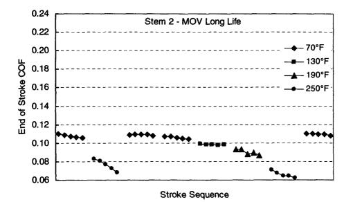
Figure 14. End-of-stroke stem nut friction at elevated temperature for Stem 2 with MOV Long Life.
