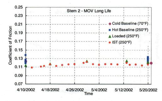
Figure 17. Aging test time line for Stem 2 with MOV Long Life.
