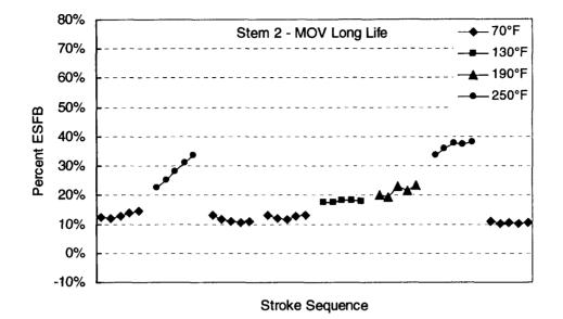
Figure 15. End-of-stroke friction behavior at elevated temperature for Stem 2 with MOV Long Life.
