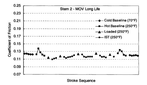
Figure 16. Aging test stroke sequence for Stem 2 with MOV Long Life.
