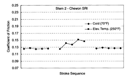
Figure 7. Elevated temperature test for Stem 2 with Chevron SRI.
