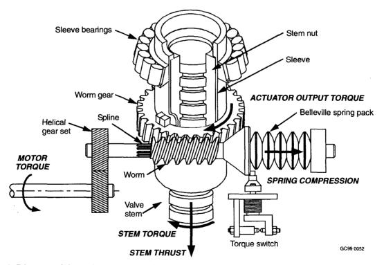
Figure 1. Diagram of the main components inside an actuator gearbox.
