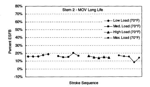
Figure 12. End-of-stroke friction behavior at various loads for Stem 2 with MOV Long Life.
