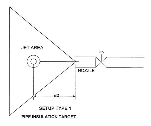
Figure A-3 Target Mount Geometry
