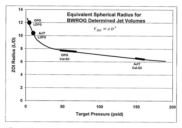
Figure 3-3 Equivalent Spherical Radius Dependence on Insulation Destruction Pressure
