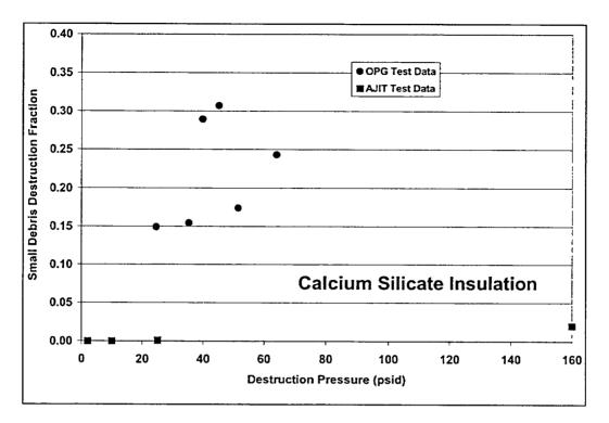
Figure 3-4 Small Debris Destruction Fractions for Calcium-Silicate Insulation
