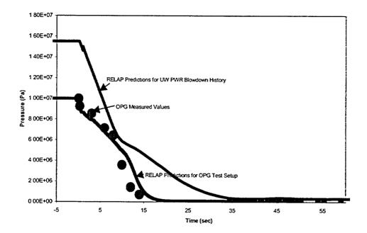
Figure 3-1 Comparison of RELAP Predictions with OPG Measurements for the Tank Pressure During Blowdown
