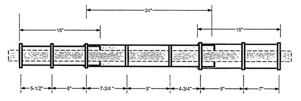
Figure A-4 Typical Band Configuration for Seam Offset Tests
