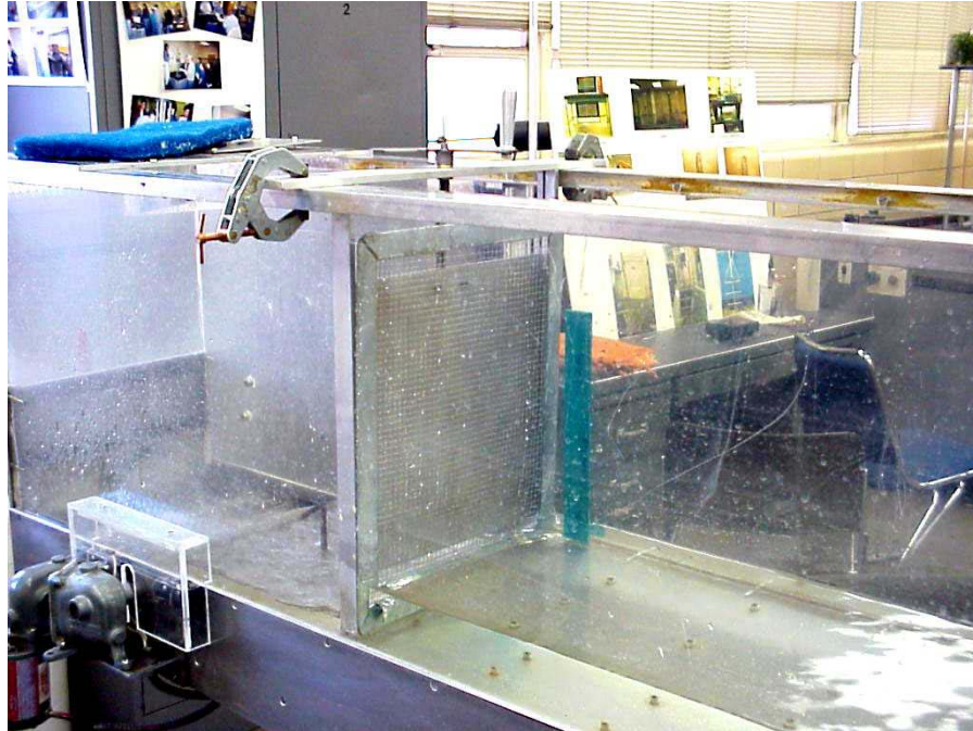
Fig. A-3. Outlet screen in the small flume test section.
