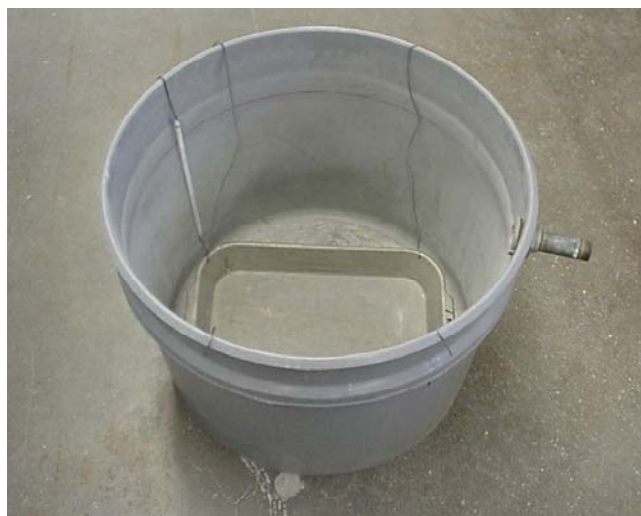
Fig. A-19. Plastic cylinder used in dissolution tests.
