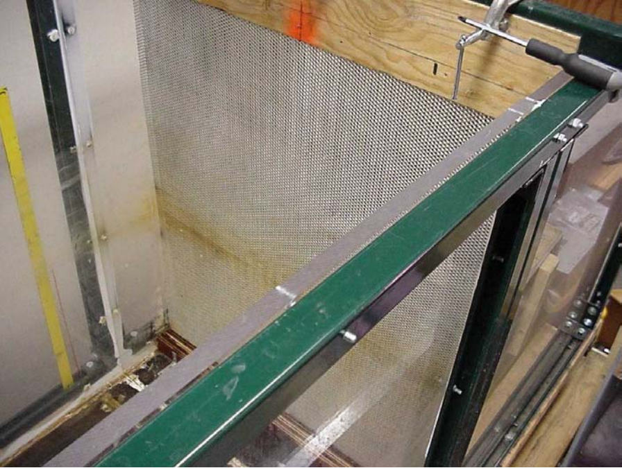
Fig. A-11. Test section exit screen.
