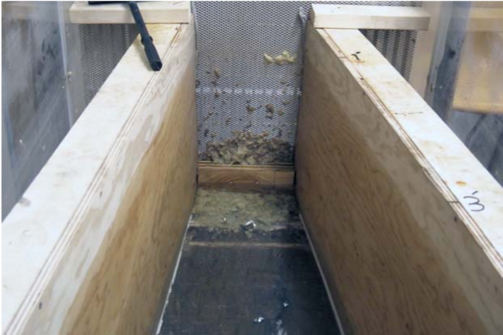
Fig. A-14. Test obstruction "curb" in converging test section.
