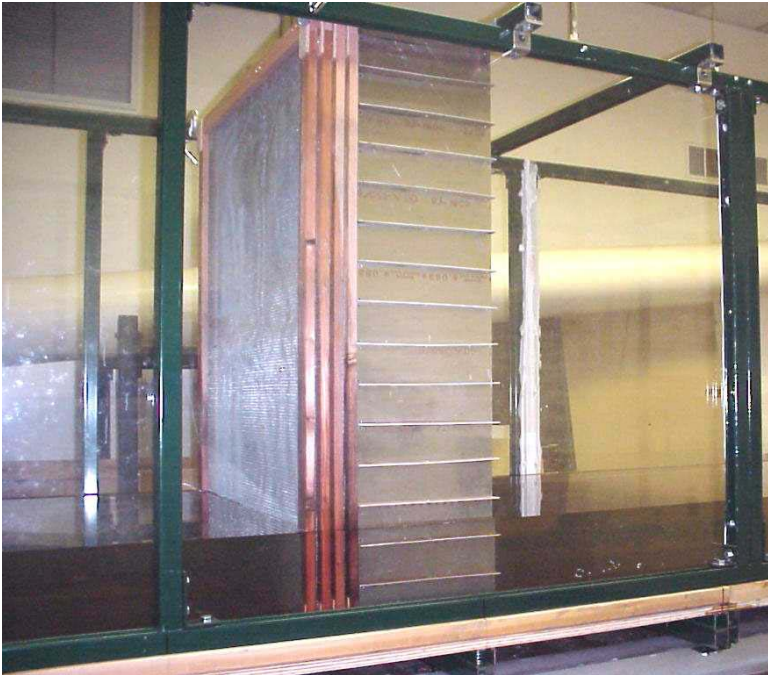
Fig. A-8. Photograph of equipment for 'Configuration A' inlet flow conditioning.
