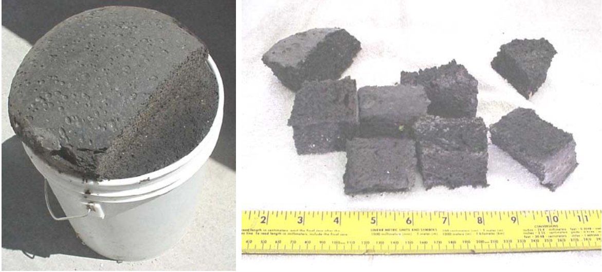
Fig. 3.9. Silicone foam insulation material (as foamed and pieces tested).
