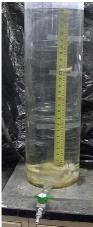
Fig. A-18. Plexiglas water column used in terminal settling velocity measurements.
