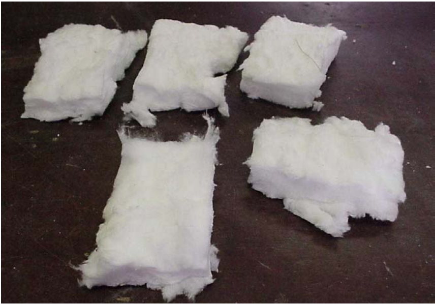
Fig. 3.3a. Kaowool insulation cut into 4-in. x 6-in. pieces.
