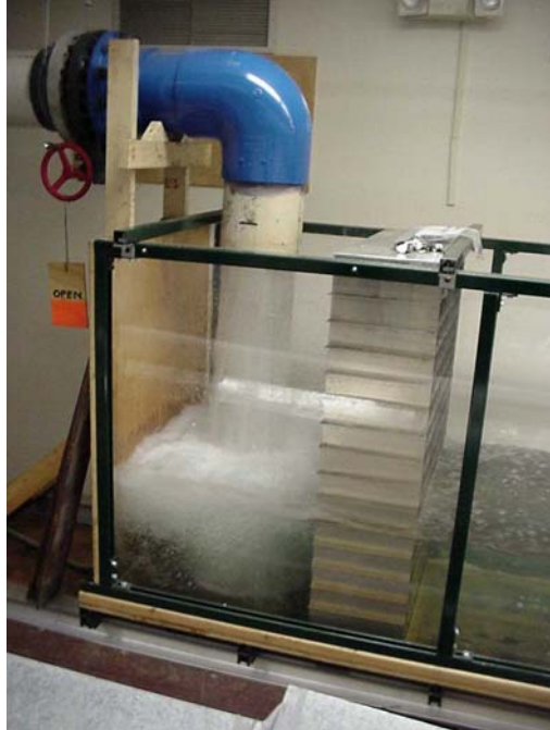
Fig. A-9. Photograph of “Configuration B” inlet flow conditioning.
