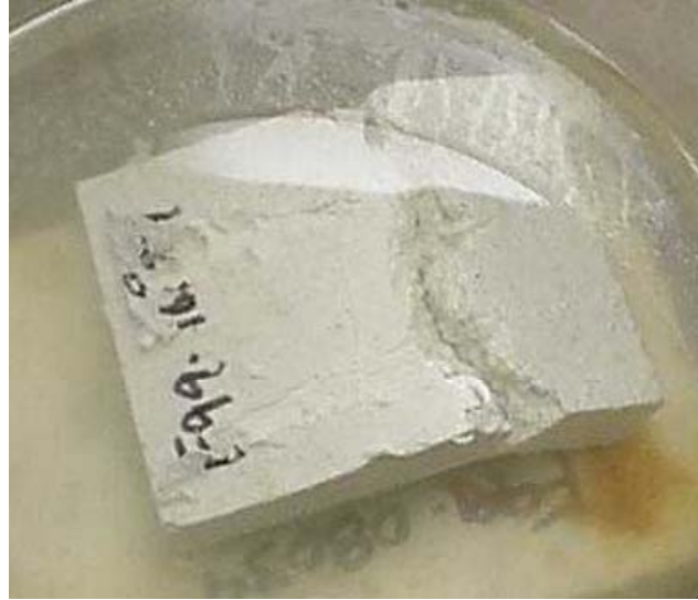
Fig. 3.8b. Wet broken piece of Marinite.
