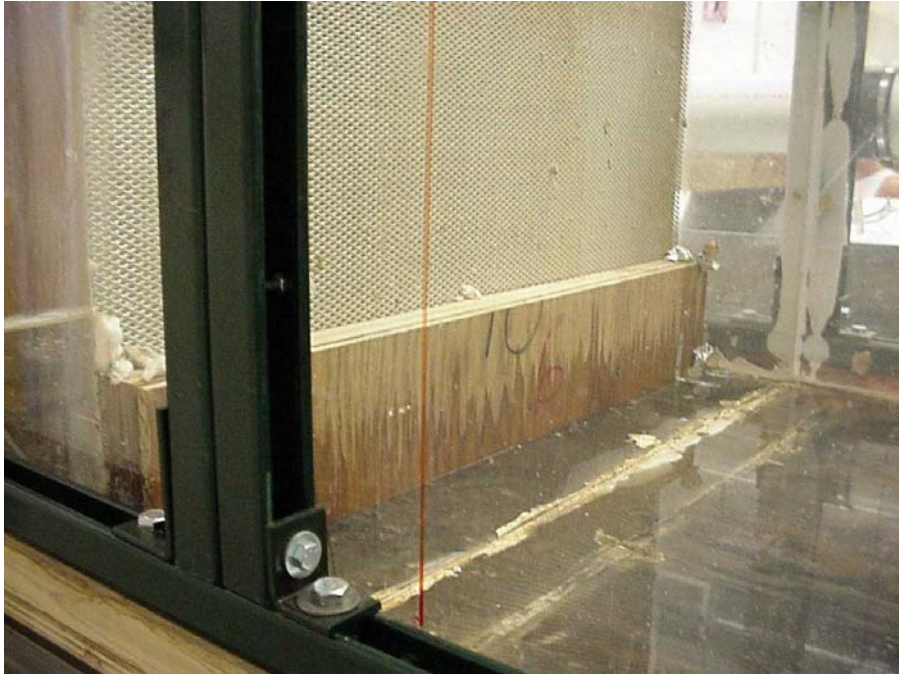
Fig. A-13. Test obstruction "curb" in standard test section.
