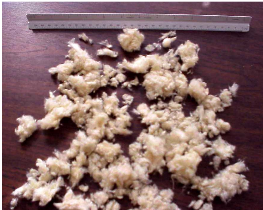
Fig. 3.1. Typical Nukon fiberglass insulation debris used in transport testing.
