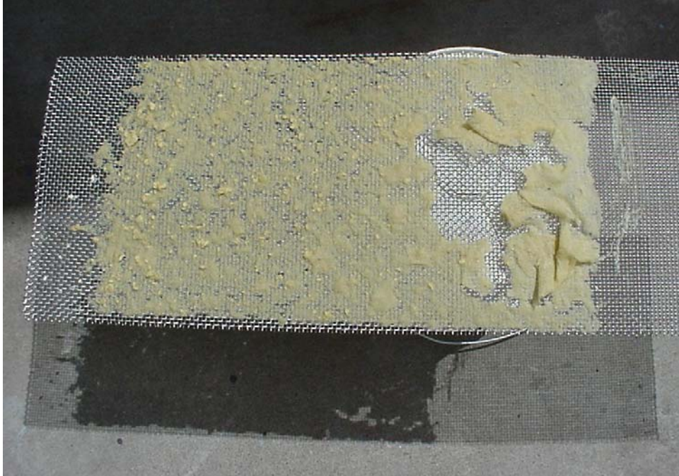
Fig. 3. Screen of 1/8-in. Mesh Opening Obstructed by Calcium-Silicate.
