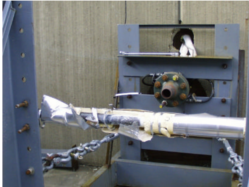
Figure D9 11-D seam at 45° Back View
