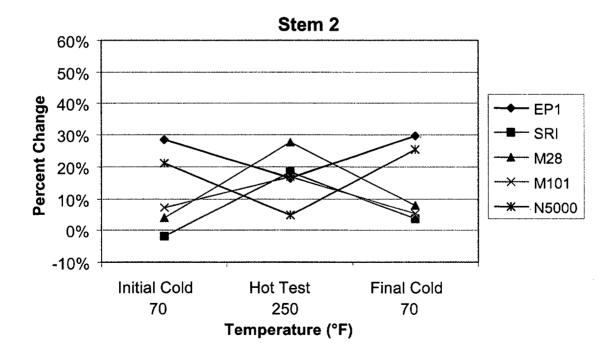
Figure C-6. End of stroke friction behavior for the single step tests with Stem 2.
