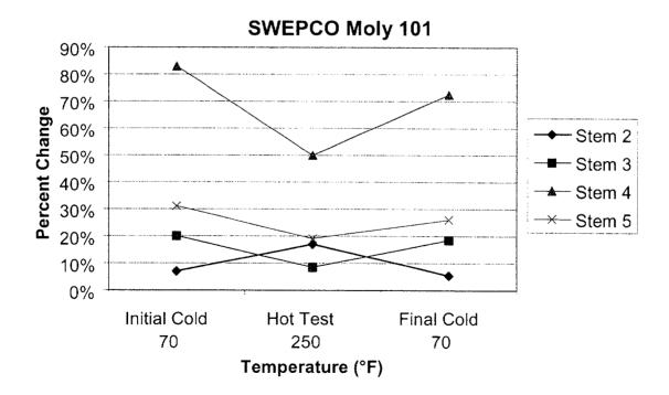
Figure C-4. End of stroke friction behavior for the single step tests with SWEPCO Moly 101.
