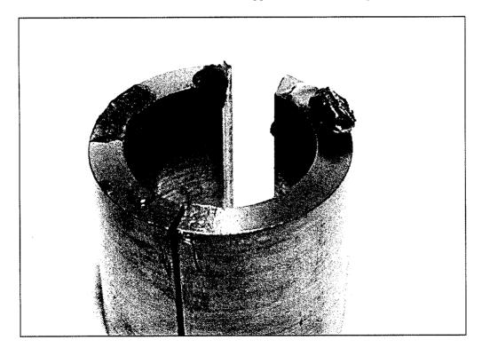
Figure A-67. Several drips of clear and silver-colored portions of the N-5000 landed on the stem spacer.
