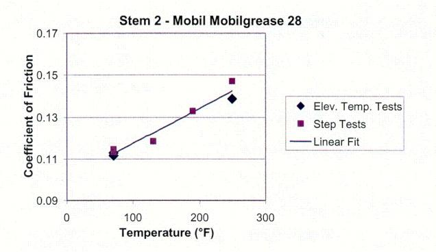
Figure B-9. The change in stem nut friction for stem 2 with Mobil 28 at elevated temperature.
