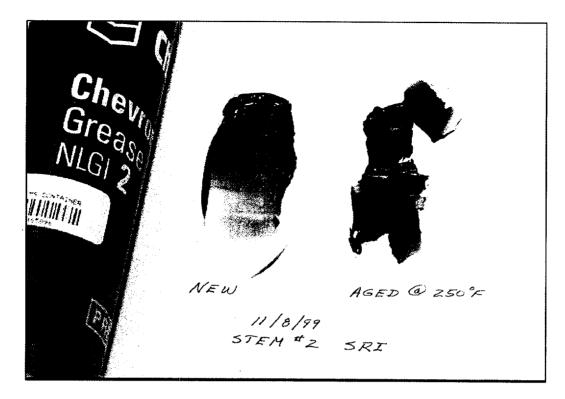
Figure A-51. Chevron SRI smear comparison.
