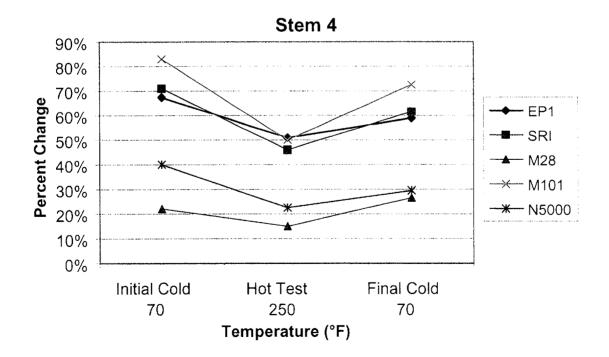
Figure C-8. End of stroke friction behavior for the single step tests with Stem 4.
