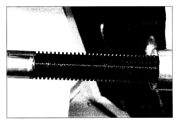
Figure A-59. A thin coat of Moly 101 was applied to each stem.
