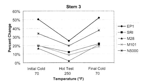
Figure C-7. End of stroke friction behavior for the single step tests with Stem 3.
