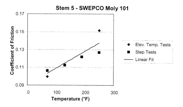
Figure B-16. The change in stem nut friction for stem 5 with Moly 101 at elevated temperature.
