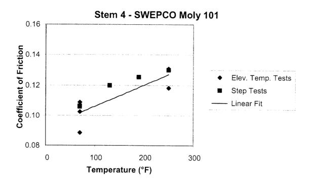
Figure B-15. The change in stem nut friction for stem 4 with Moly 101 at elevated temperature.
