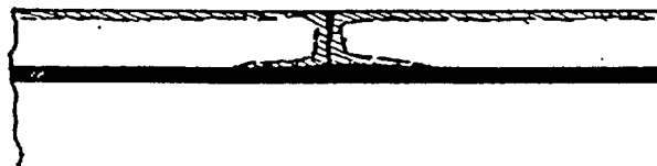
Carbon dioxide can penetrate into concrete where it has cracked, and along the reinforcement where is locally debonded.
