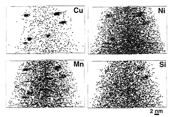
Figure 1. Atom maps of the solute distribution in weld 73 after neutron irradiation to a fluence of  $2 \times 10^{23}$  n m<sup>-2</sup>.
