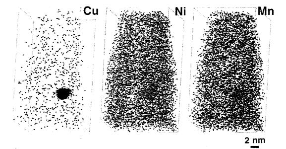
Figure 4. Atom maps of the solute distribution in weld 73 after neutron irradiation to a fluence of  $2 \times 10^{23}$  n m<sup>-2</sup> and anneal for 168 h at 454°C.
