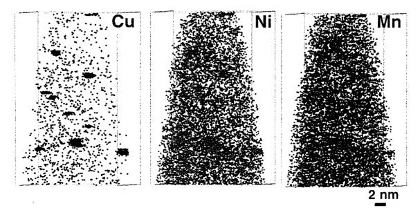
Figure 2. Atom maps of the solute distribution in weld 73 after neutron irradiation to a fluence of  $2 \times 10^{23}$  n m<sup>-2</sup> and anneal for 0.5 h at 454°C.
