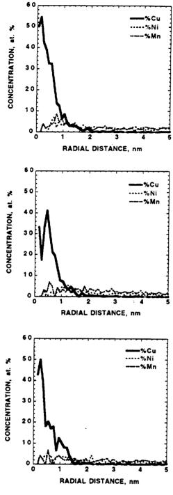
Figure 9. Radial concentration distributions of three copper-enriched precipitates in weld 73 after neutron irradiation to a fluence of  $2 \times 10^{23}$  n m<sup>-2</sup> and anneal for 1 h at 454°C.
