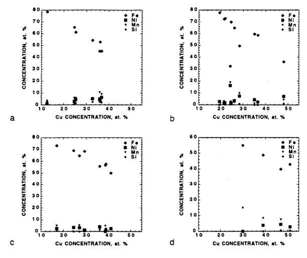
Figure 6. Concentration correlation of the copper-enriched precipitates in weld 73 after (a) neutron irradiation to a fluence of  $2 \times 10^{23}$  n m<sup>-2</sup>, (b) anneal for 0.5 h, (c) anneal for 1 h, and (d) anneal for 168 h at 454°C.
