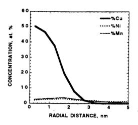
Figure 10. Radial concentration distribution of a copper-enriched precipitate in weld 73 after neutron irradiation to a fluence of  $2 \times 10^{23}$  n m<sup>-2</sup> and anneal for 168 h at 454°C.
