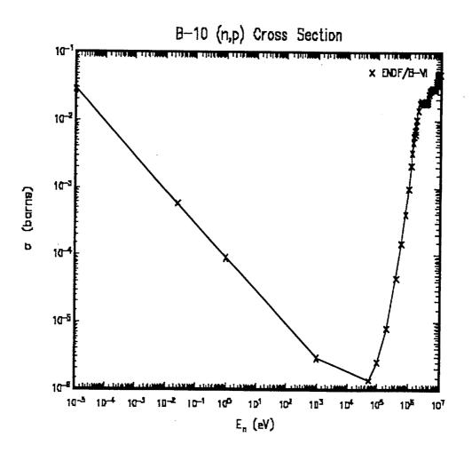
Figure 3.1 <sup>10</sup>B (n,p) Cross Section as a Function of Neutron Energy
