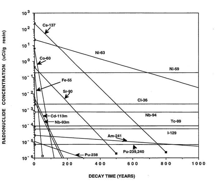
Figure 5.4 Change in Radionuclide Concentration with Time in Crystal River RWCU Resin
