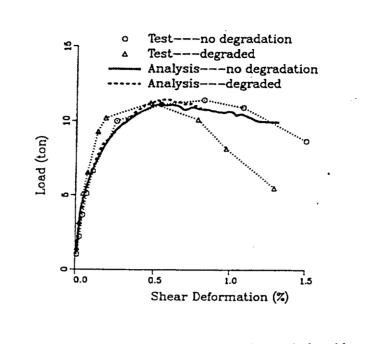
Fig. 21: Comparison of Load-Deformation Relationships
