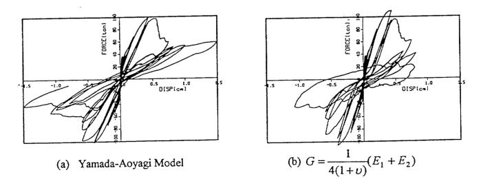
Fig. 16: Effects of Different Models for Shear Transfer Across Cracks
