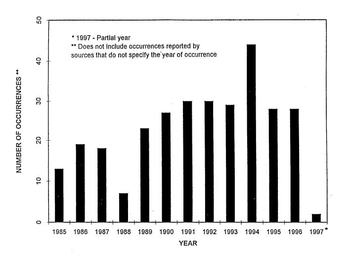
Figure 2-3 Passive Structures and Components - Degradation Occurrences Distribution By Years (1985-1997)
