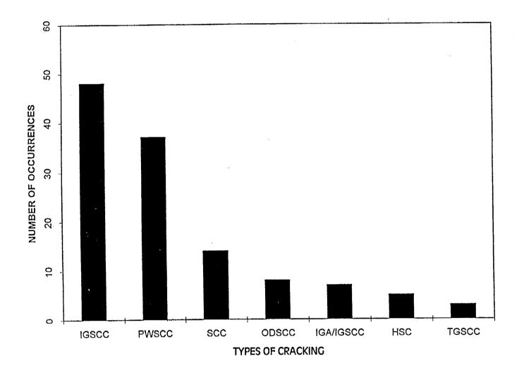
Figure 2-8 Passive Structures and Components - Degradation Occurrences Distribution By Type of Cracking Induced By Corrosion
