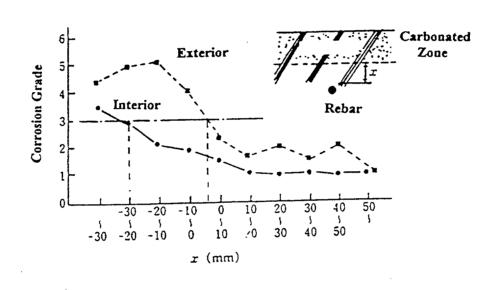
Fig. 2: Distance Between Carbonation Front from Rebar vs. Corrosion Grade (Ref.4)
