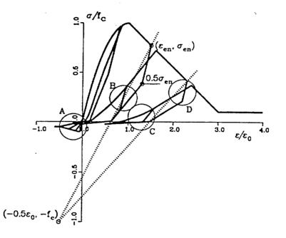
Fig. 9: Uniaxial Hysteretic Model for Concrete
