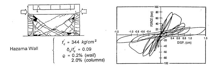
(a) Final Failure Mode
