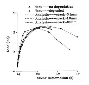
Fig. 24: Comparison of Load-Deformation Relationships by varying Crack Width
