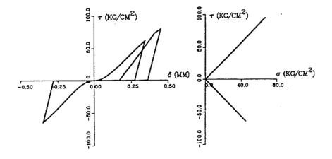
(a) Shear Stress vs. Shear
