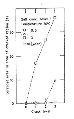
Fig. 4: Effects of Crack Width (Level 0 = no crack; 1 = micro crack; 2 = 0.03 mm crack; 3 = 0.06 mm crack) on Corrosion Progress Observed in Laboratory Tests (Ref.6)
