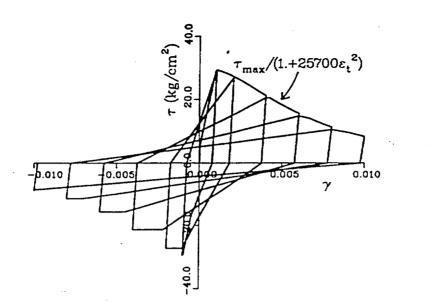
Fig. 11: Hysteretic Model for Shear Transfer Across the Cracks
