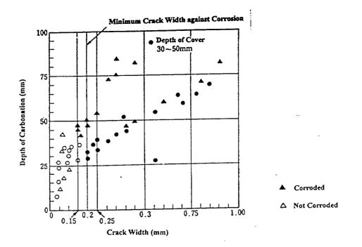
Fig. 3: Observed relationship Between Crack Width, Carbonation Depth and Corrosion of Rebars in 60 Year Old Building (Ref.5)
