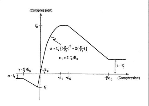
Fig. 8: Envelope Curve for Concrete
