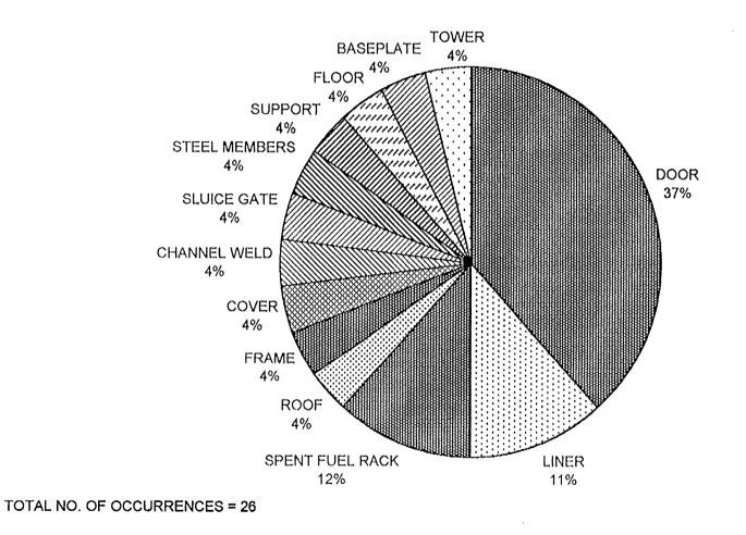
Figure 2-9 Passive Structures and Components - Degradation Occurrences Distribution of Subcomponents for Structural Steel
