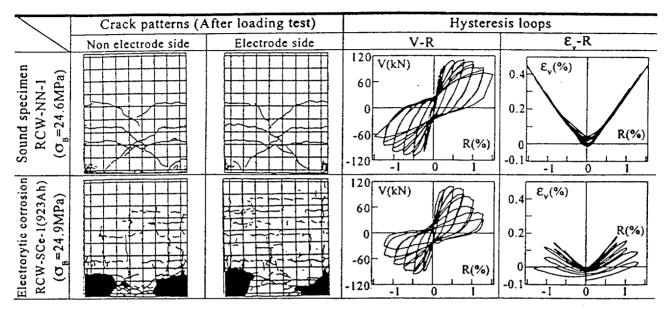
a: Shear Walls (Top - Non-Degraded; Bottom - Degraded)
