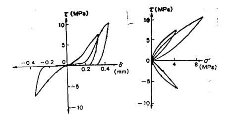
(a) Shear stress (τ) vs. ShearDeformation (δ) Relationship
