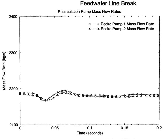
Figure 23: Recirculation Pump 1 and 2 Mass Flow Rates (0-0.2 sec)
