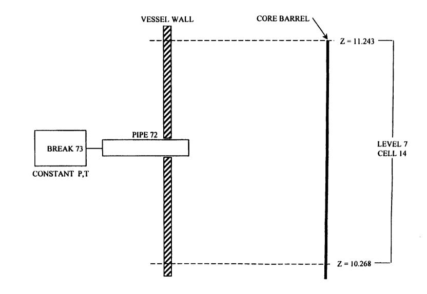
Figure 3: Break Nodalization
