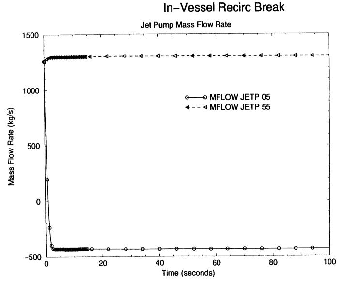
Figure 16: Mass Flow Rate in Jet Pump Components 5 and 55 (0-100 sec)
