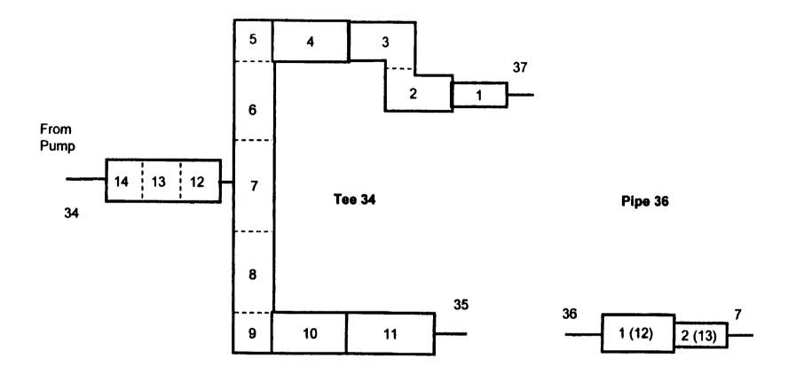
Figure 3: Renodalization of Tee Component 34
