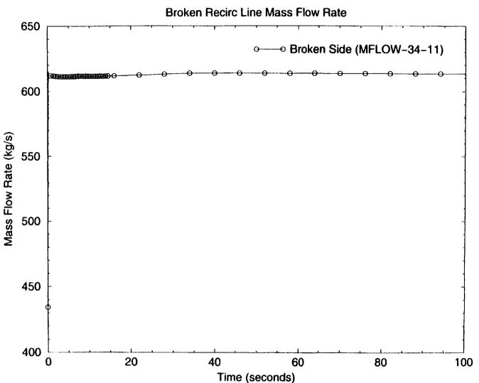
Figure 6: Mass Flow Rate in the Broken Side of the Recirculation Line (0-100 sec)
