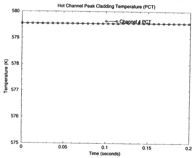
Figure 35: Peak Cladding Temperature for Hot Channel Component 4 (0-0.2 sec)
