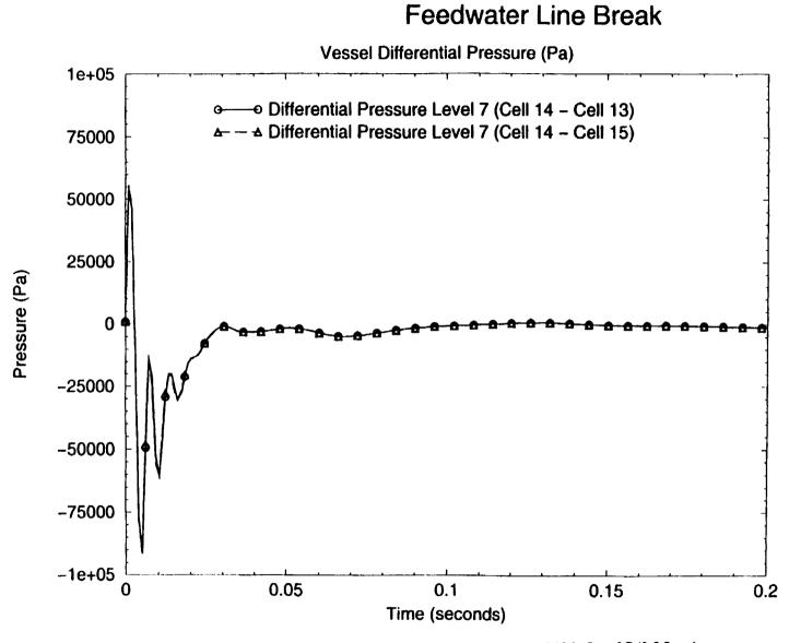
Figure 33: Differential Pressure Between Cell 14, 15 and 13 in Level 7 (0-0.2 sec)
