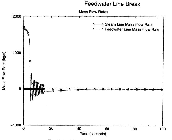
Figure 21: Steam Line and Feedwater Mass Flow Rates (0-100 sec)
