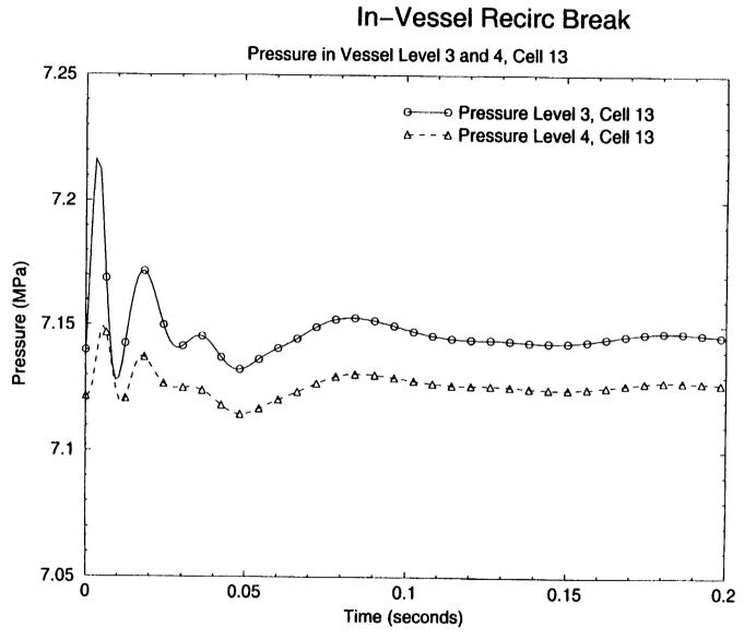
Figure 19: Pressure in Vessel Level 3, Cell 13, and Level 4 and Cell 13 (0-0.2 sec)
