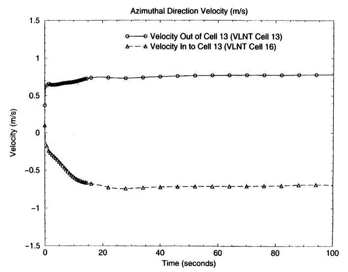
Figure 26: Azimuthal Liquid Velocities in And Out of Cell 13, Level 3 (0-100 sec)
