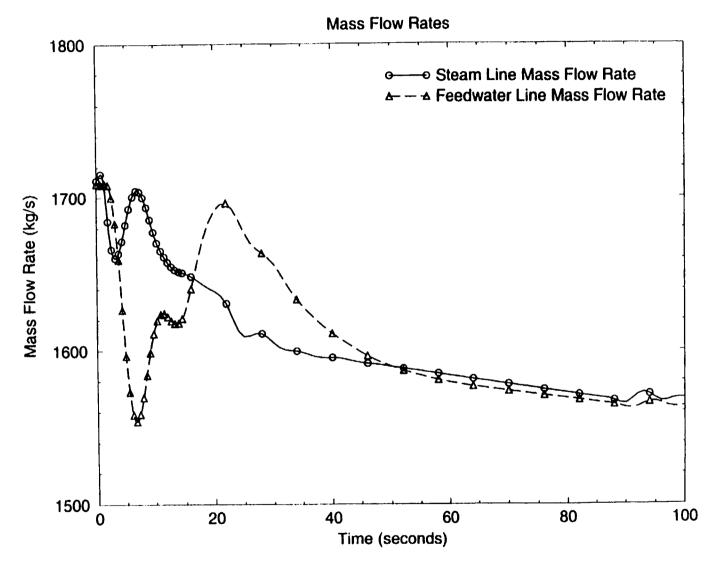
Figure 32: Steam Line and Feedwater Mass Flow Rates (0-100 sec)
