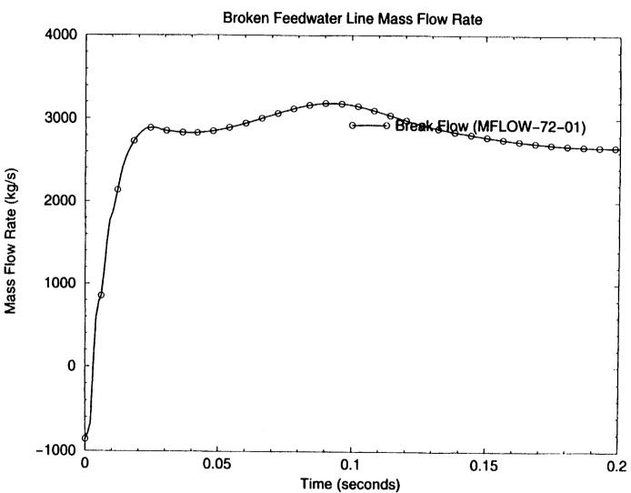
Figure 4: Mass Flow Rate in the Broken Feedwater Line (0-0.2 sec)
