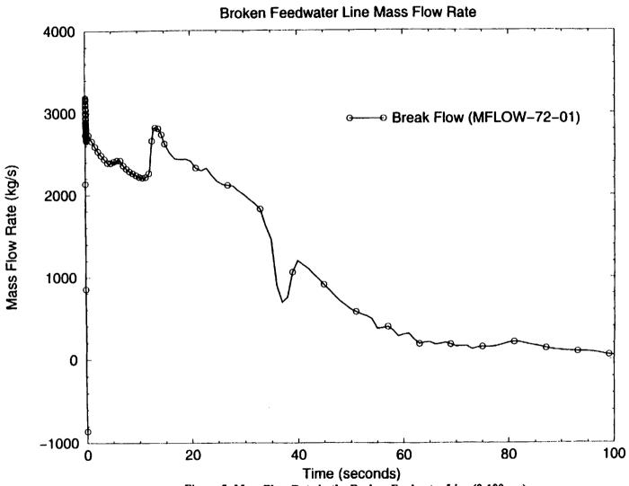
Figure 5: Mass Flow Rate in the Broken Feedwater Line (0-100 sec)
