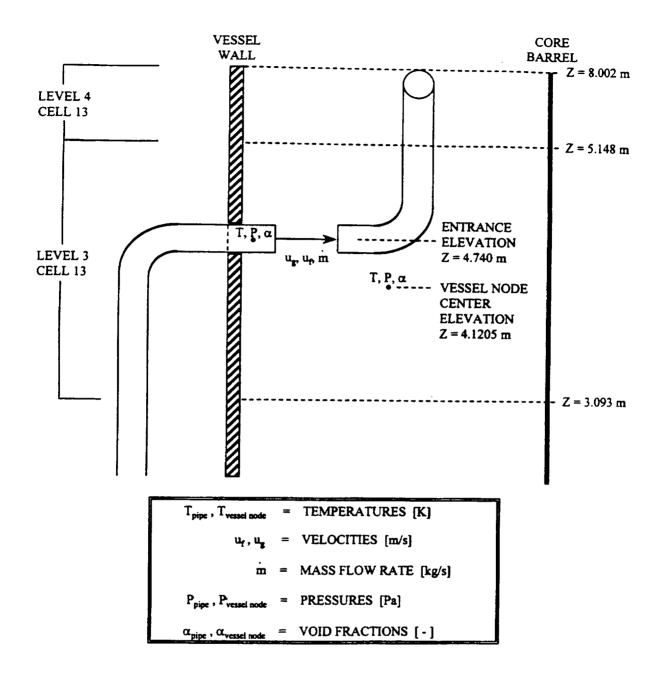
Figure 1: Simplified Break Nodalization, Side View
