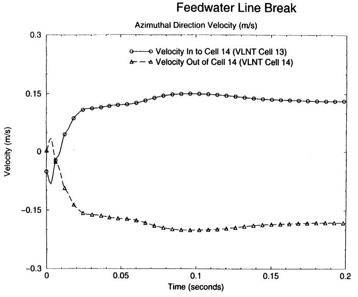
Figure 34: Azimuthal Liquid Velocities in And Out of Cell 14, Level 7 (0-0.2 sec)
