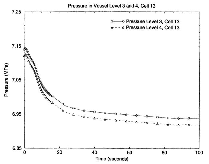
Figure 20: Pressure in Vessel Level 3, Cell 13, and Level 4 and Cell 13 (0-100 sec)
