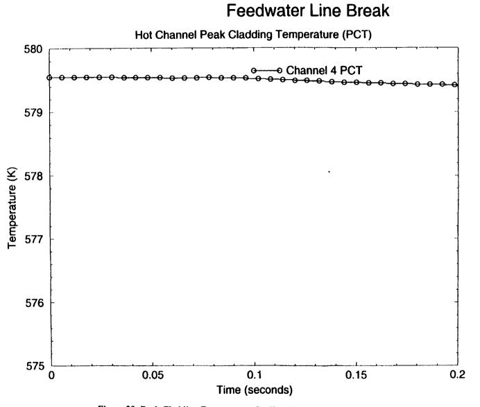
Figure 29: Peak Cladding Temperature for Hot Channel Component 4 (0-0.2 sec)
