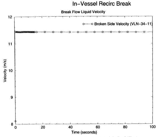
Figure 8: Liquid Velocity in the Broken Side of the Recirculation line (0-100 sec)
