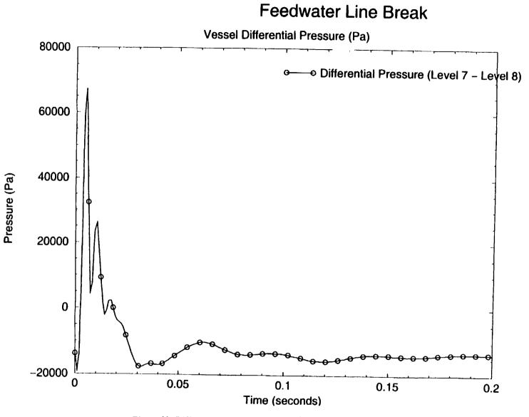
Figure 32: Differential Pressure Between Level 7 and 8 in Cell 14 (0-0.2 sec)
