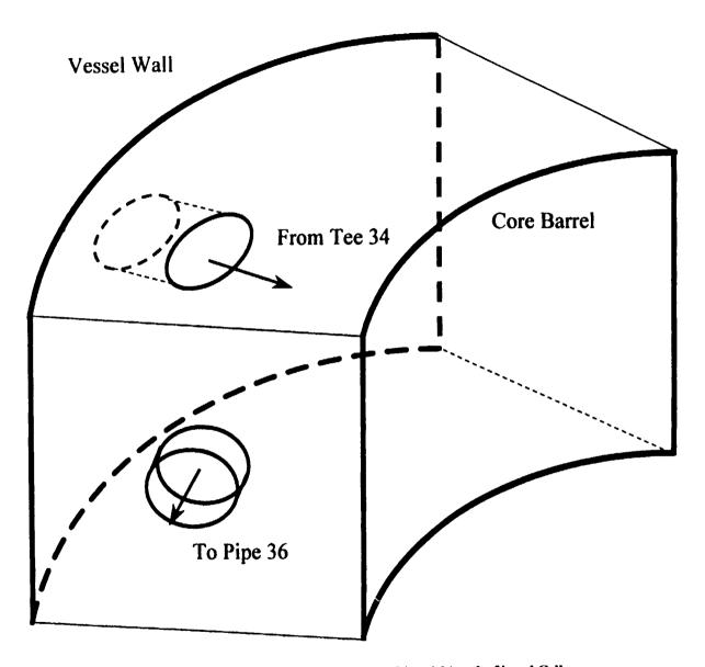
Figure 4: Connection of Components 34 and 36 to the Vessel Cell
