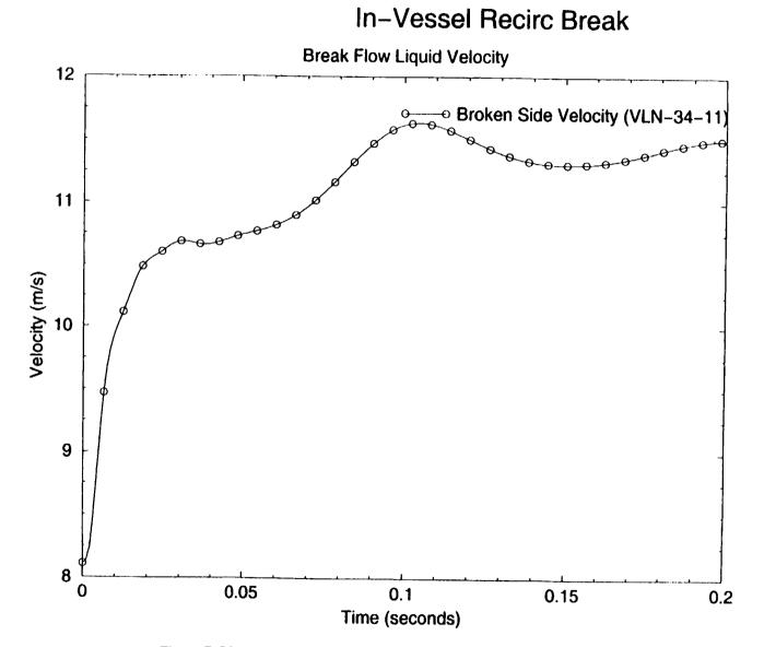
Figure 7: Liquid Velocity in the Broken Side of the Recirculation line (0-0.2 sec)
