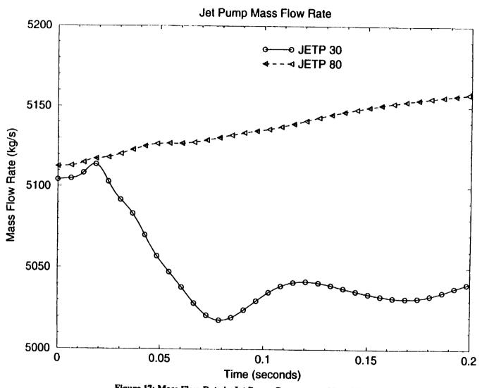
Figure 17: Mass Flow Rate in Jet Pump Components 30 and 80 (0-0.2 sec)
