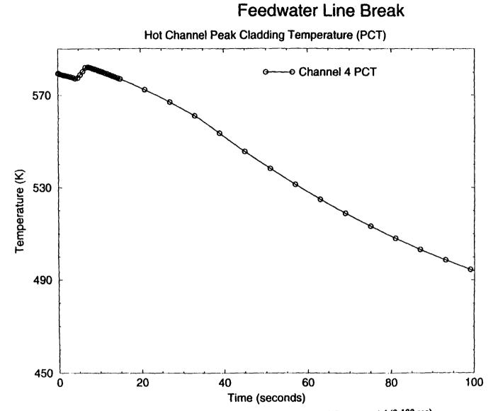
Figure 30: Peak Cladding Temperature for Hot Channel Component 4 (0-100 sec)
