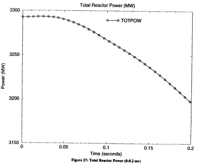
In-Vessel Recirculation Line Break
