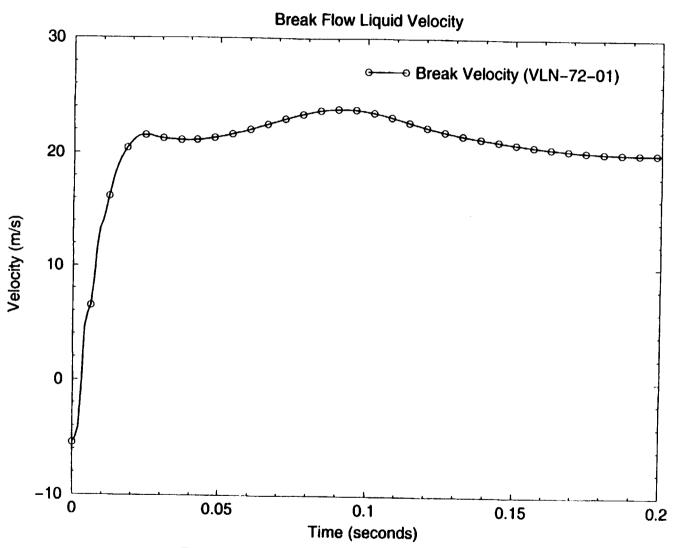
Figure 6: Liquid Velocity in the Broken Feedwater Line (0-0.2 sec)
