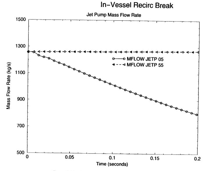
Figure 15: Mass Flow Rate in Jet Pump Components 5 and 55 (0-0.2 sec)
