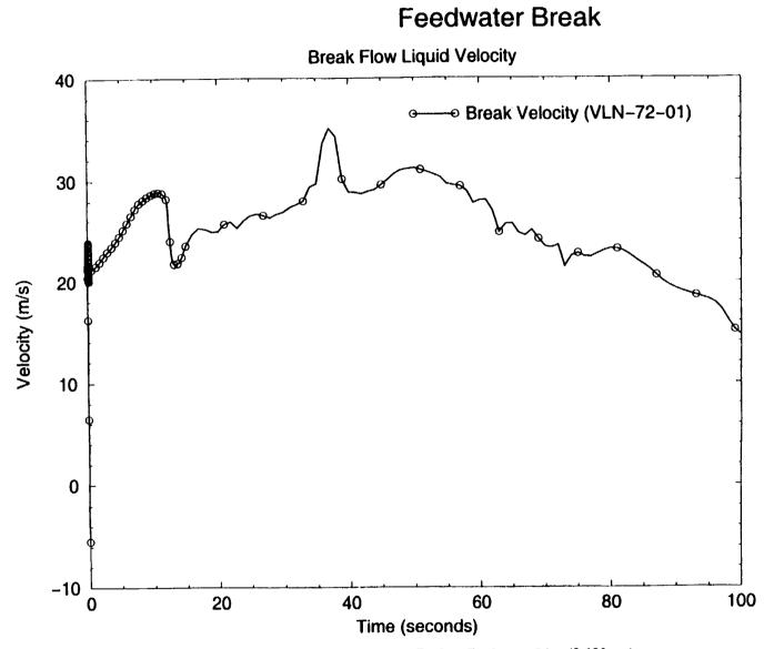
Figure 7: Liquid Velocity in the Broken Feedwater Line (0-100 sec)
