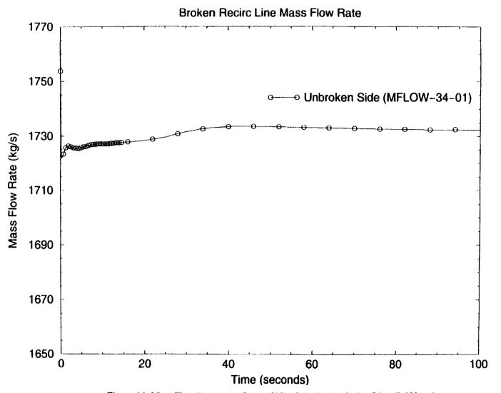
Figure 14: Mass Flow Rate in the Intact Side of the Recirculation Line (0-100 sec)
