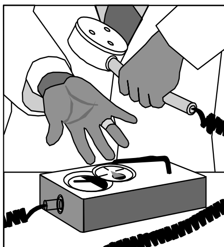
Surveying arm and hand using survey meter and beta/gamma probe.
