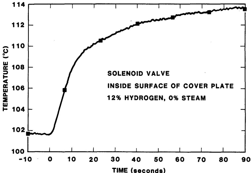
Figure 19. Typical Temperature Response of Solenoid Valve
