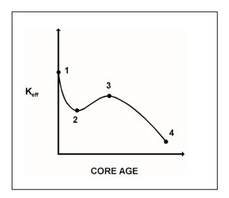
Refer to the curve of K<sub>eff</sub> versus core age for an operating reactor (see figure below).
