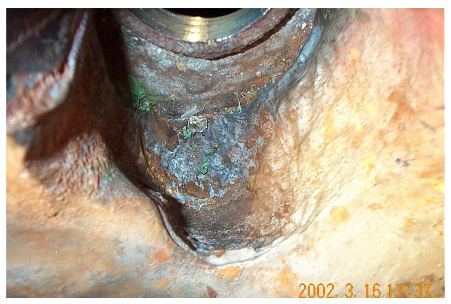
Nozzle 3 with insulation removed and shielding installed 03-16-02
