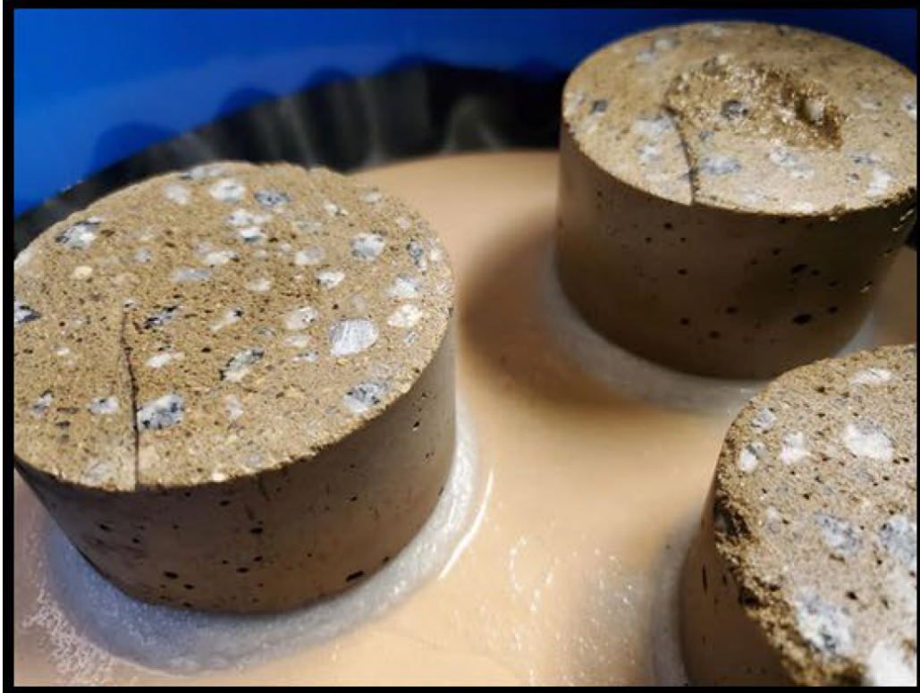
Figure 10. Zero-bleed, Structural Flowable Fill with No. 8 Stone (ZB-FF-8-D) Grout Samples. Image Credit: SREL Doc-R-21-0003, Figure 8.
