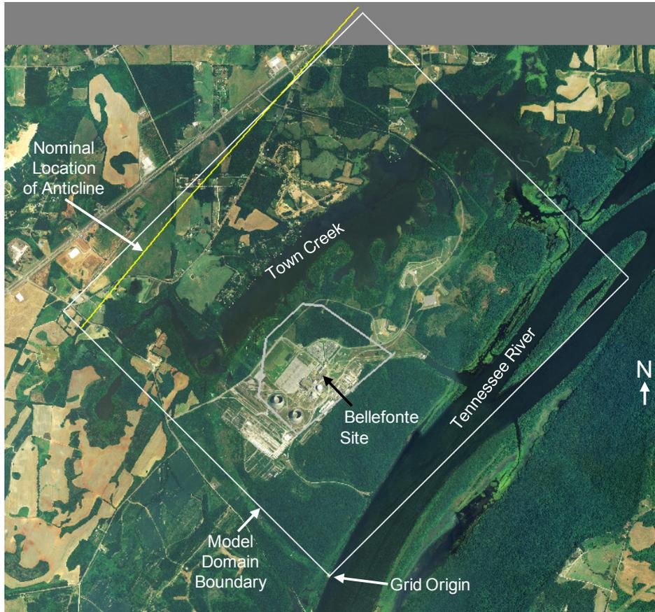
**Figure 22. Extent of the groundwater simulation model grid relative to key features. The grid origin is located in the lower left corner of the model at the bottom of the domain.**
