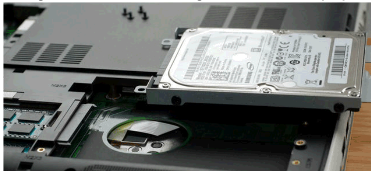
Figure 2. A hard drive being removed from a laptop.
