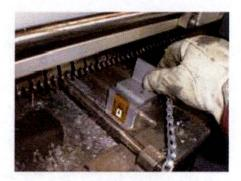
With a gloved hand install the solder level fixture as shown on either front side of the solder pot.
