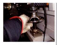
While wearing the smock & gloves, use the wheel to the right of the solder pot. Adjust the conveyor as shown in the next picture.
