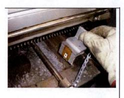
With a gloved hand remove the solder level fixture from the solder pot.
