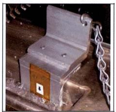
Verify the solder level at a minimum is at the bottom of the solder level fixture. If not, add solder to the pot accordingly.
