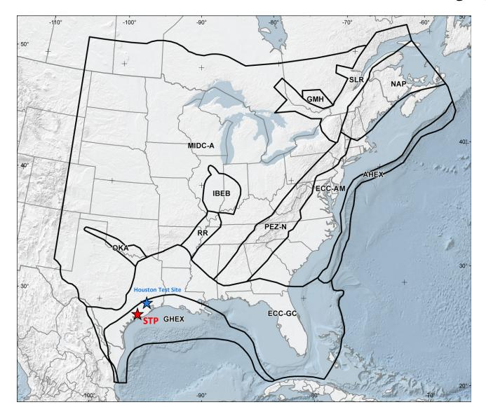
Seismotectonic zones are based on historical seismicity and regional-scale geologic and tectonic data to characterize seismic sources zones at a finer scale than the Mmax zones model.
