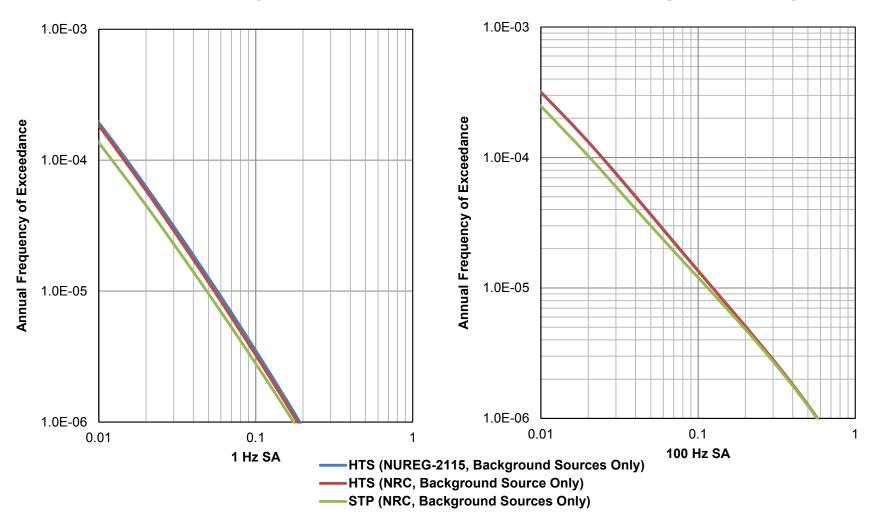
Staff concluded that the COL applicant's use of NUREG-2115 hazard curves for the Houston Test Site for 1 Hz, 10 Hz, and 100 Hz, an adequate substitute for performing hazard calculations at the STP site using the CEUS-SSC model.
