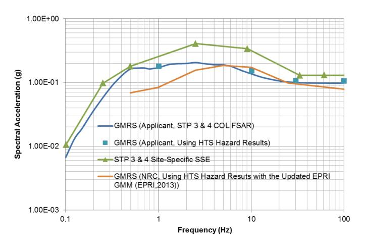
The applicant's CEUS-SSC GMRS and the staff's confirmatory CEUS-SSC GMRS, which are based on the use of CEUS-SSC model for the Houston Test Site, are well below the STP 3 & 4 Site-Specific SSE
