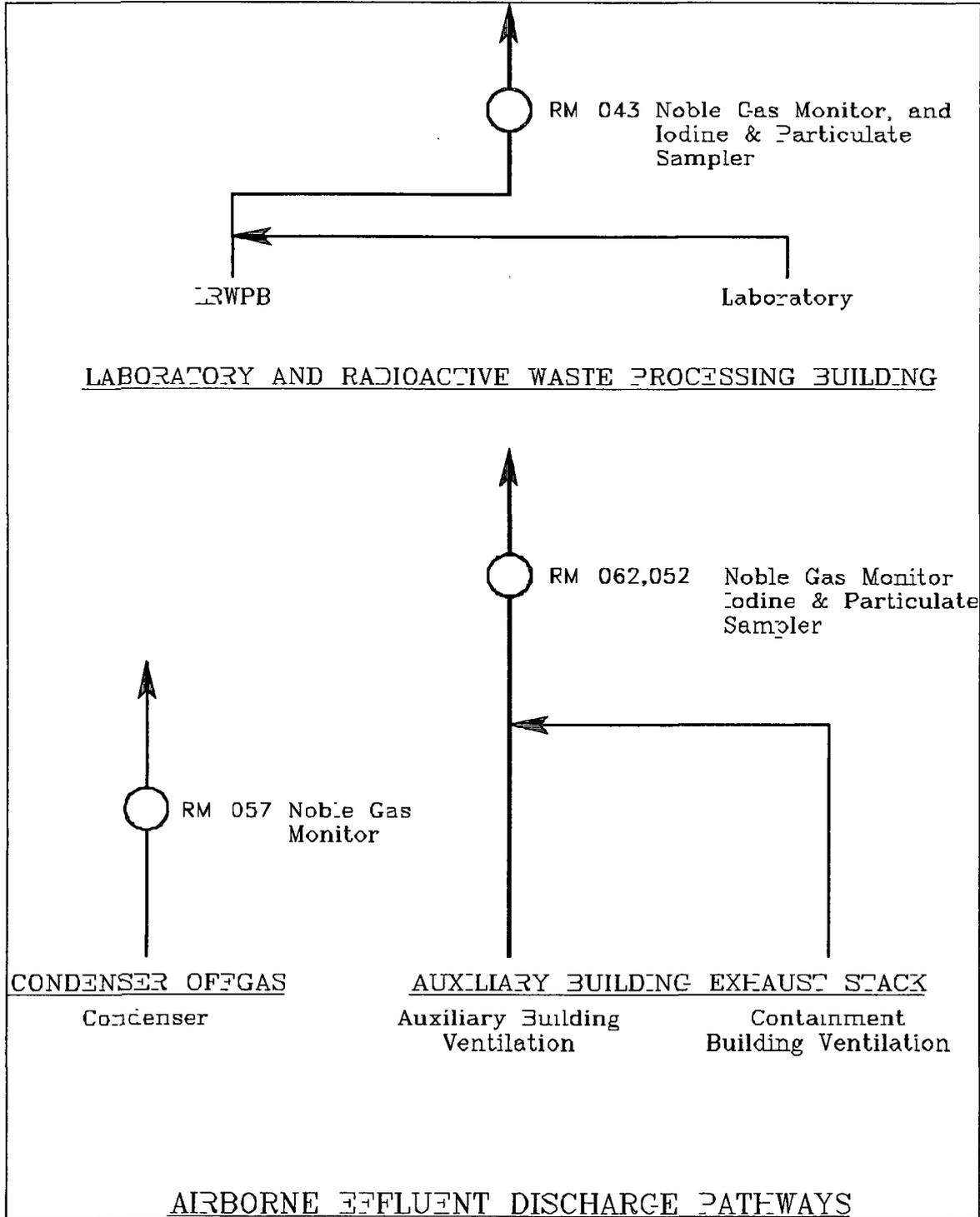
Figure 5 - Airborne Radioactive Waste Disposal System
