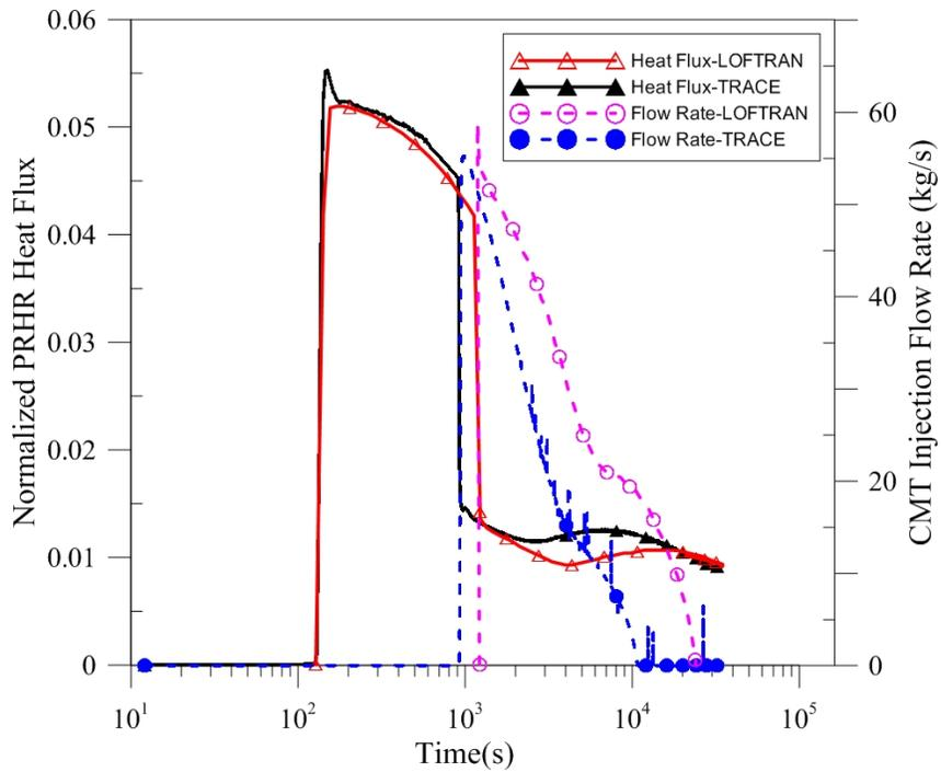
**Figure 5 Normalized PRHR heat flux and CMT injection flow rate (loss of normal feedwater flow)**
