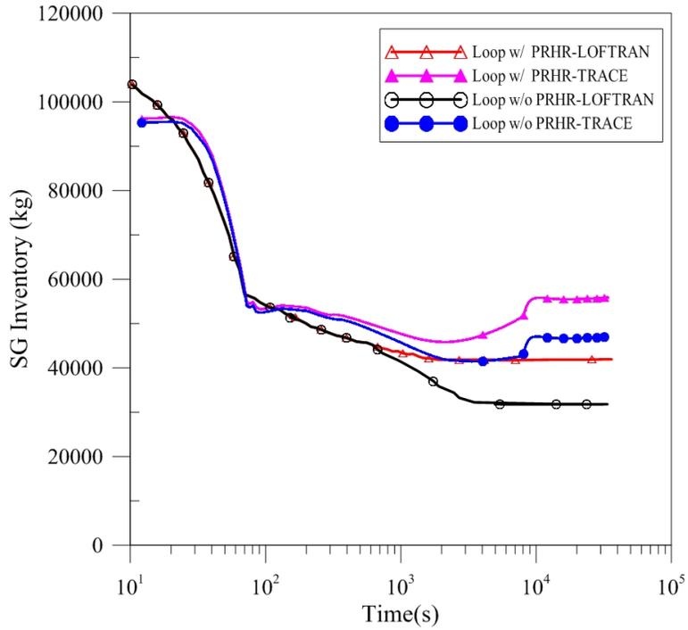
Figure 10 SG inventory (loss of AC power to the plant auxiliaries)
