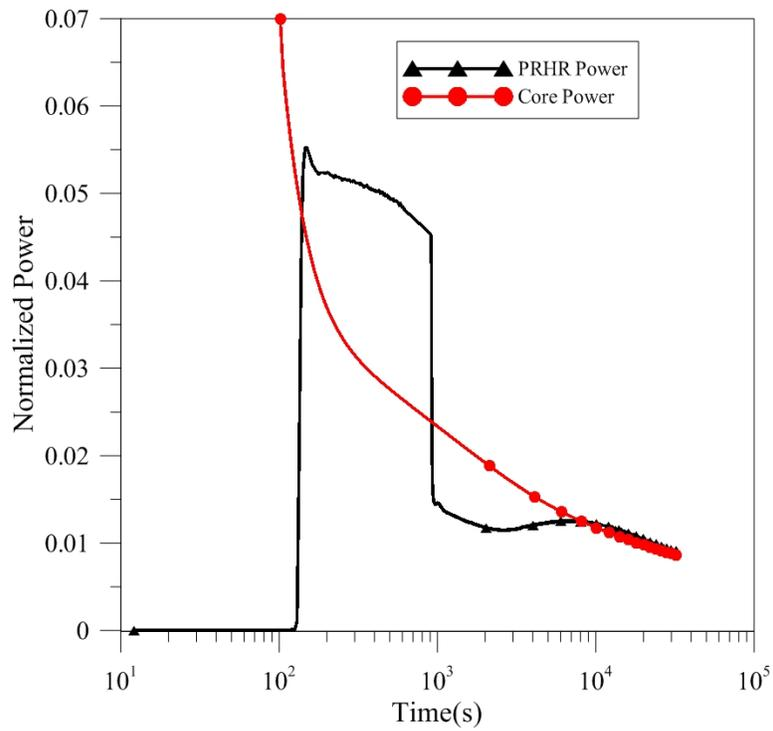
**Figure 7 Normalized PRHR and core power (loss of normal feedwater flow)**
