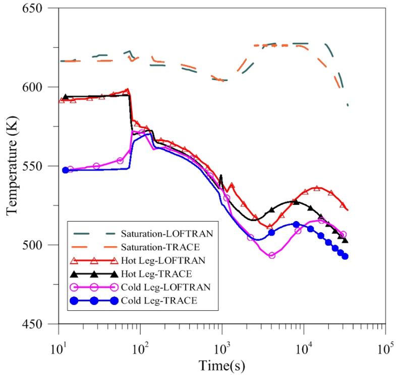
**Figure 6 RCS temperature in loop containing the PRHR (loss of normal feedwater flow)**
