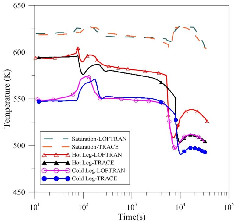
Figure 11 RCS temperature in loop containing the PRHR (loss of AC power to the plant auxiliaries)
