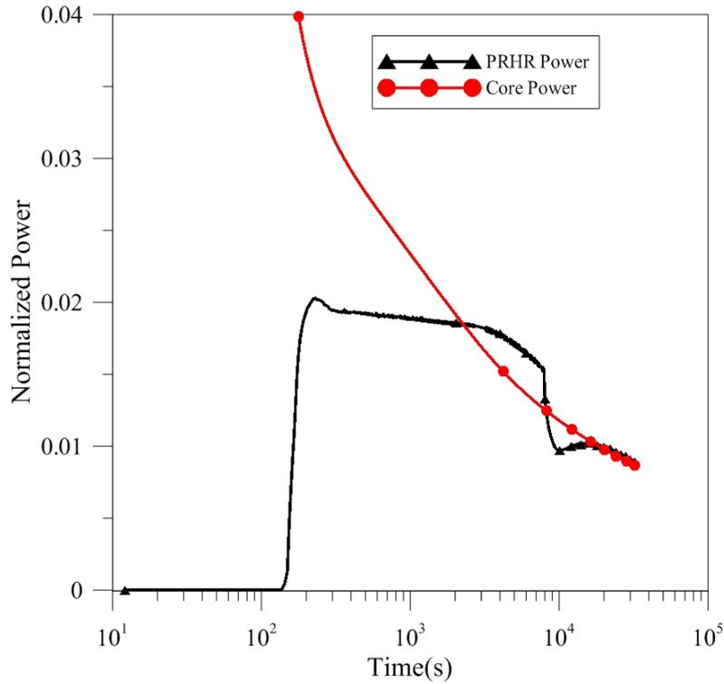
Figure 12 Normalized PRHR and core power (loss of AC power to the plant auxiliaries)
