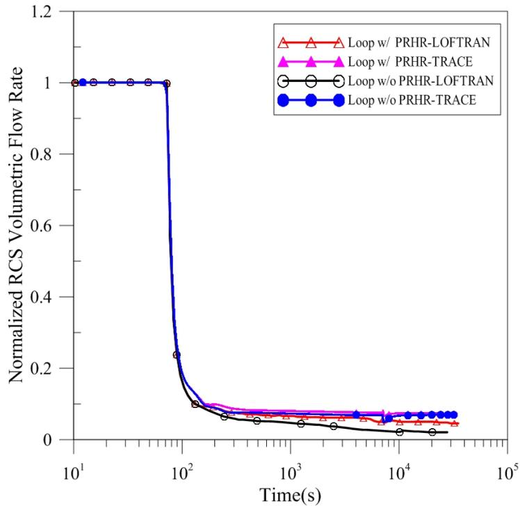
**Figure 8 Normalized RCS volumetric flow rate (loss of AC power to the plant auxiliaries)**
