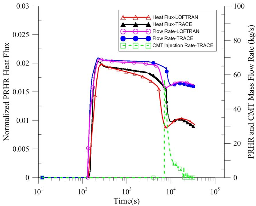
**Figure 9 Normalized PRHR heat flux and mass flow rate of PRHR and CMT injection (loss of AC power to the plant auxiliaries)**
