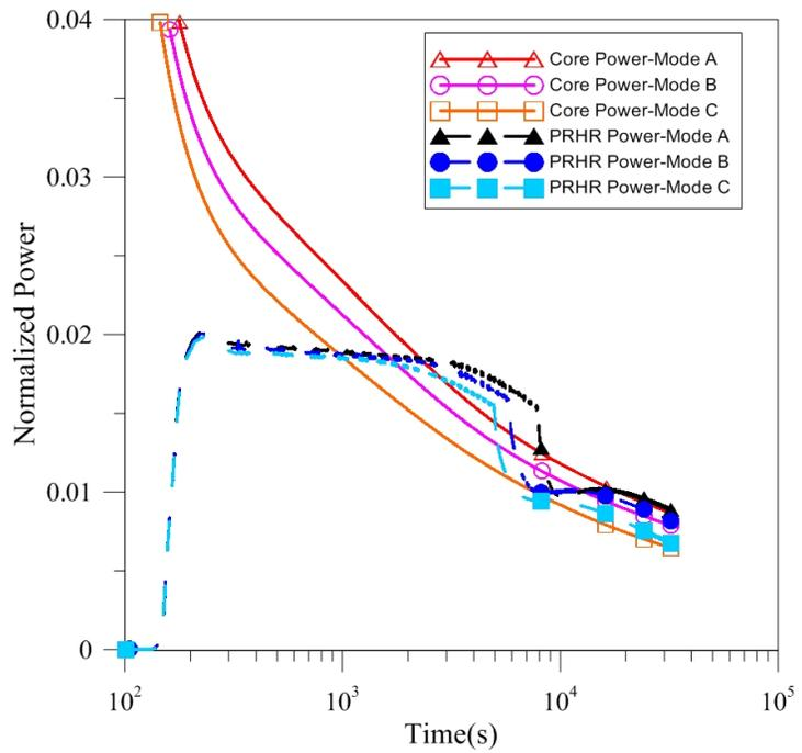
Figure 13 Sensitivity study on different decay heat generation (loss of AC power to the plant auxiliaries)
