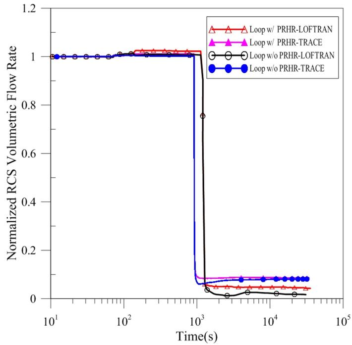
**Figure 4 Normalized RCS volumetric flow rate (loss of normal feedwater flow)**
