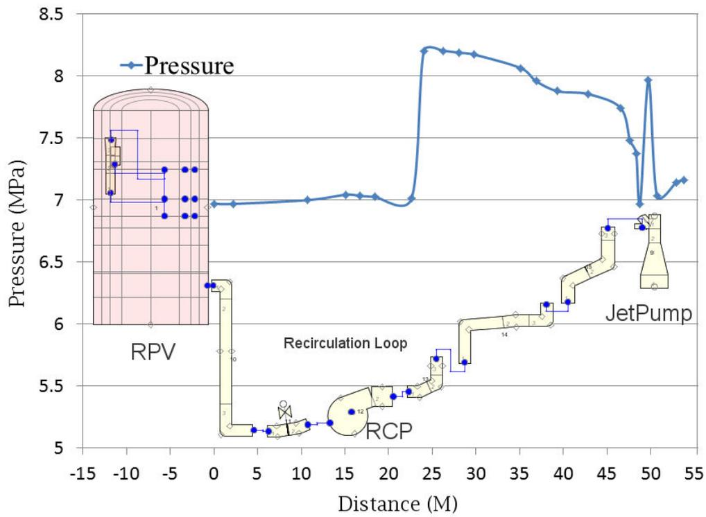
**Figure 2 Pressure distributions in recirculation loop**
