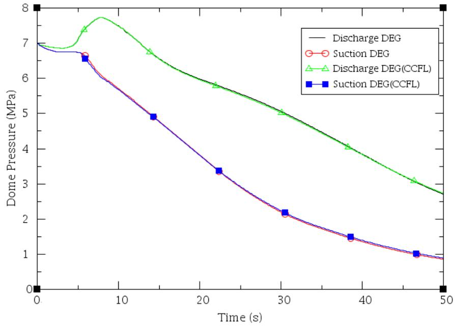
**Figure 4 Comparison of reactor pressure**
