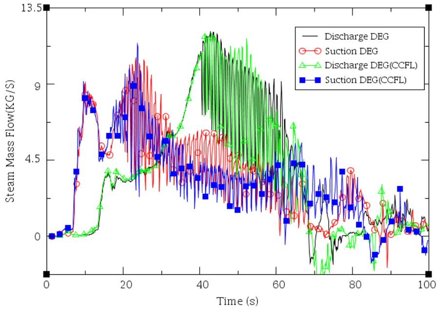
**Figure 11 Comparison of the steam flow in lower plenum**
