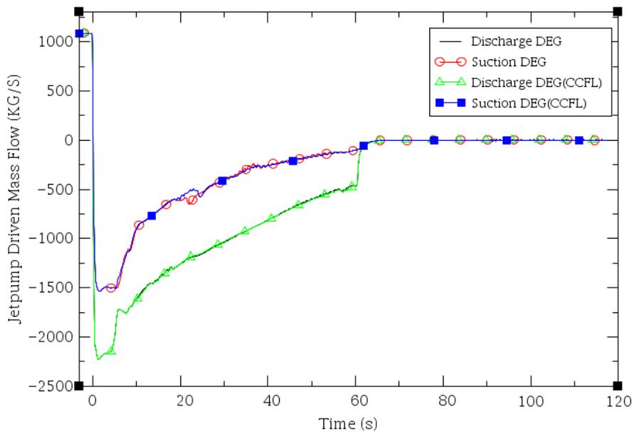
**Figure 10 Comparison of driven flow rate of jet pumps at the broken loop**
