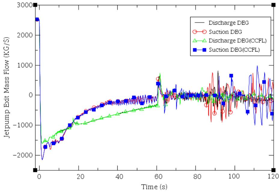
**Figure 7 Comparison of the jet pumps exit flow rate at the broken loop**
