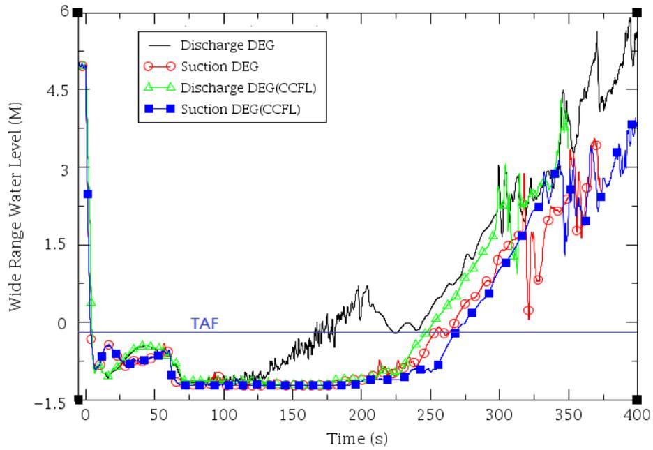
**Figure 9 Comparison of the reactor water level**
