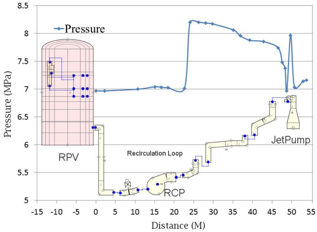
**Figure 2 Pressure distributions in recirculation loop**
