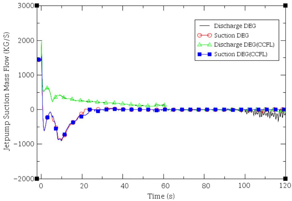
**Figure 8 Comparison of the jet pumps suction flow rate at the broken loop**
