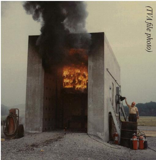
*Picture of TVA Browns Ferry seal penetration tests*
