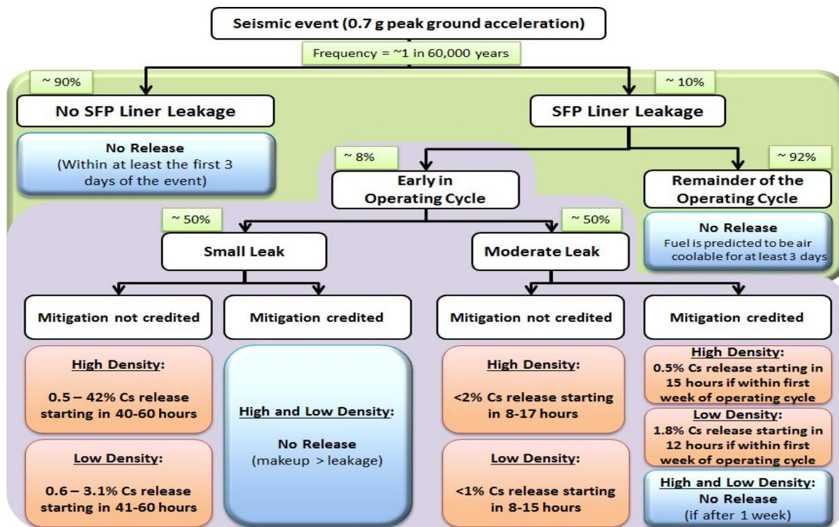
Note: The low-density pool has about 1/3 of Cs-137 inventory compared to high-density pool. Early in the operating cycle refers to early time after shutdown.
