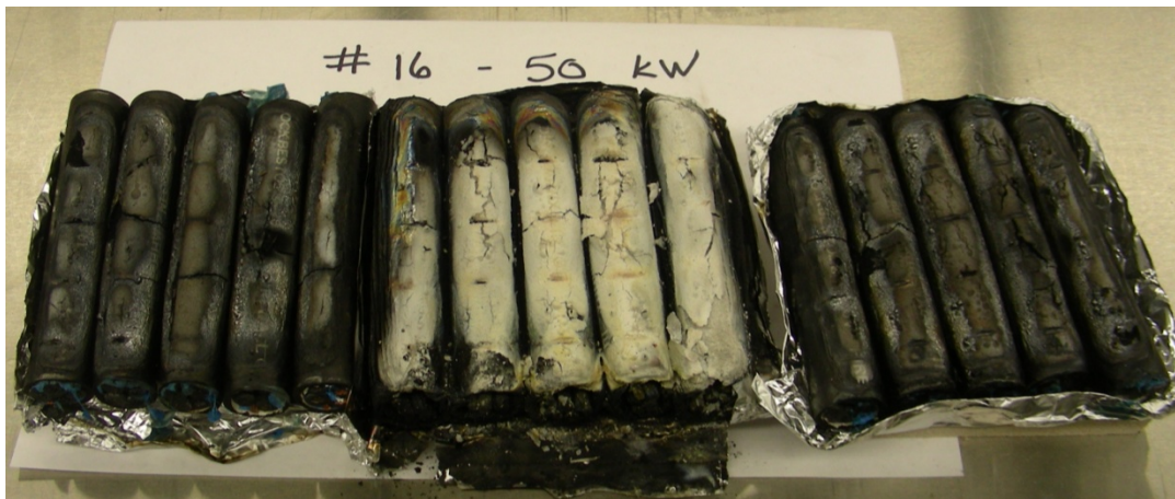
Figure 6-12. Photograph of Cable #16 after Cone Calorimeter test at 50 kW/m 2 .
