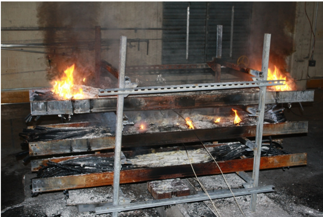
Figure 8-17. Fire spread to the ends of Tray 3, Multiple Tray Test 15.
