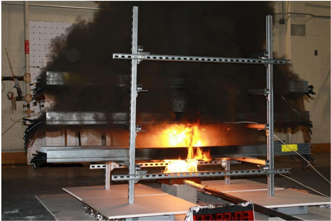
Figure 8-1. Multiple Tray (MT) cable test apparatus.
