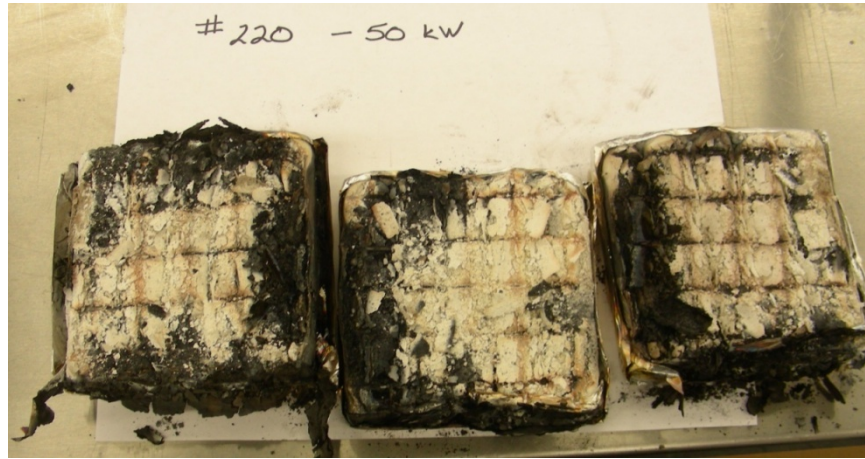
Figure 6-27. Photograph of Cable #220 after Cone Calorimeter test at 50 kW/m 2 .
