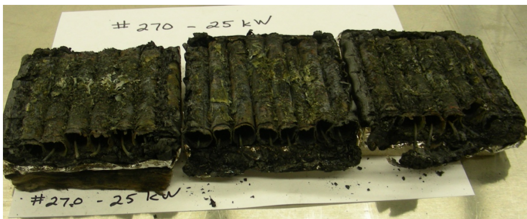
Figure 6-29. Photograph of Cable #270 after Cone Calorimeter test at 25 kW/m 2 .
