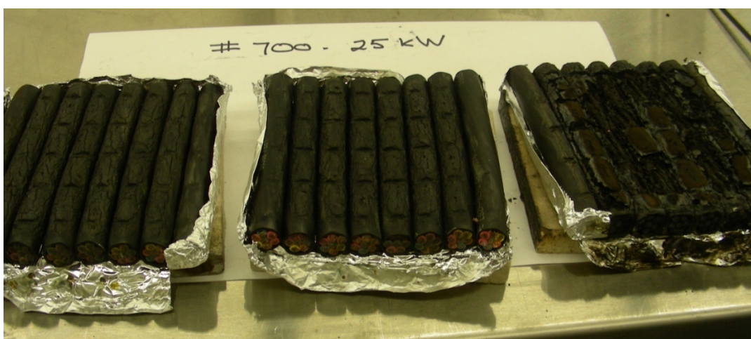
Figure 6-38. Photograph of Cable #700 after Cone Calorimeter test at 25 kW/m 2 .
