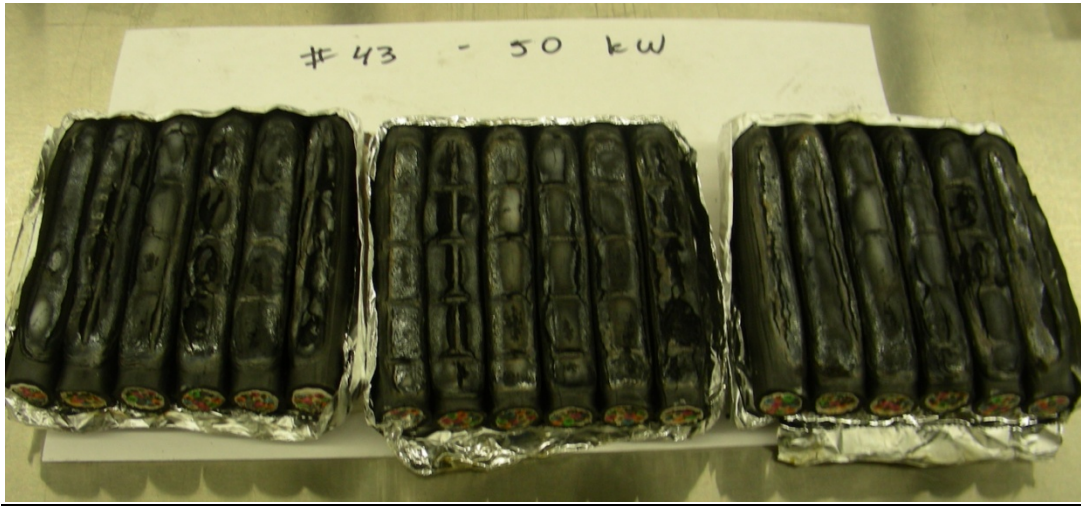
Figure 6-18. Photograph of Cable #43 after Cone Calorimeter test at 50 kW/m 2 .
