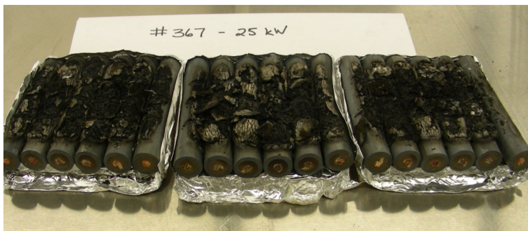
Figure 6-35. Photograph of Cable #367 after Cone Calorimeter test at 25 kW/m 2 .
