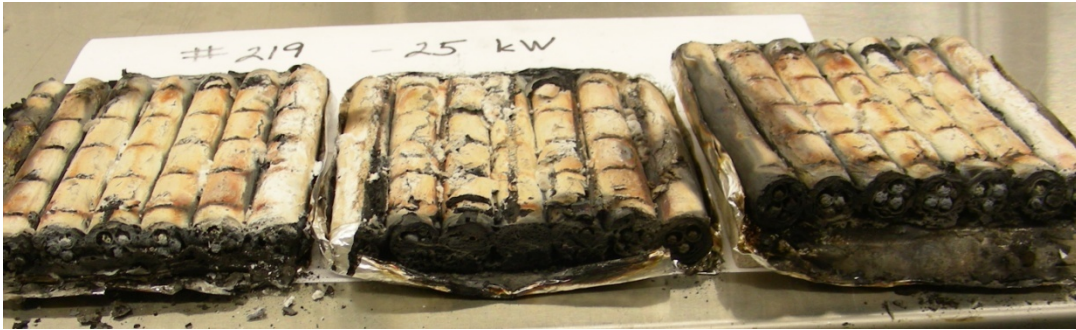
Figure 6-23. Photograph of Cable #219 after Cone Calorimeter test at 25 kW/m 2 .
