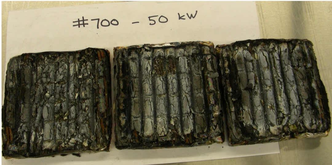
Figure 6-39. Photograph of Cable #700 after Cone Calorimeter test at 50 kW/m 2 .
