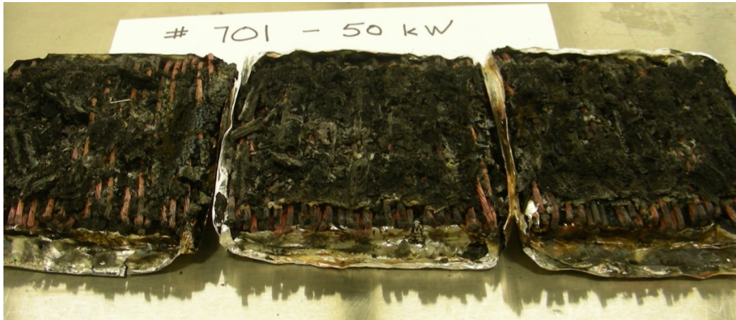
Figure 6-42. Photograph of Cable #701 after Cone Calorimeter test at 50 kW/m 2 .
