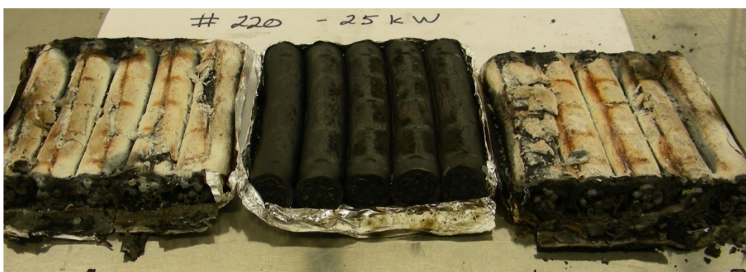
Figure 6-26. Photograph of Cable #220 after Cone Calorimeter test at 25 kW/m 2 .
