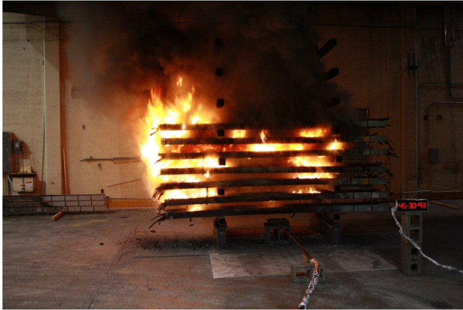
Figure 8-31. Photograph of Multiple Tray Test MT-23.
