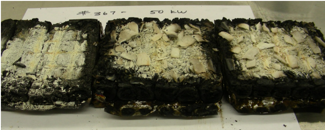
Figure 6-36. Photograph of Cable #367 after Cone Calorimeter test at 50 kW/m 2 .
