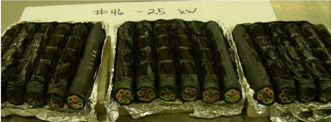
Figure 6-20. Photograph of Cable #46 after Cone Calorimeter test at 25 kW/m 2 .
