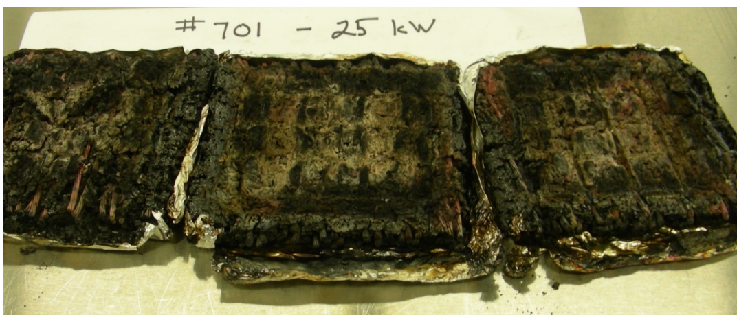
Figure 6-41. Photograph of Cable #701 after Cone Calorimeter test at 25 kW/m 2 .
