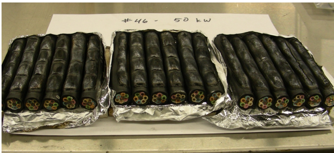
Figure 6-21. Photograph of Cable #46 after Cone Calorimeter test at 50 kW/m 2 .
