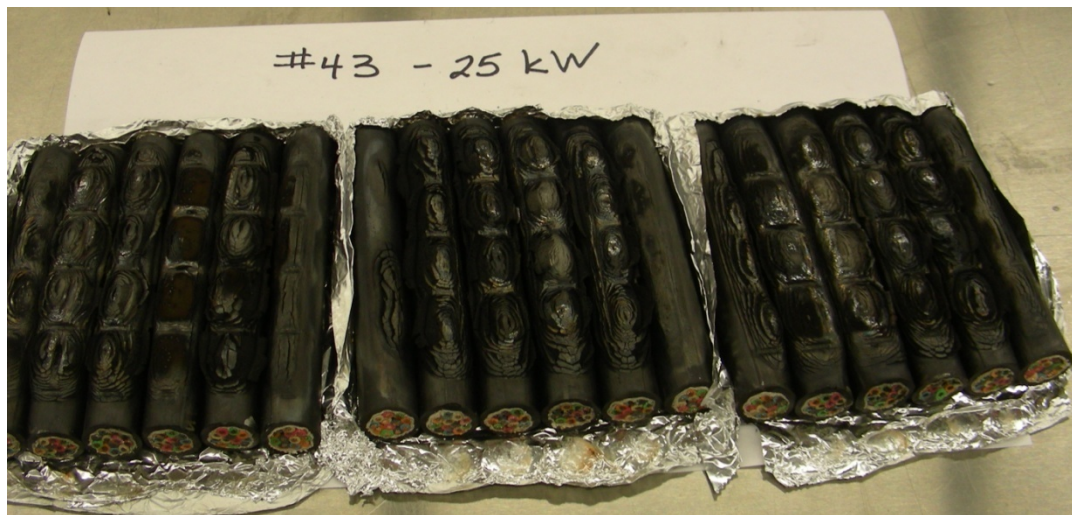
Figure 6-17. Photograph of Cable #43 after Cone Calorimeter test at 25 kW/m 2 .
