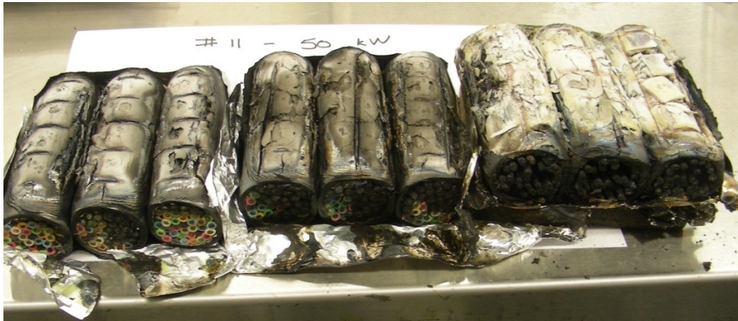
Figure 6-9. Photograph of Cable #11 after Cone Calorimeter test at 50 kW/m 2 .
