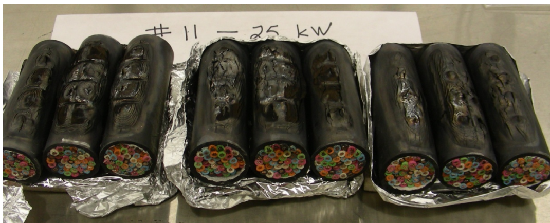
Figure 6-8. Photograph of Cable #11 after Cone Calorimeter test at 25 kW/m 2 .
