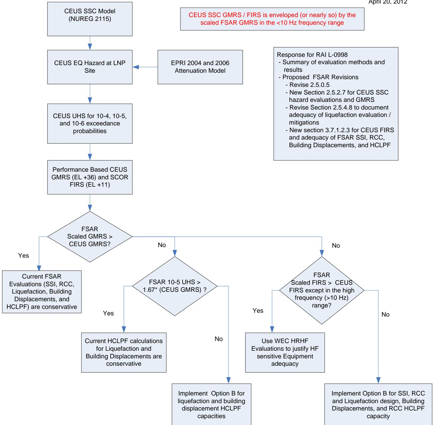
CEUS SSC GMRS / FIRS is enveloped (or nearly so) by the scaled FSAR GMRS in the <10 Hz frequency range
