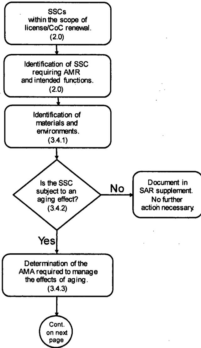
**Figure 3-1 Flowchart of AMR Process**
