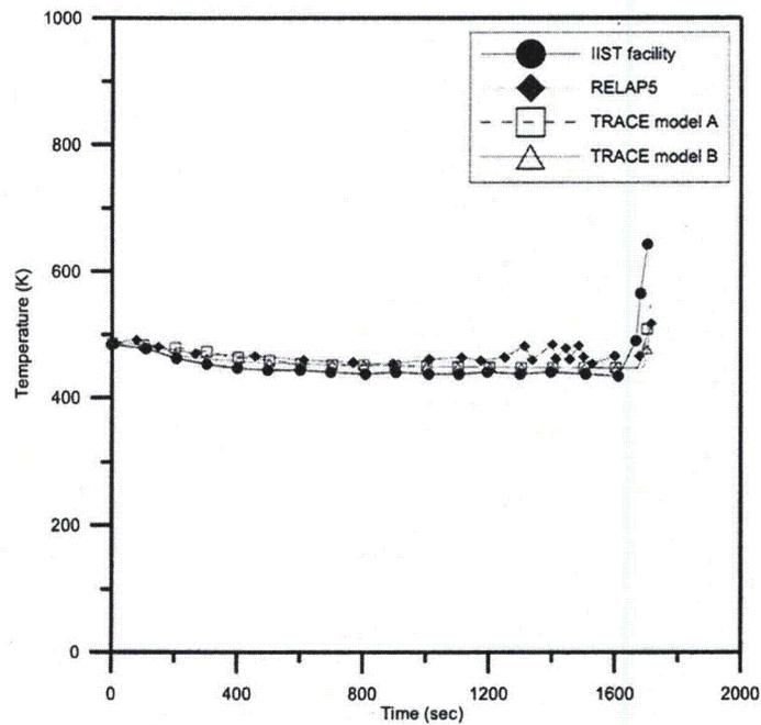
**Fig. 4.14 The comparison of Core cladding temperature among IIST facility, RELAP5, TRACE in the SBLOCA experiment**
