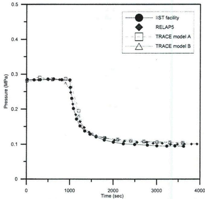
Fig. 4.16 The comparison of SG1 secondary side pressure among IIST facility, RELAP5, TRACE in the C61128 experiment
