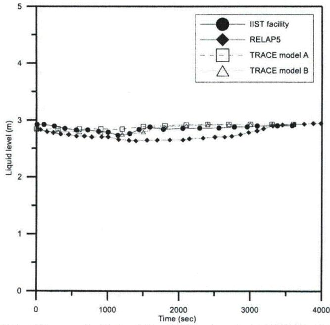
**Fig. 4.26 The comparison of core collapsed liquid level among IIST facility, RELAP5, TRACE in the C61210 experiment**
