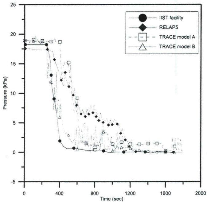
**Fig. 4.6 The comparison of SG2-outlet tube top differential pressure among IIST facility, RELAP5, TRACE in the SBLOCA experiment**
