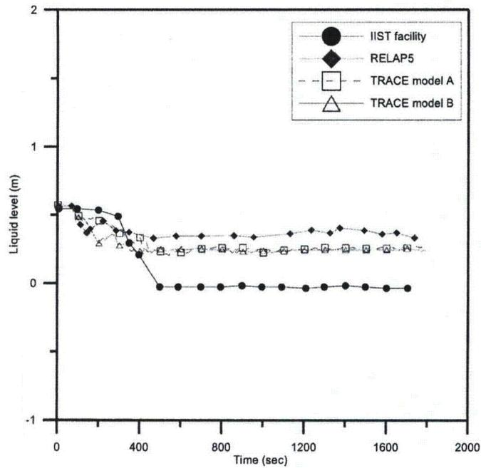
**Fig. 4.7 The comparison of SG1-inlet plenum liquid level among IIST facility, RELAP5, TRACE in the SBLOCA experiment**
