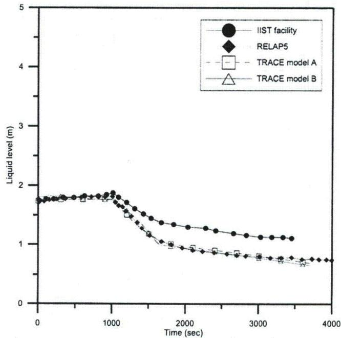
**Fig. 4.32 The comparison of pressurizer collapsed liquid level among IIST facility, RELAP5, TRACE in the C70122 experiment**
