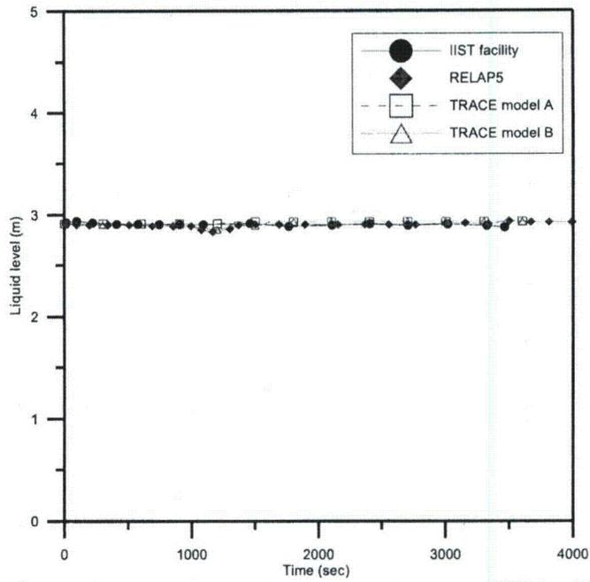
**Fig. 4.33 The comparison of core collapsed liquid level among IIST facility, RELAP5, TRACE in the C70122 experiment**
