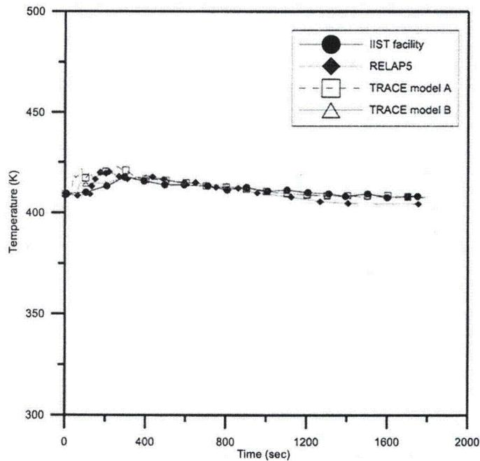
**Fig. 4.12** The comparison of loop 3 cold-leg temperature among IIST facility, RELAP5, TRACE in the SBLOCA experiment
