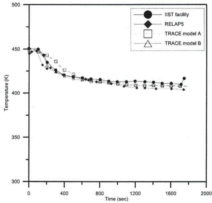
**Fig. 4.11** The comparison of loop 3 hot-leg temperature among IIST facility, RELAP5, TRACE in the SBLOCA experiment
