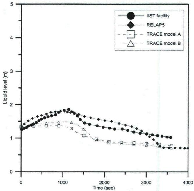
Fig. 4.25 The comparison of pressurizer collapsed liquid level among IIST facility, RELAP5, TRACE in the C61210 experiment
