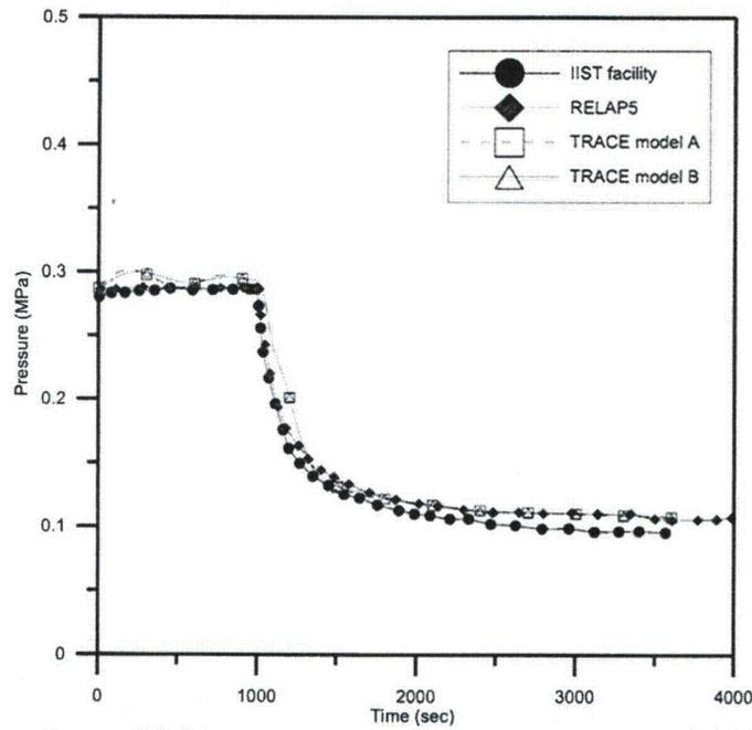
**Fig. 4.23 The comparison of SG1 secondary side pressure among IIST facility, RELAP5, TRACE in the C61210 experiment**
