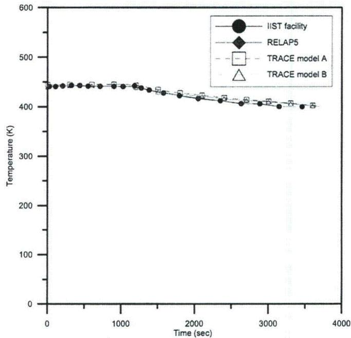
**Fig. 4.20 The comparison of loop 1 hot-leg temperature among IIST facility, RELAP5, TRACE in the C61128 experiment**
