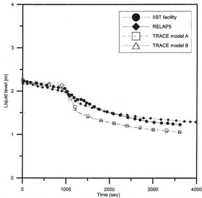
**Fig. 4.17** The comparison of SG1 collapsed liquid level among IIST facility, RELAP5, TRACE in the C61128 experiment
