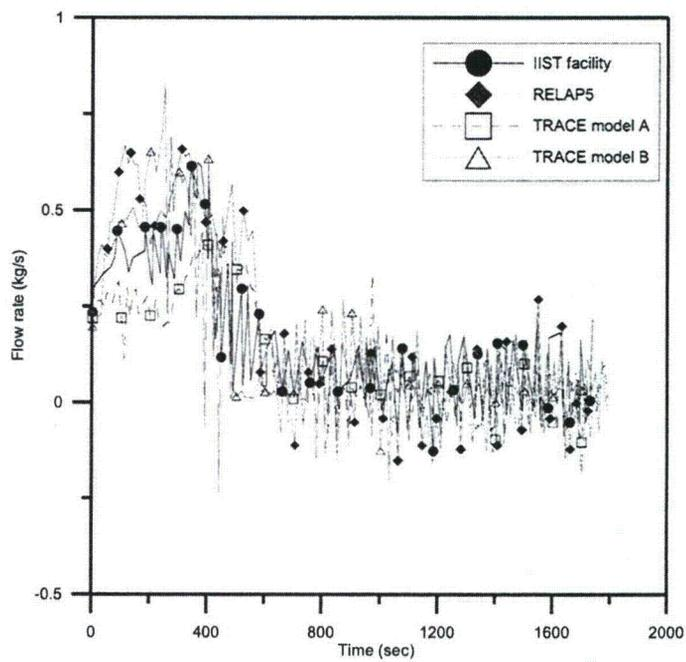
**Fig. 4.4 The comparison of loop 3 flow rate among IIST facility, RELAP5, TRACE in the SBLOCA experiment**
