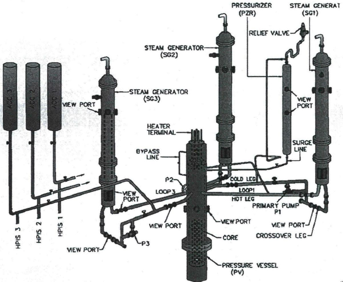
Fig. 2.1 The schema of the IIST facility<sup>(7)</sup>
