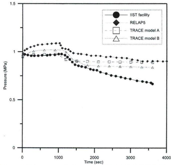
**Fig. 4.22 The comparison of Primary system pressure among IIST facility, RELAP5, TRACE in the C61210 experiment**
