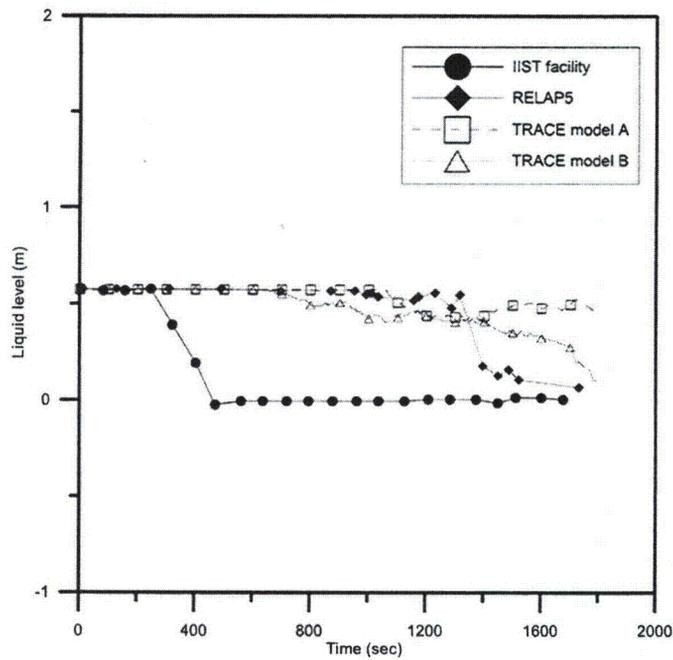
**Fig. 4.8 The comparison of SG1-outlet plenum liquid level among IIST facility, RELAP5, TRACE in the SBLOCA experiment**
