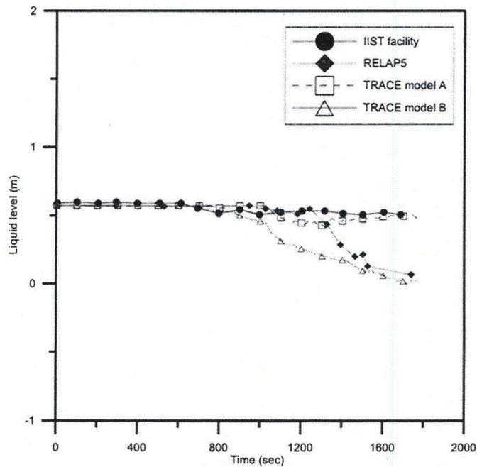
**Fig. 4.10 The comparison of SG3-outlet plenum liquid level among IIST facility, RELAP5, TRACE in the SBLOCA experiment**
