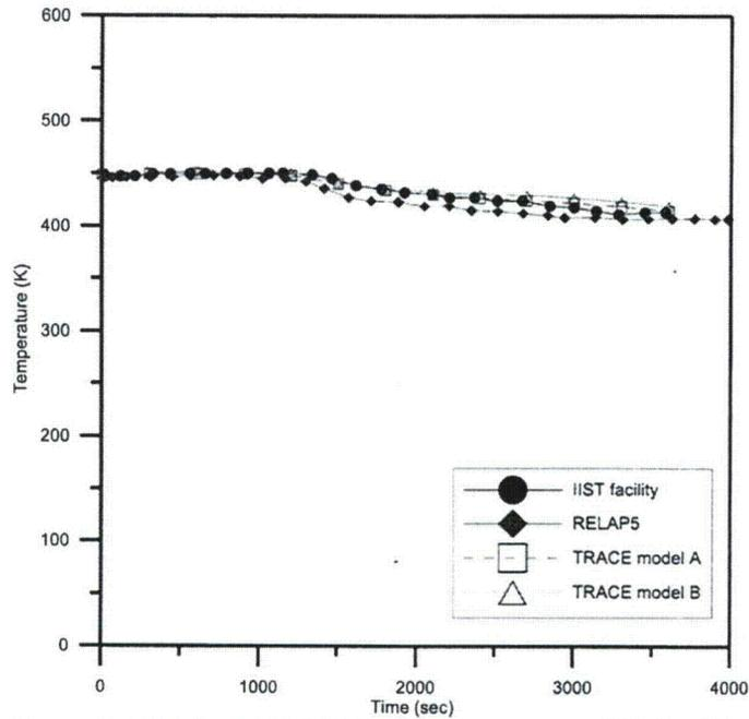
**Fig. 4.27 The comparison of loop 1 hot-leg temperature among IIST facility, RELAP5, TRACE in the C61210 experiment**
