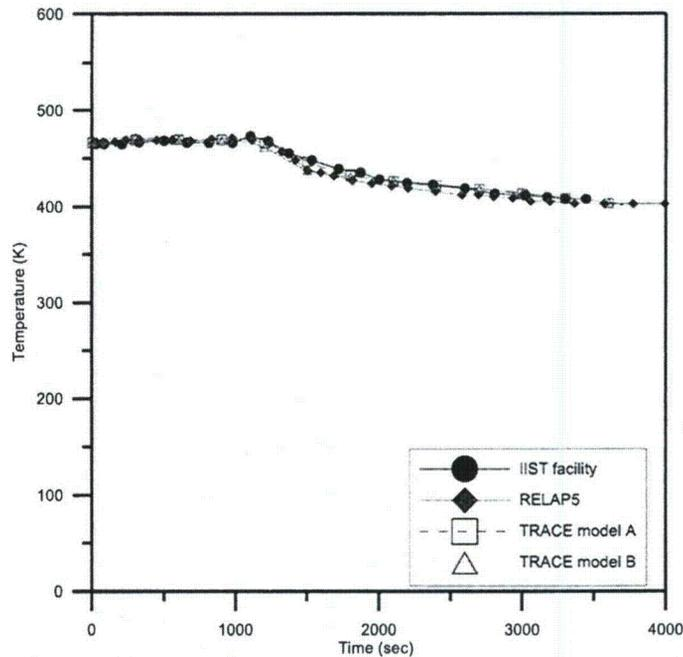
**Fig. 4.34 The comparison of loop 1 hot-leg temperature among IIST facility, RELAP5, TRACE in the C70122 experiment**
