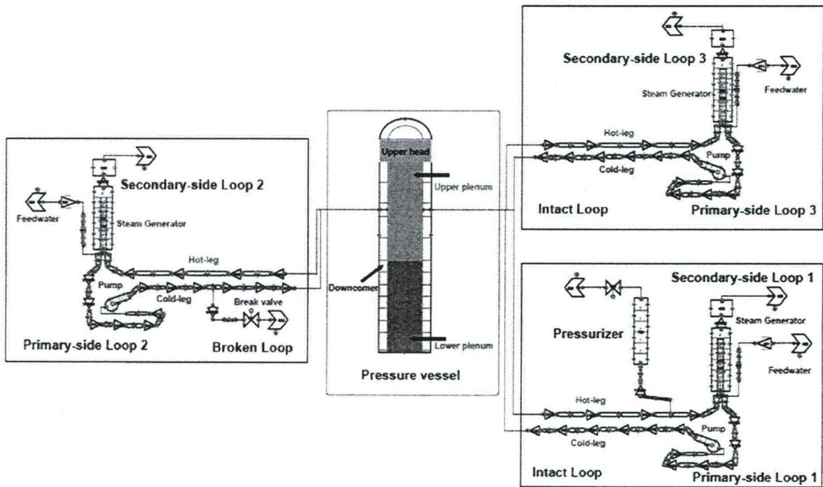
Fig. 3.2 The TRACE IIST facility model (model B)
