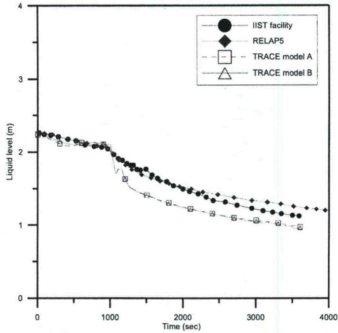
Fig. 4.24 The comparison of SG1 collapsed liquid level among IIST facility, RELAP5, TRACE in the C61210 experiment
