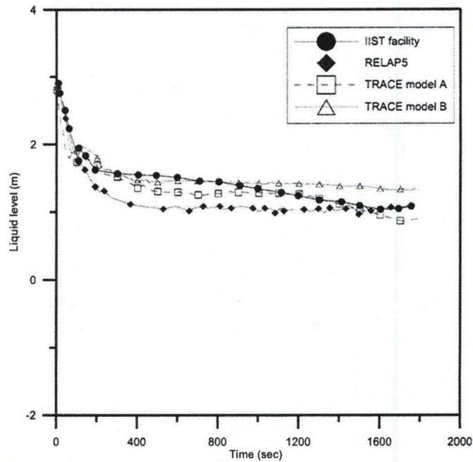
**Fig. 4.13 The comparison of core collapsed liquid level among IIST facility, RELAP5, TRACE in the SBLOCA experiment**
