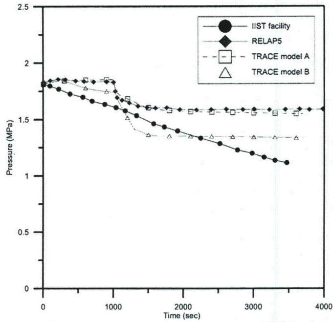
**Fig. 4.29** The comparison of Primary system pressure among IIST facility, RELAP5, TRACE in the C70122 experiment
