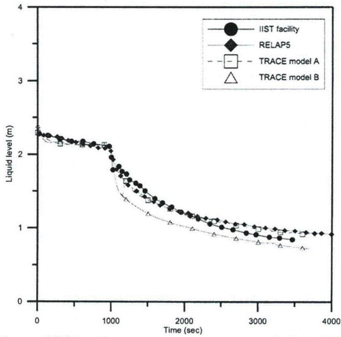
**Fig. 4.31 The comparison of SG1 collapsed liquid level among IIST facility, RELAP5, TRACE in the C70122 experiment**
