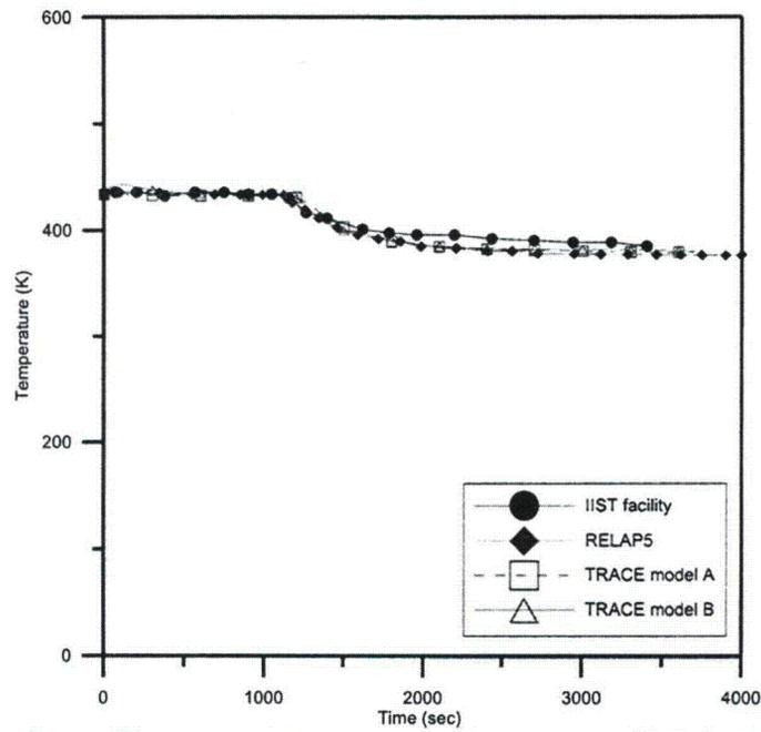
Fig. 4.35 The comparison of loop 1 cold-leg temperature among IIST facility, RELAP5, TRACE in the C70122 experiment
