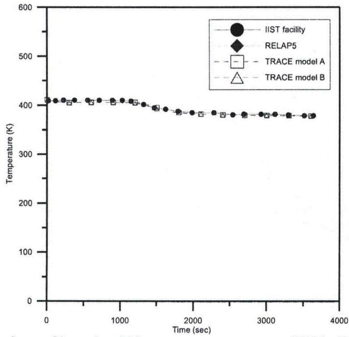
**Fig. 4.21 The comparison of loop 1 cold-leg temperature among IIST facility, RELAP5, TRACE in the C61128 experiment**
