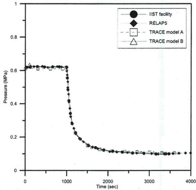
**Fig. 4.30** The comparison of SG1 secondary side pressure among IIST facility, RELAP5, TRACE in the C70122 experiment
