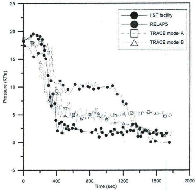
**Fig. 4.5 The comparison of SG2-inlet tube top differential pressure among IIST facility, RELAP5, TRACE in the SBLOCA experiment**
