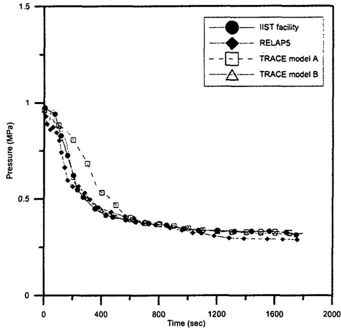
**Fig. 4.1 The comparison of primary system pressure among IIST facility, RELAP5, TRACE in the SBLOCA experiment**
