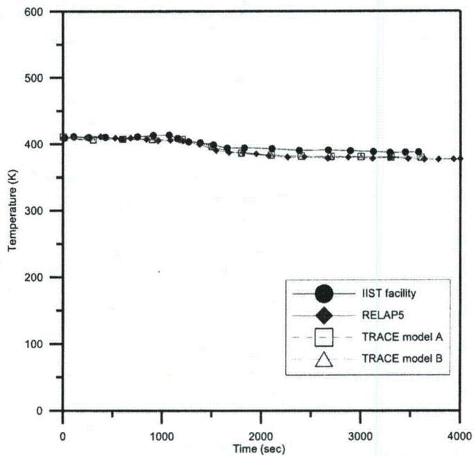
**Fig. 4.28 The comparison of loop 1 cold-leg temperature among IIST facility, RELAP5, TRACE in the C61210 experiment**
