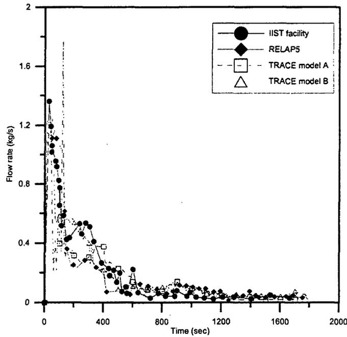
**Fig. 4.2 The comparison of break flow rate among IIST facility, RELAP5, TRACE in the SBLOCA experiment**
