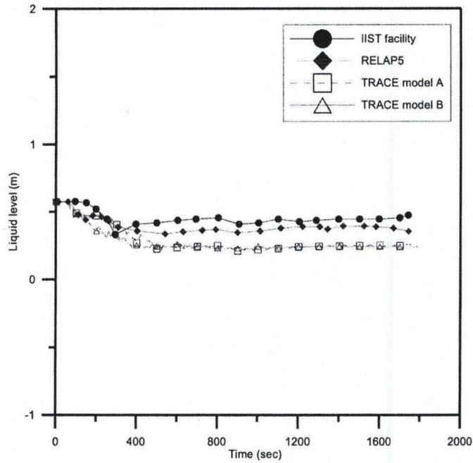
**Fig. 4.9 The comparison of SG2-inlet plenum liquid level among IIST facility, RELAP5, TRACE in the SBLOCA experiment**
