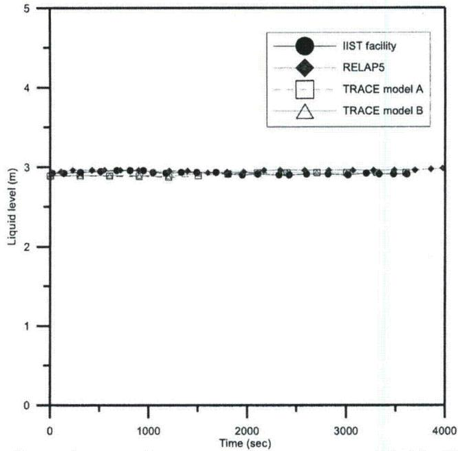
**Fig. 4.19 The comparison of core collapsed liquid level among IIST facility, RELAP5, TRACE in the C61128 experiment**
