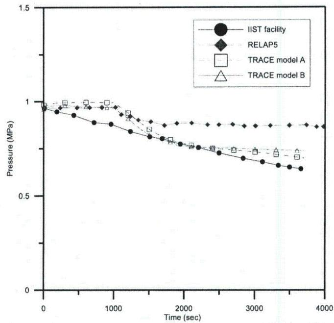
Fig. 4.15 The comparison of Primary system pressure among IIST facility, RELAP5, TRACE in the C61128 experiment
