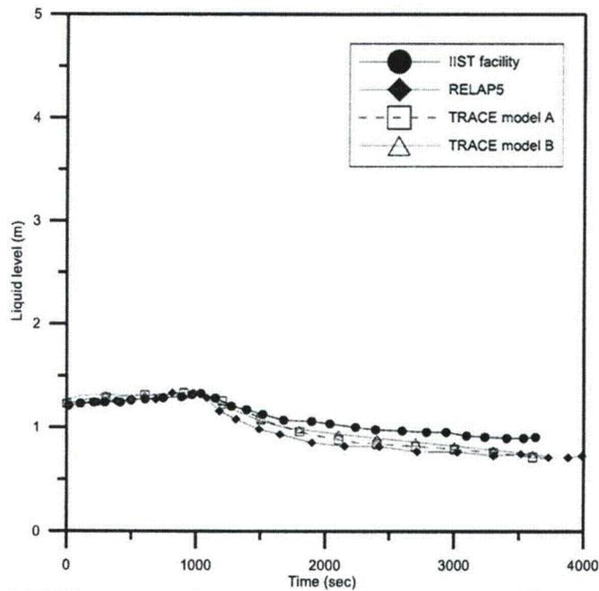
**Fig. 4.18** The comparison of pressurizer collapsed liquid level among IIST facility, RELAP5, TRACE in the C61128 experiment
