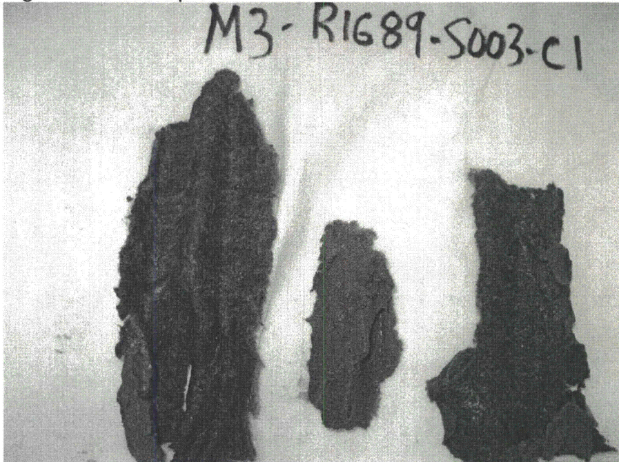
Figure 8: Close-Up of a Piece of Debris Bed Removed from the Strainer Surface
