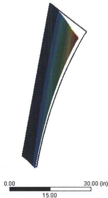
Figure RAI-20 S01 - 1 - Displacement of ribbed (Model A) and uniform (Model B) plates under rigid transverse forcing.
