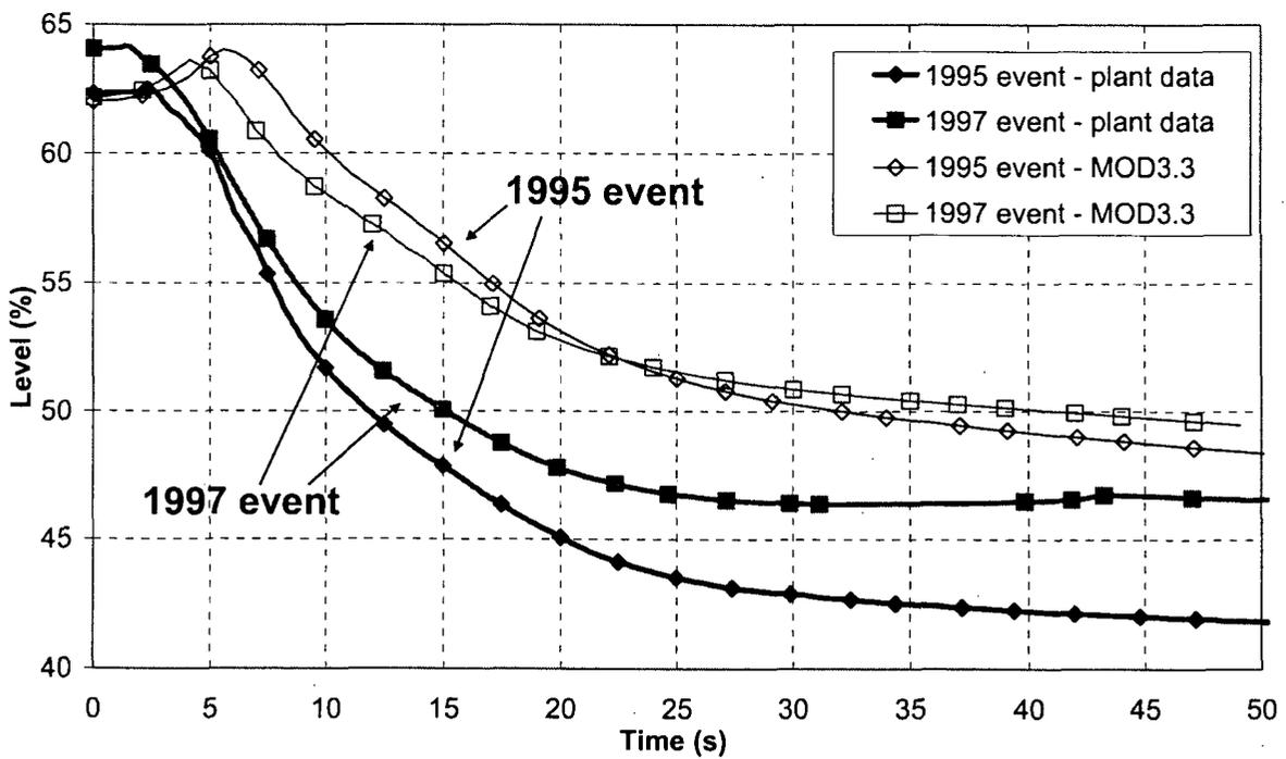
Figure 7 Pressurizer level
