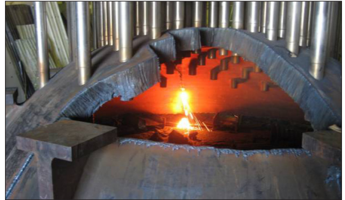
Figure 4.2 Sectioning of reactor vessel head penetrations from Washington Nuclear Power, Unit 1, a canceled plant
