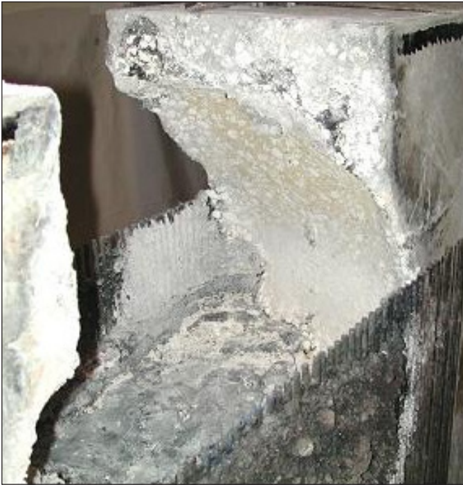
Figure 11.2: Posttest debris from CCI tests
