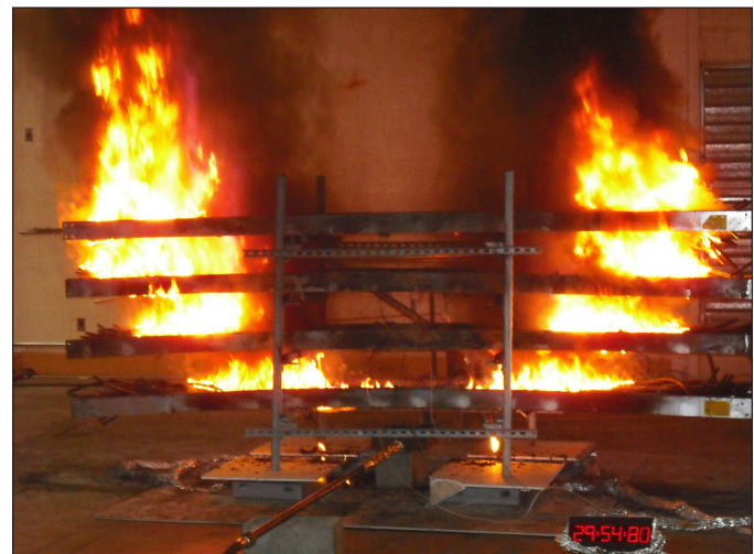
Figure 2.5 Cable tray fire test
