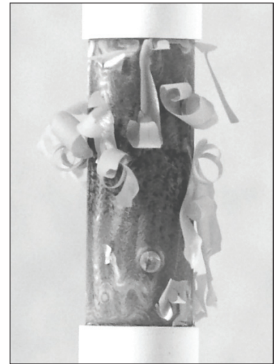
Figure 7.11 Oxidation of a foreign niobium-bearing cladding alloy under LOCA conditions
