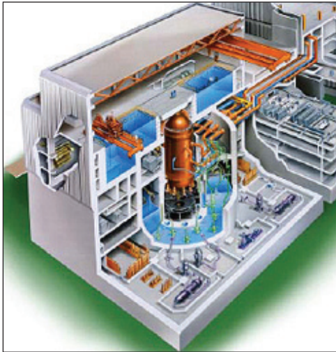
Figure 5.5 Advanced Boiling-Water Reactor (ABWR)
