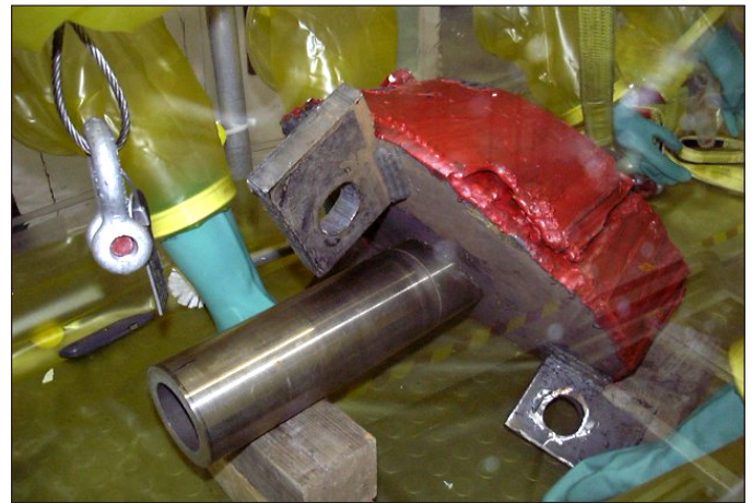
Figure 4.3 Non-destructive and destructive examination of salvaged control rod drive mechanism penetrations and J-groove welds from North Anna, Unit 2
