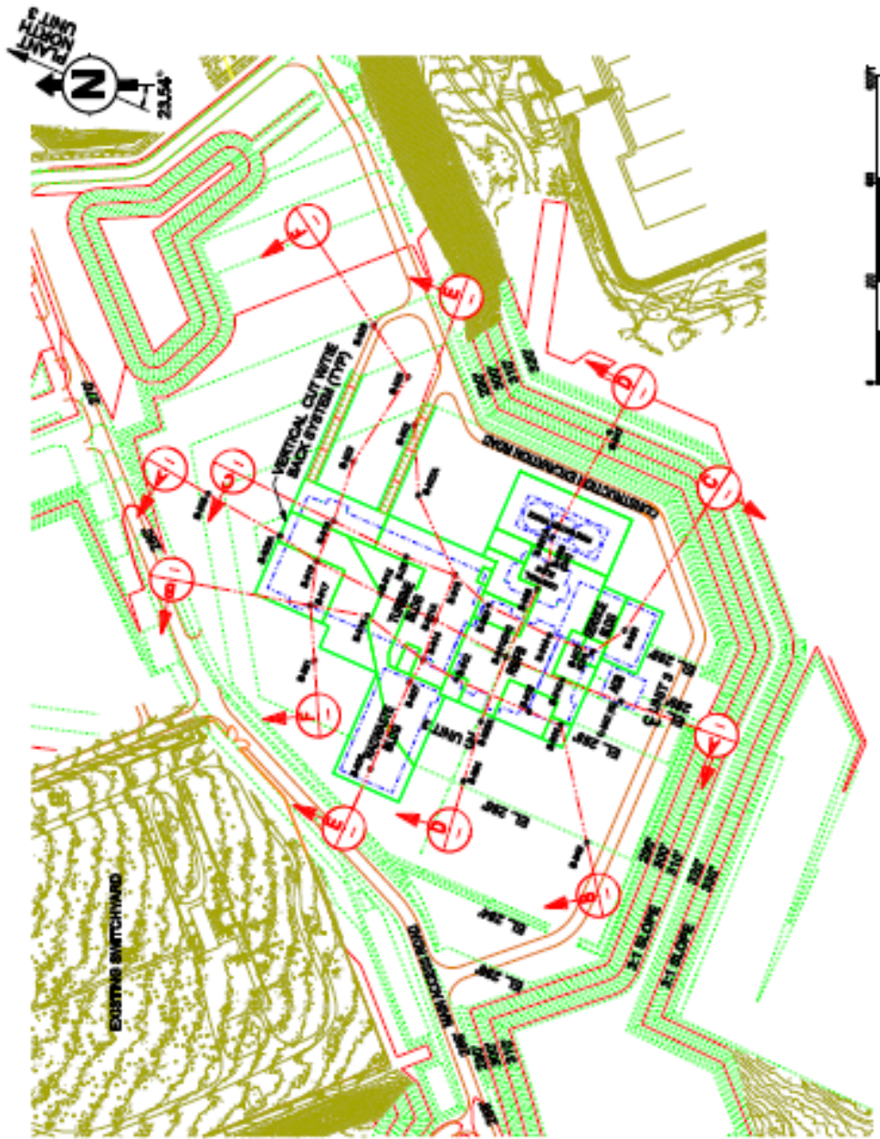
Figure 2.5.4-7 Plans for Excavation (FSAR Figure 2.5-214)
