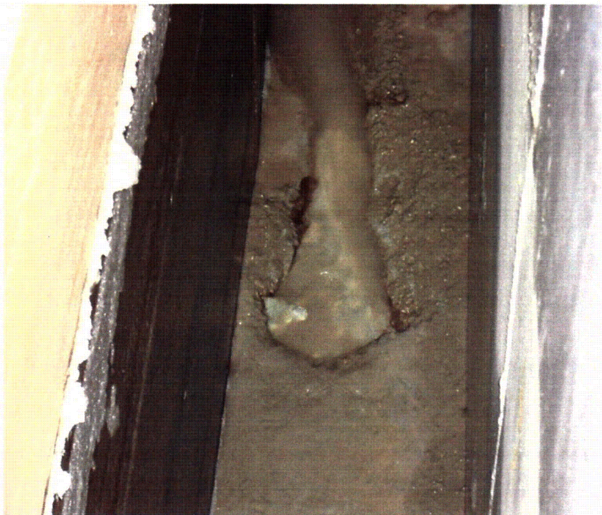
Figure 17-2 Zoomed View Of Debris Settled On Test Flume Floor During Drain Down
