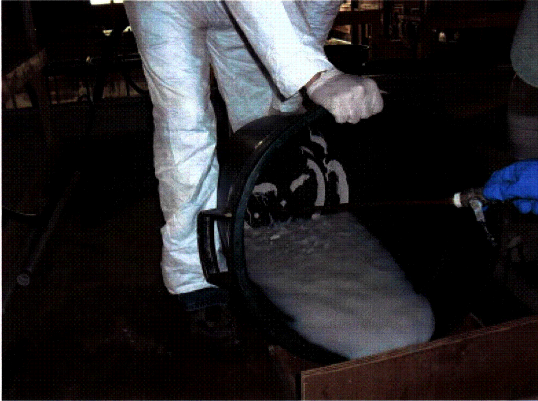
Figure 15-4: Particulate Debris being Rinsed into the Test Flume
