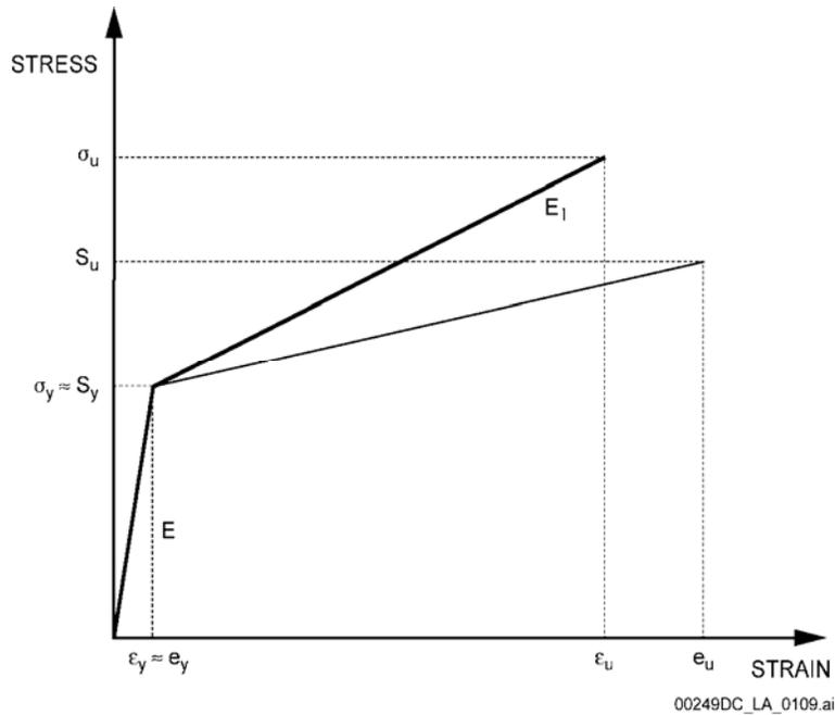
Figure 5. Key Attributes of Bi-linear Stress-Strain Curves
