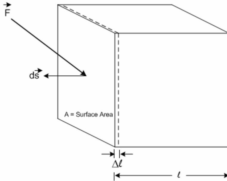
Figure 8. Forces on Element inducing Deformation
