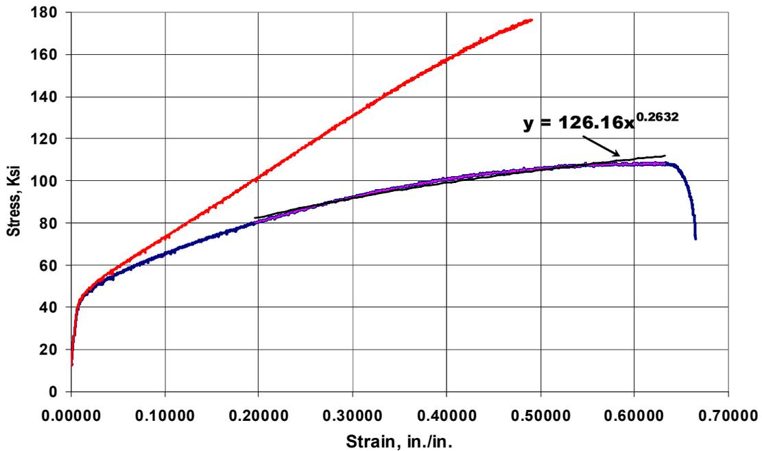
Figure I-6. Alloy 22 Stress-Strain Curve
