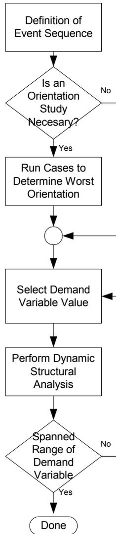
Figure 11. Flowchart for Dynamic Structural Analyses
