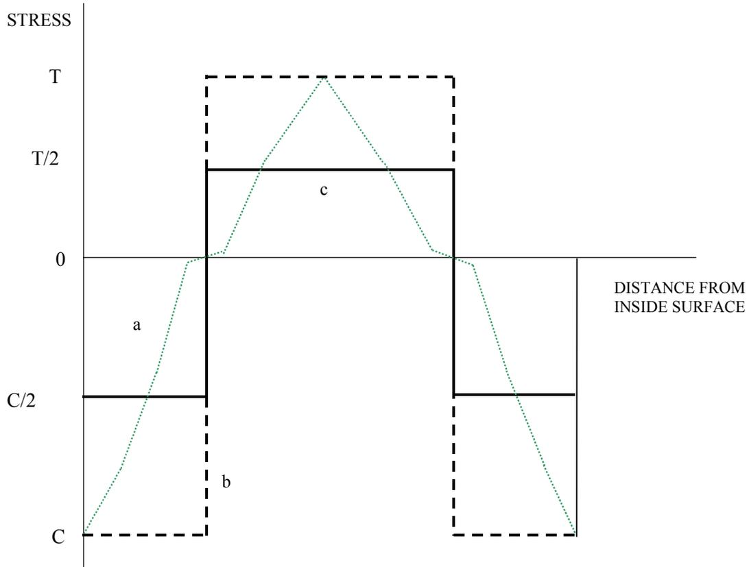
NOTES: (a) Schematic representation of axial and hoop stress distribution from Herrera et al. (2002 [DIRS 166799], Figures 48 and 52) (green dotted line), (b) first (“full”) approximation (dashed line), and (c) second (“half”) approximation (solid line).
