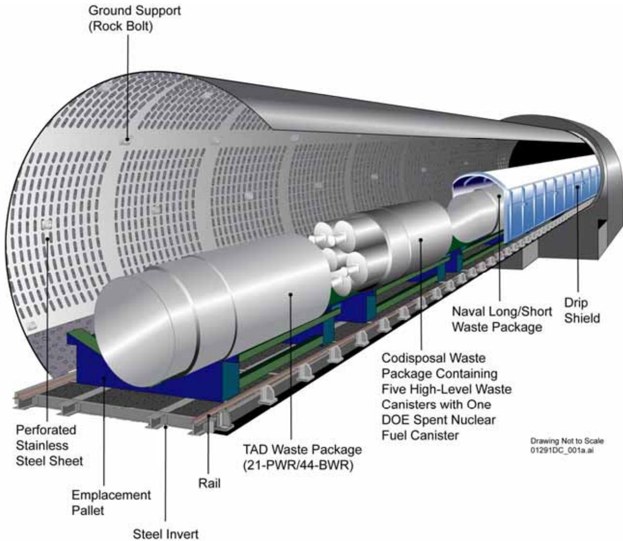
Figure B. Cutaway View of Different Waste Packages in a Repository Drift
