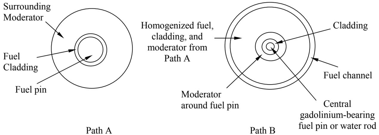
Figure 19. SCALE Representation of BWR Fuel Pin Cell and Assembly for SAS2H Calculations
