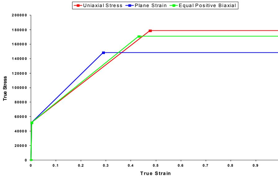
Figure I-10. Alloy 22 Tri-linear Material
