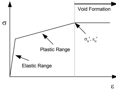
Figure 9. Tri-linear Stress-Strain Curve
