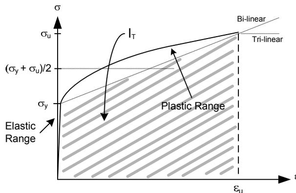
Figure 7. Illustration of Physical Basis for Toughness Index
