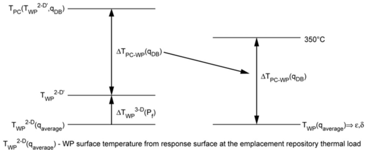
$T_{WP}^{2-D}(q_{average})$  - WP surface temperature from response surface at the emplacement repository thermal load
