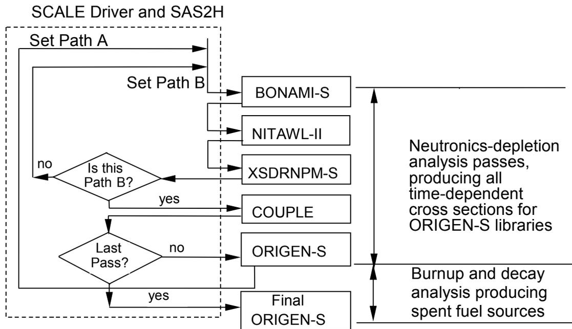
Figure 20. Computational Flow for Source Term Generation in SAS2H
