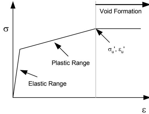
Figure I-8. Tri-linear Stress-Strain Curve
