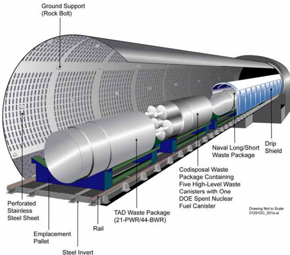
Figure 2. Cutaway View of Different Waste Packages in a Repository Drift
