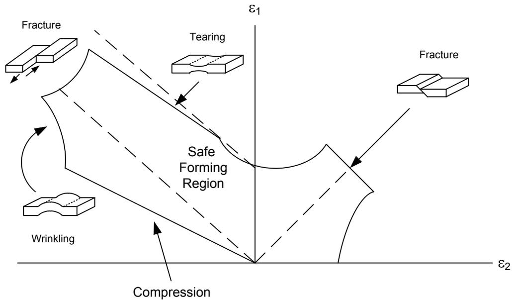
Figure I-1. Four Bi-axial Membrane Strain Safe Forming Region
