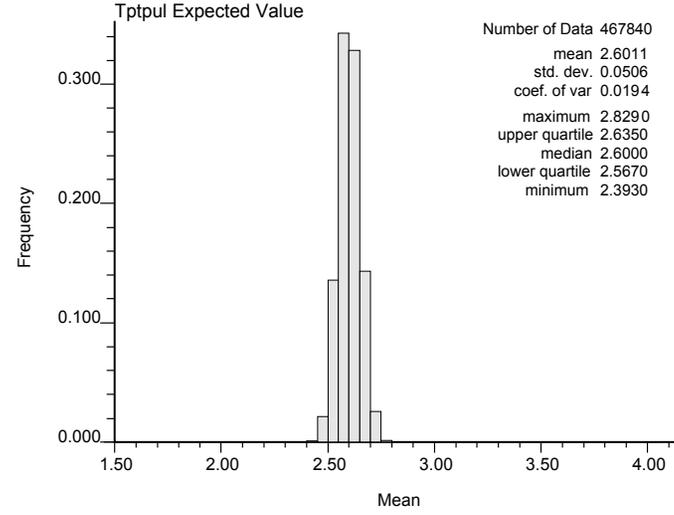
Figure 6-37. Solid Conductivity in the Tptpul,  $k_s$
