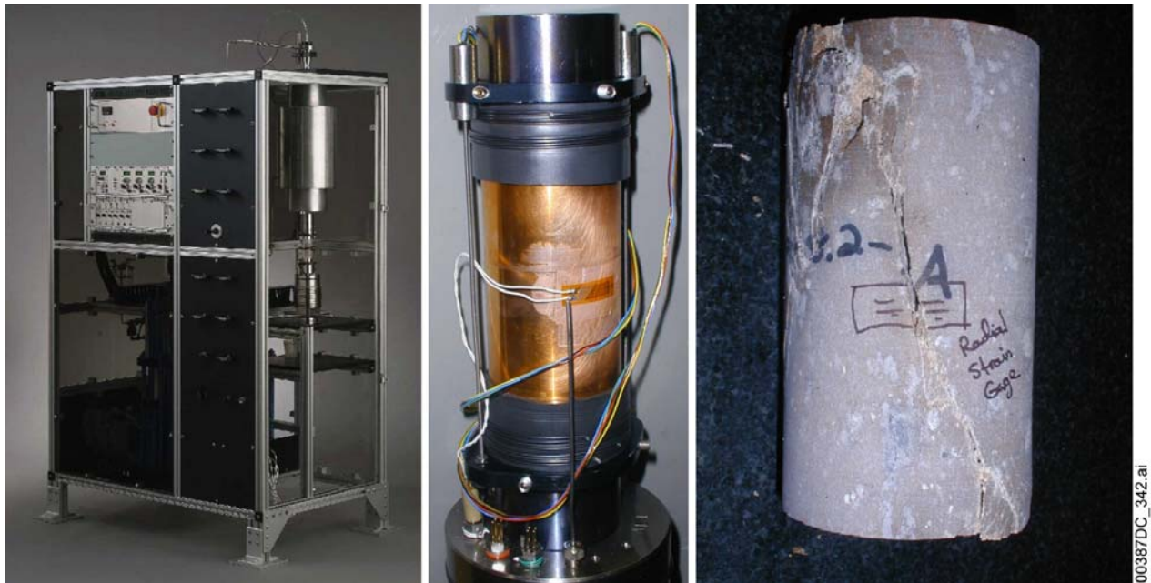
Figure 6-154. Triaxial Static Fatigue Experimental Setup and Posttest Sample for Heated, Saturated, 50.8 mm Diameter Samples of Tptpmn
