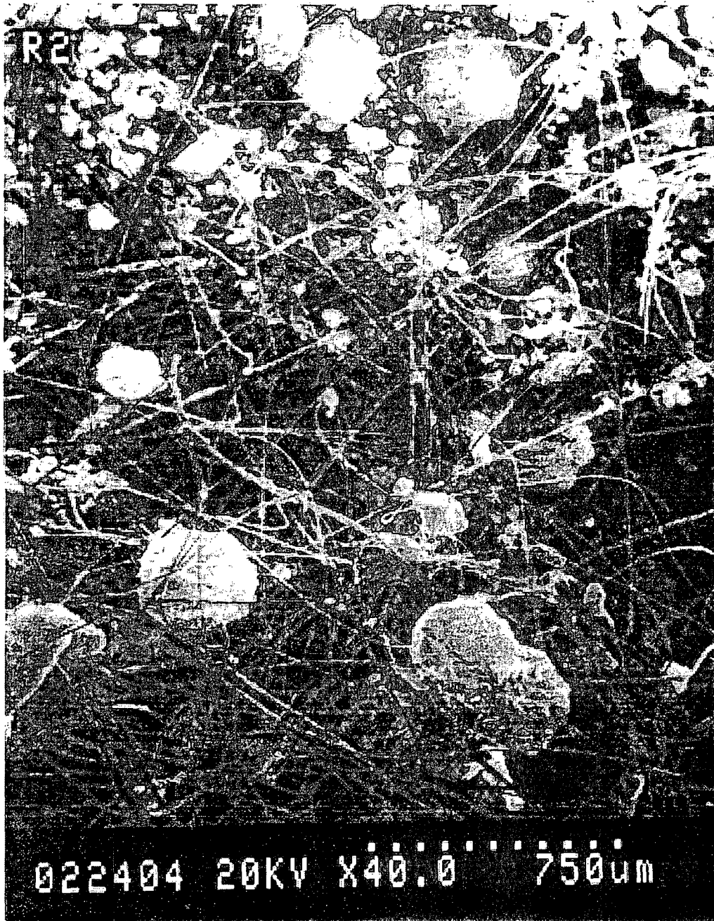
Figure E-23 SEM of a Typical Mixed Debris Bed (750 μm magnification)
