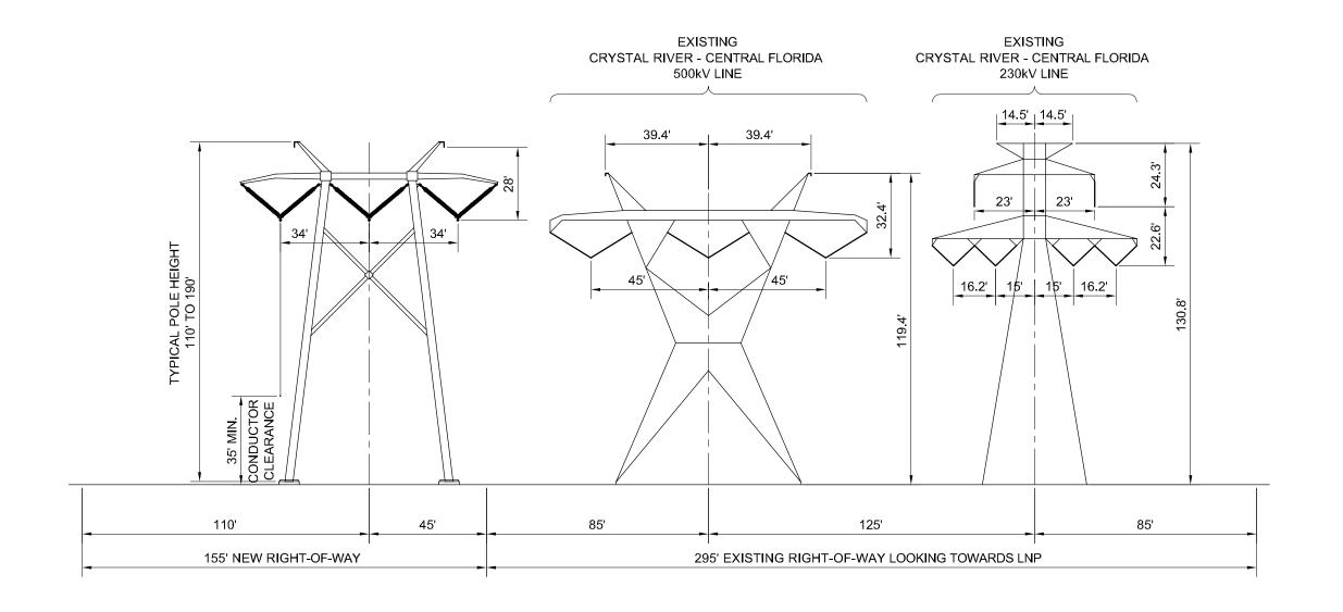
1. TYPICAL PIER FOUNDATION TO BE 5' TO 8' IN DIAMETER.
