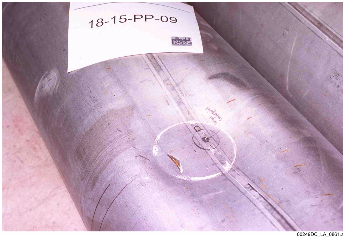
Figure 1.5.1-27. Deformed Shape of Standardized Canister for 40-in. Drop onto a 6-in. Post (Isometric View)
