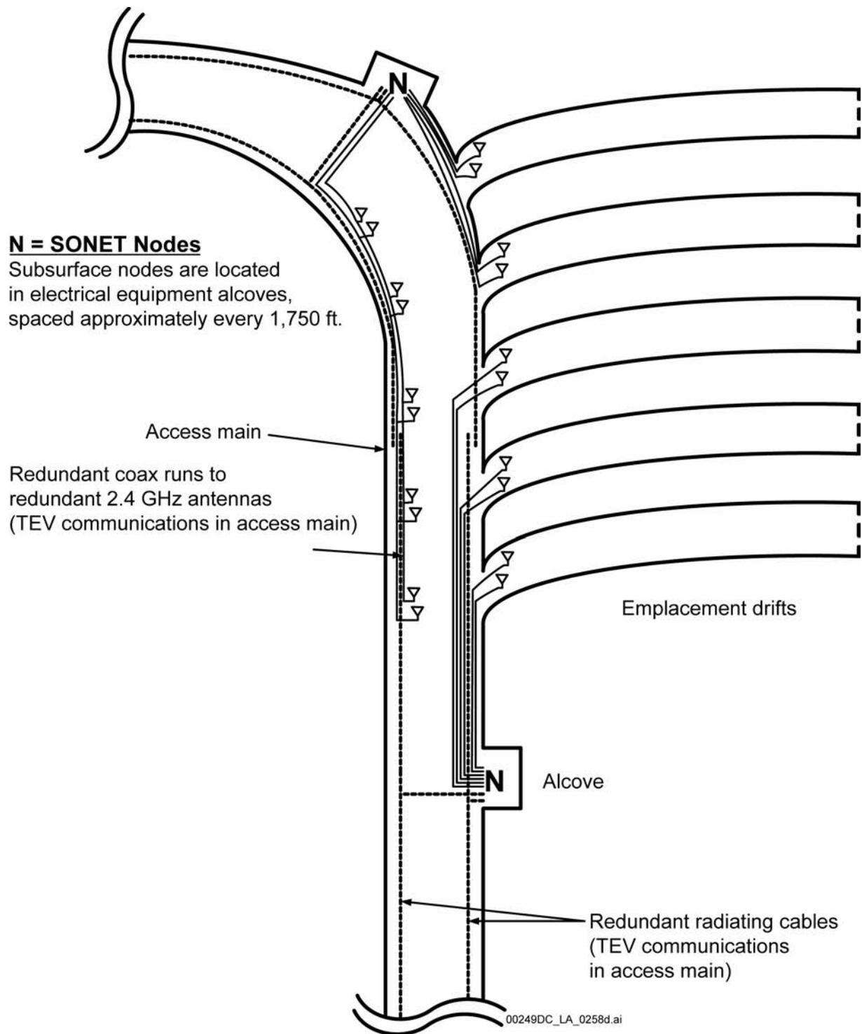
Figure 1.4.2-9. Site Topology—Wireless Configuration—Main and Emplacement Drifts
