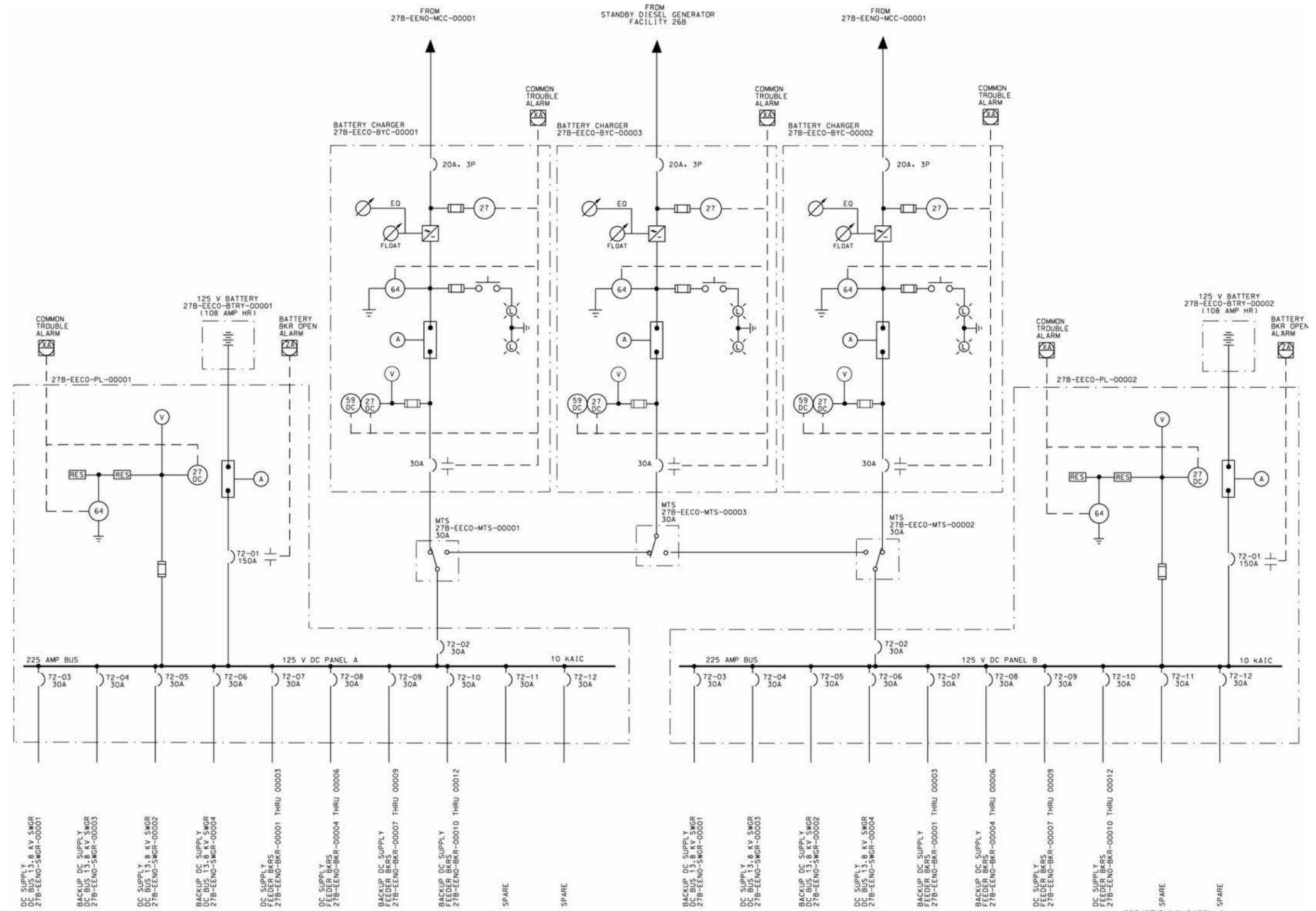
NOTE: Relays numbered "27" indicate under voltage relays, relays numbered "59" indicate over voltage relays, and relays numbered "64" indicate ground fault relays. This figure includes no SSCs that are either ITS or ITWI.
