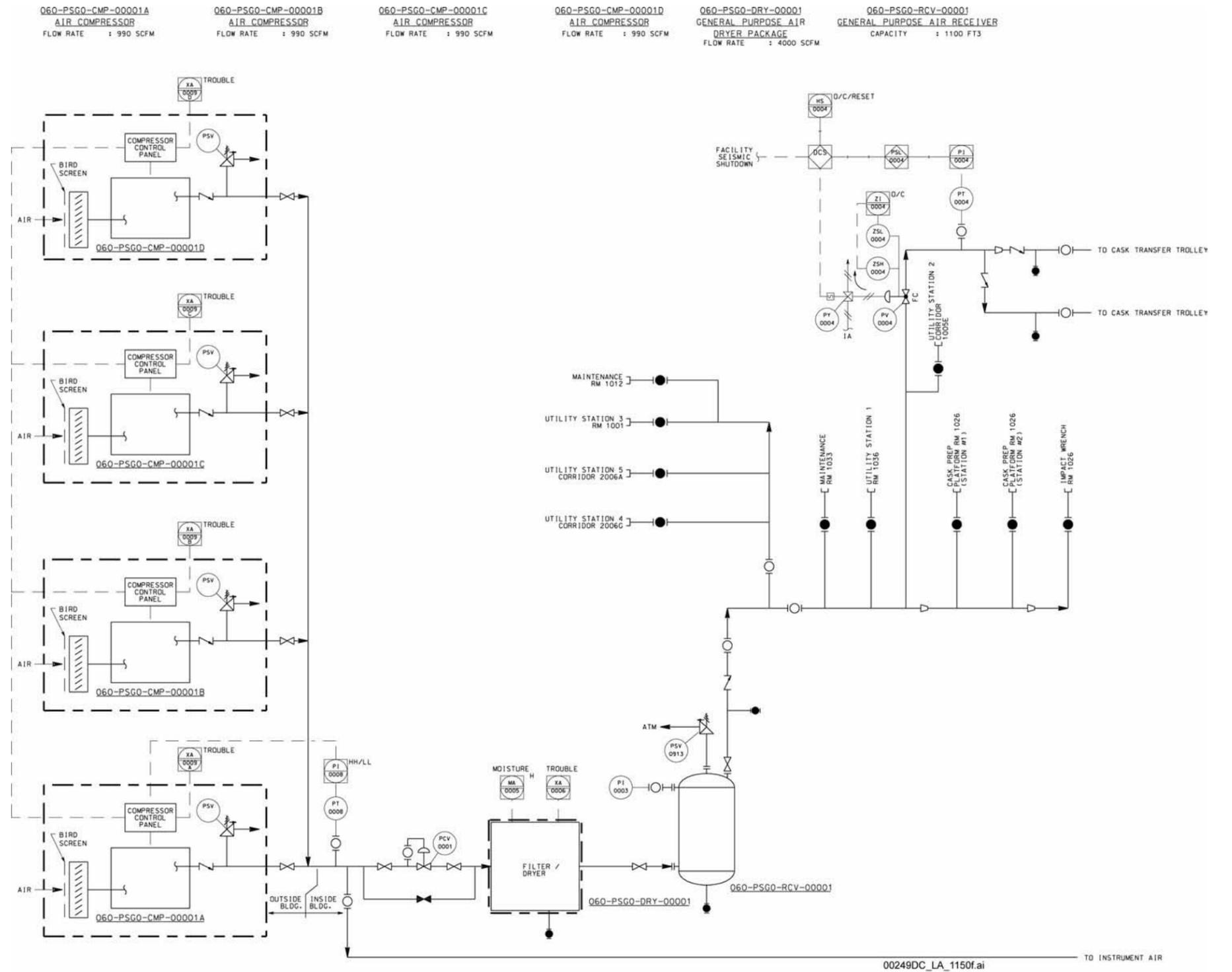
NOTE: PCV = pressure control valve; PI = pressure indicator;
