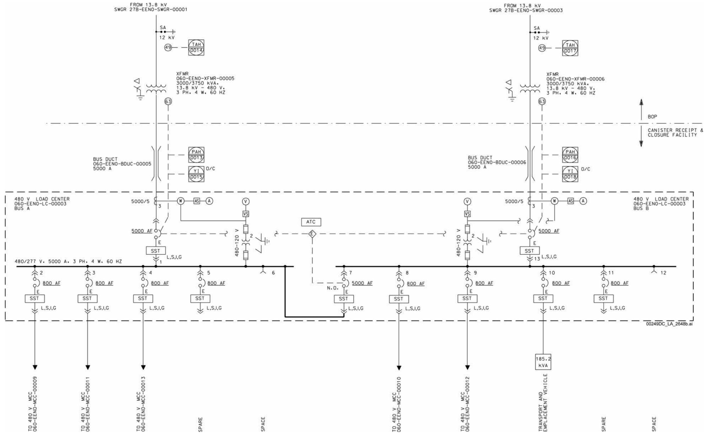
NOTE: The one tie and two incoming breakers are electrically interlocked to prevent all three from being closed at the same time. Auto transfer control provides automatic bus transfer upon failure of one source. This figure includes no SSCs that are either ITS or ITWI.
