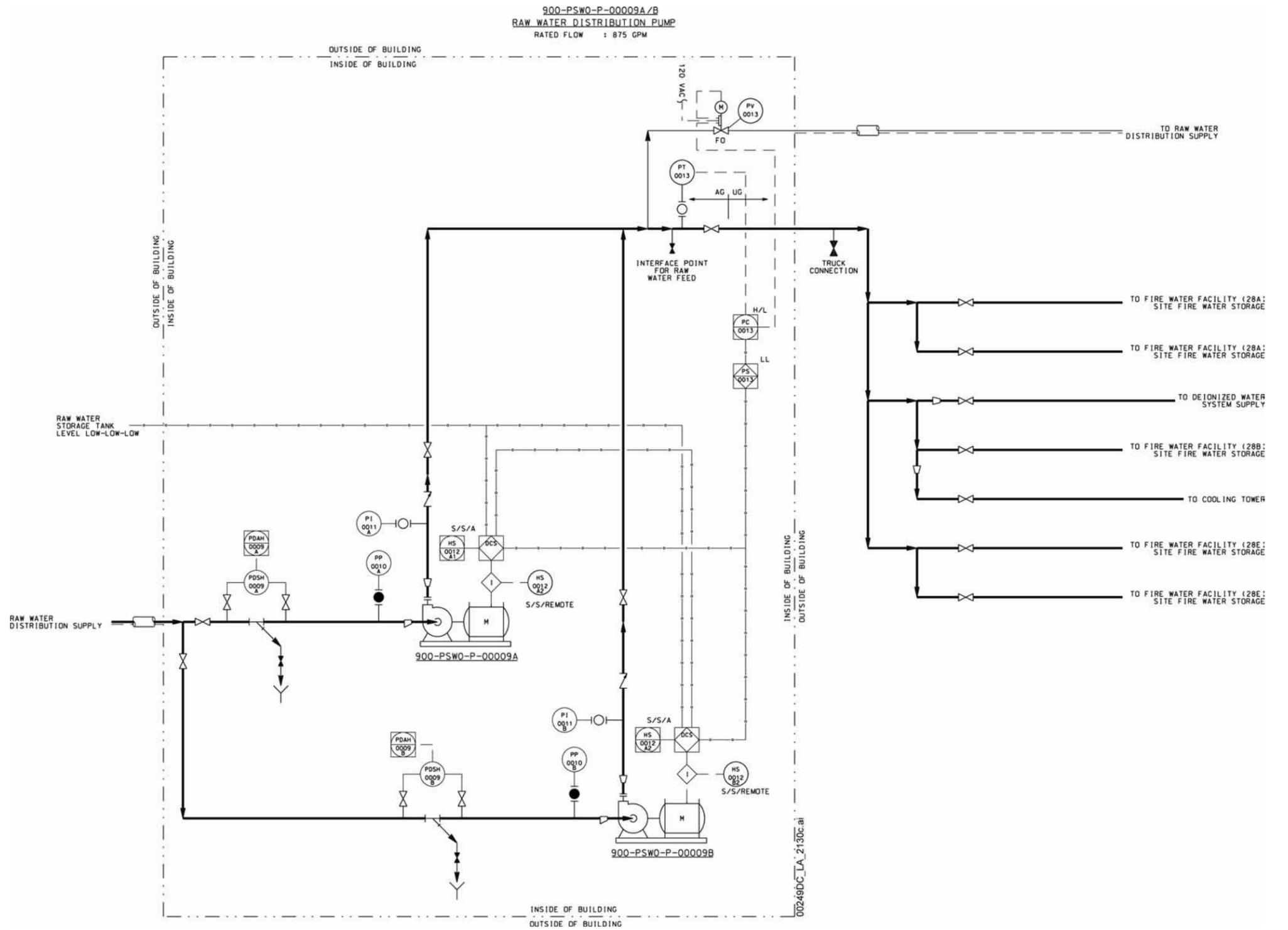
Figure 1.4.4-6. Infrastructure Raw Water System Supply and Distribution Piping and Instrumentation Diagram (Sheet 2 of 2)
