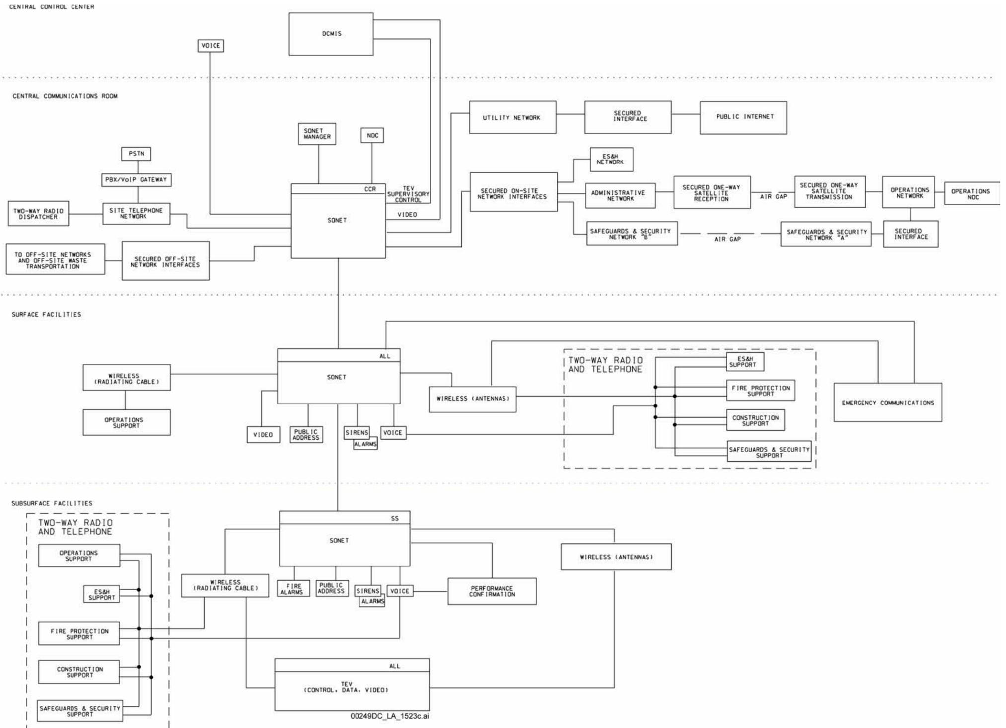
NOTE: Emergency communications include data, video, and voice feeds to the Emergency Operations Center, backup emergency operations center, and offsite locations.
