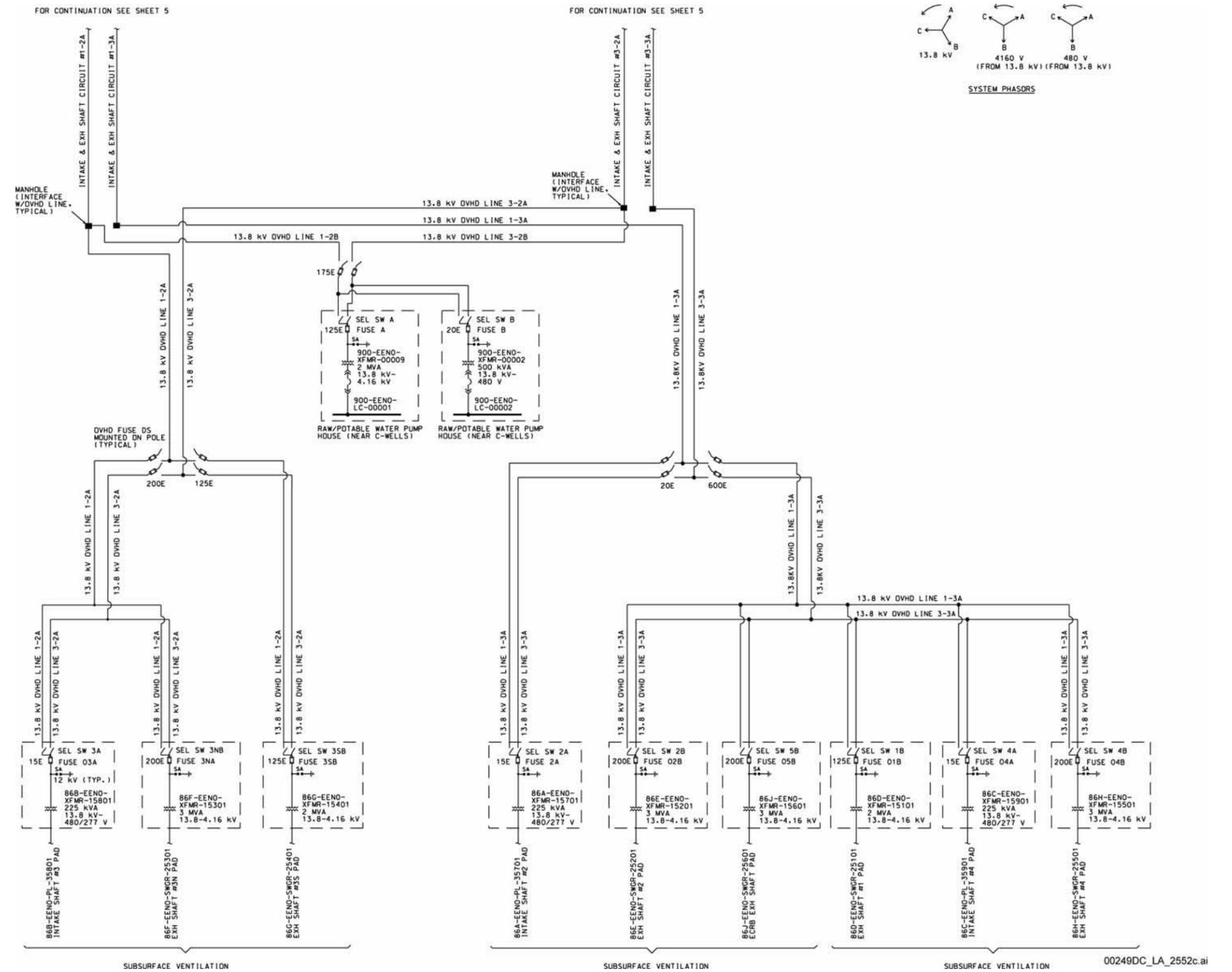
Figure 1.4.1-2. 13.8 kV Normal Power Distribution Main Single Line (Sheet 2 of 6)
