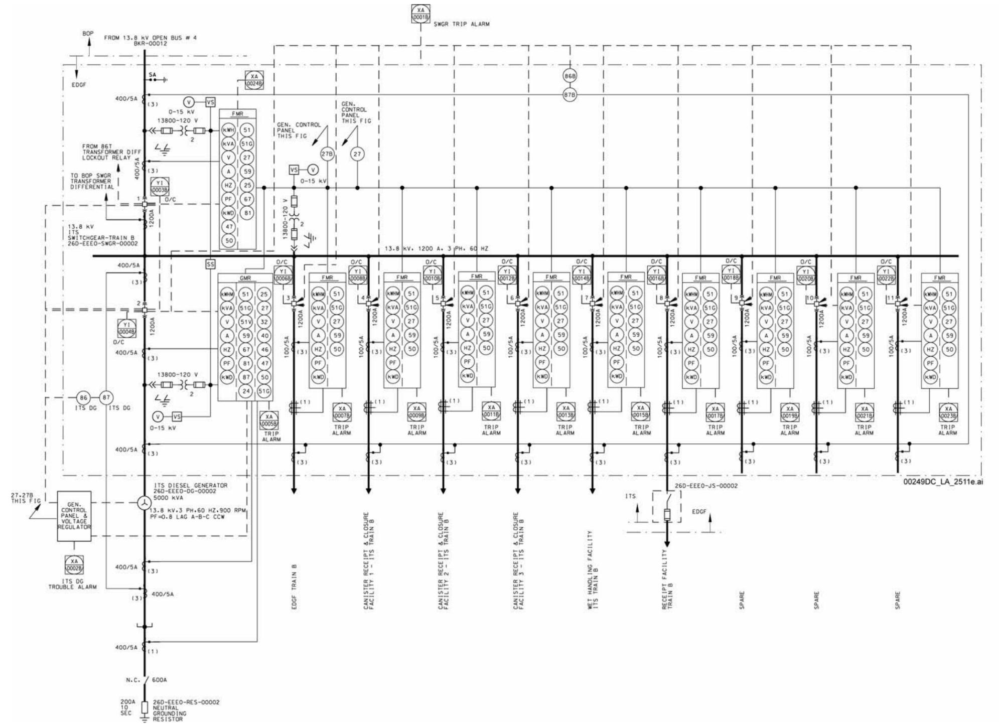
Figure 1.4.1-11. Emergency Diesel Generator Facility ITS Train B 13.8 kV Single Line Diagram
