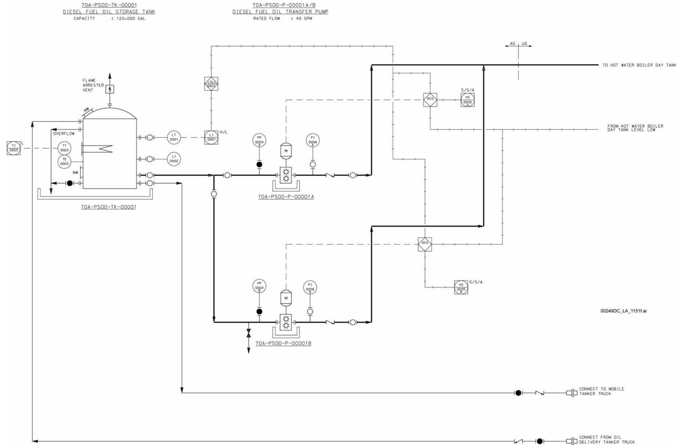
NOTE: FT = flow transmitter; PI = pressure indicator.
