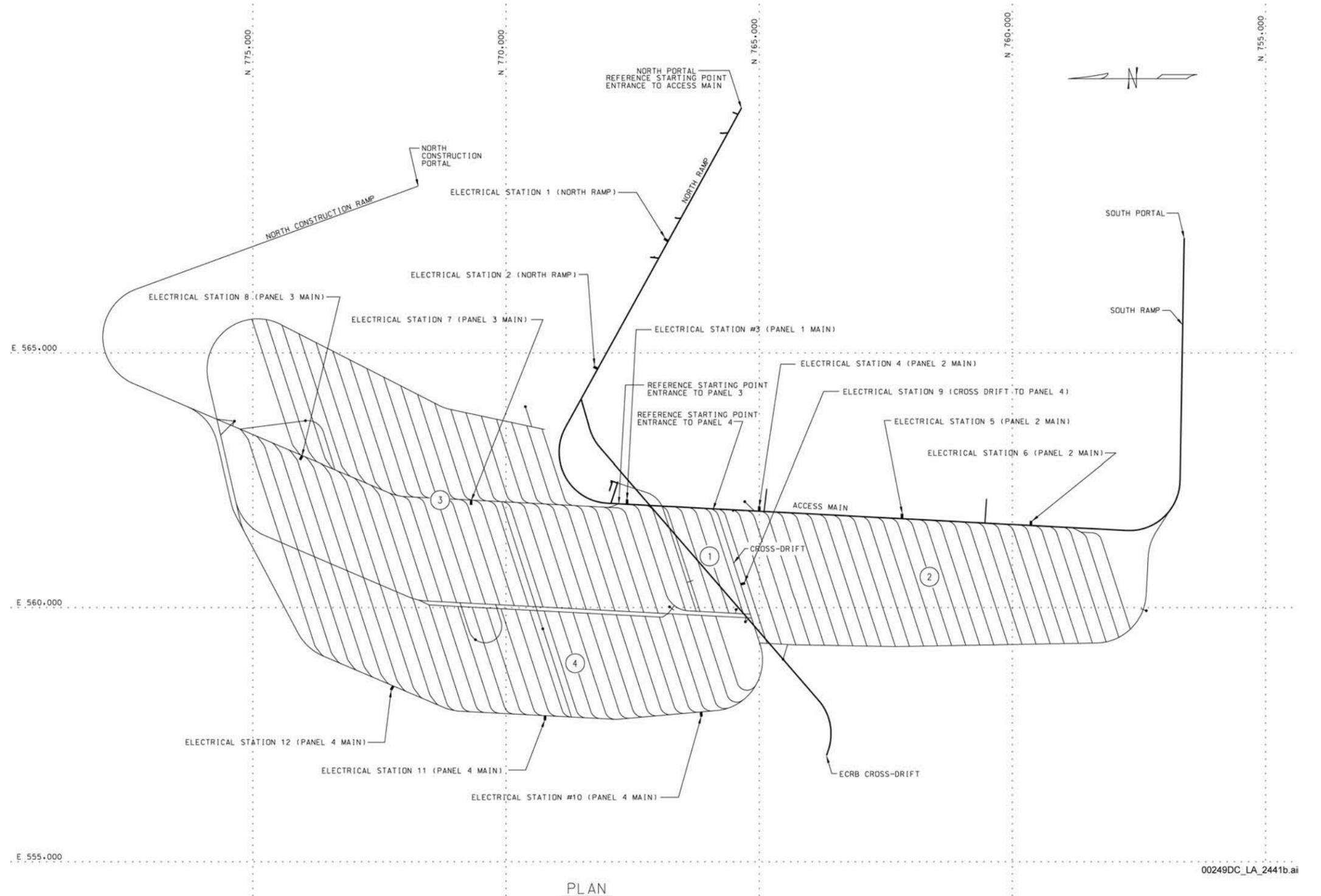
Figure 1.4.1-6. Subsurface Facility Access Main Electrical Station Location
