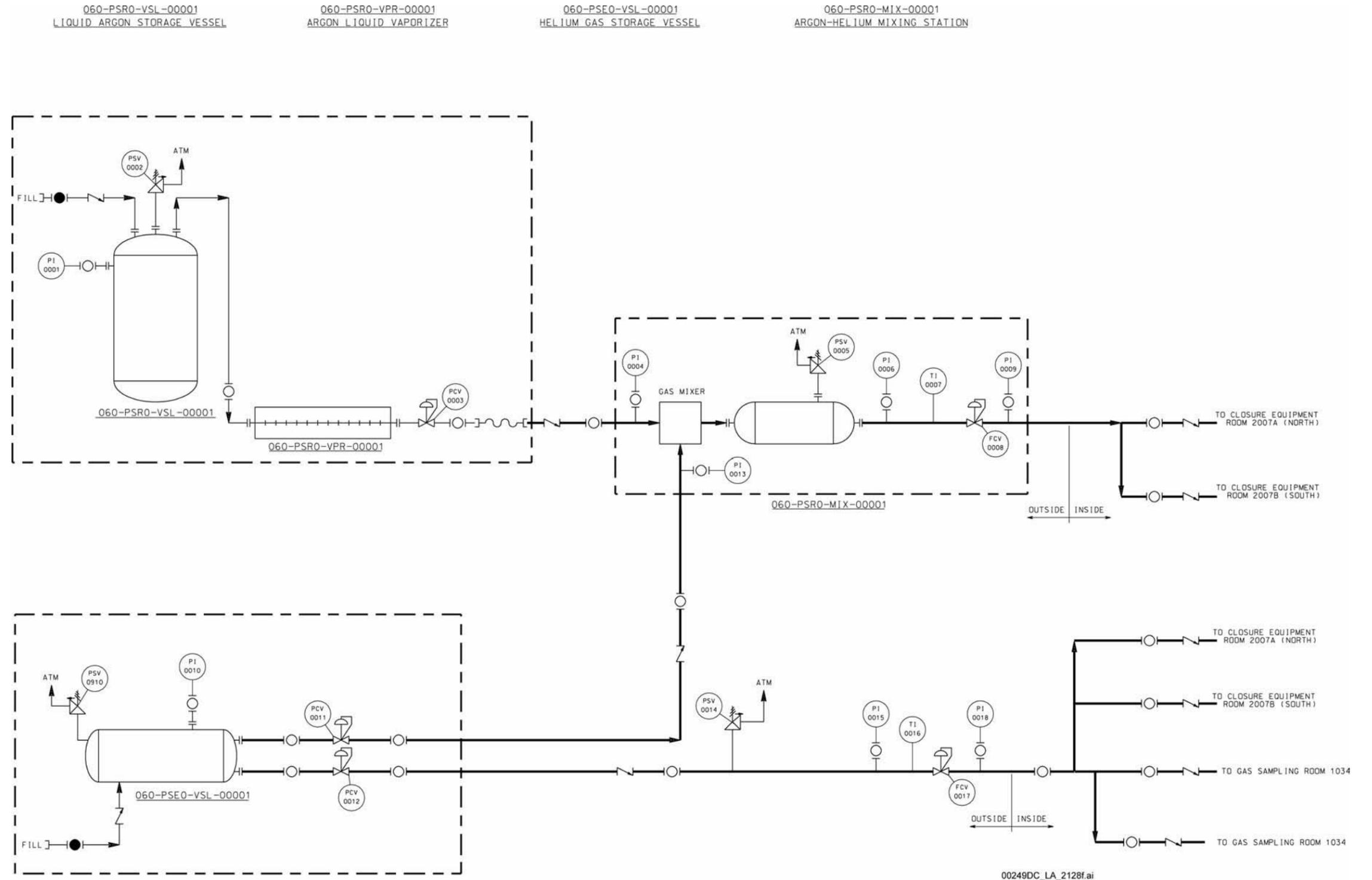
Figure 1.4.4-4. Canister Receipt and Closure Facility Helium and Argon Gas Supply and Distribution System Piping and Instrumentation Diagram
