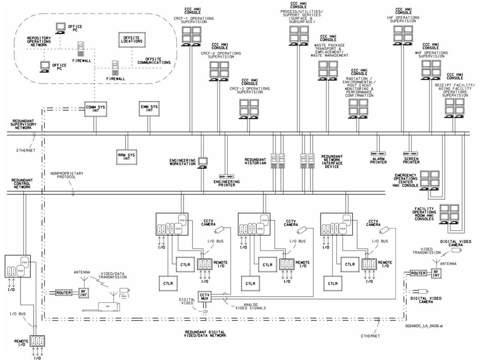
NOTE: CCC = Central Control Center; CCTV = closed-circuit television; EMM = environmental/meteorological monitoring; FDI = foreign device interface; HMI = human-machine interface; I/O = input-output; MUX = multiplexer; PC = personal computer; RF = radio frequency; RRM = radiation/radiological monitoring.
