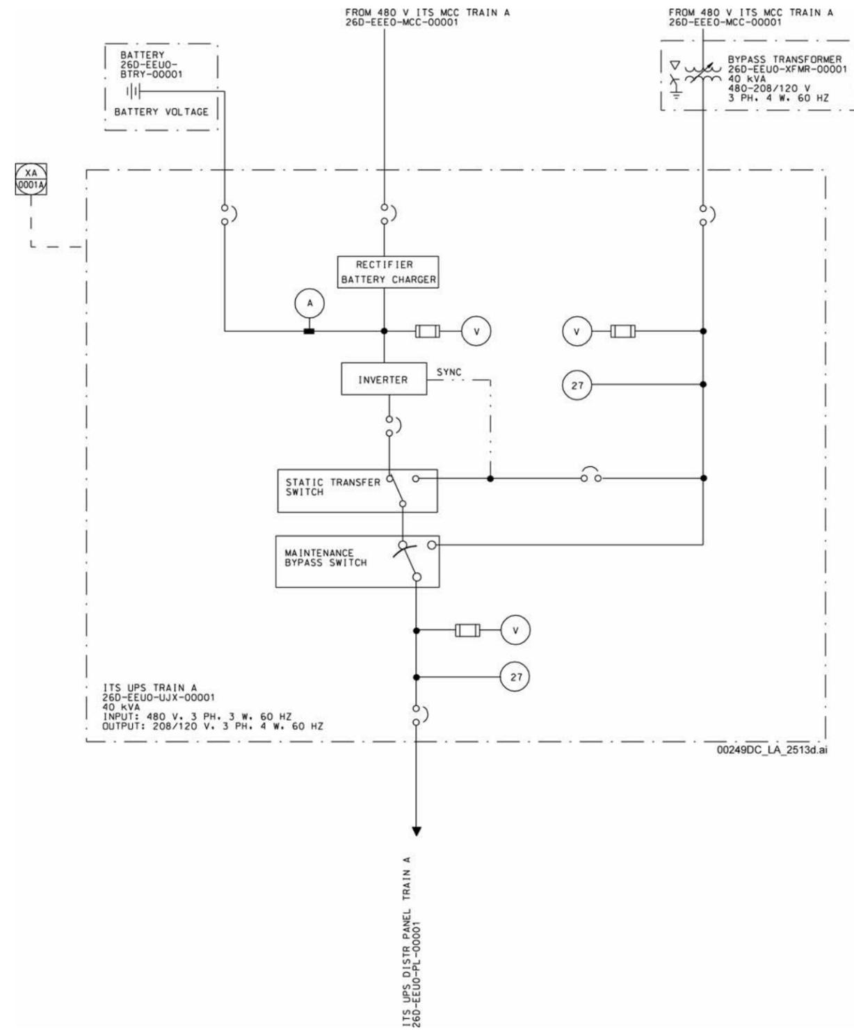
Figure 1.4.1-26. Emergency Diesel Generator Facility ITS Train A Uninterruptible Power Supply Single Line Diagram
