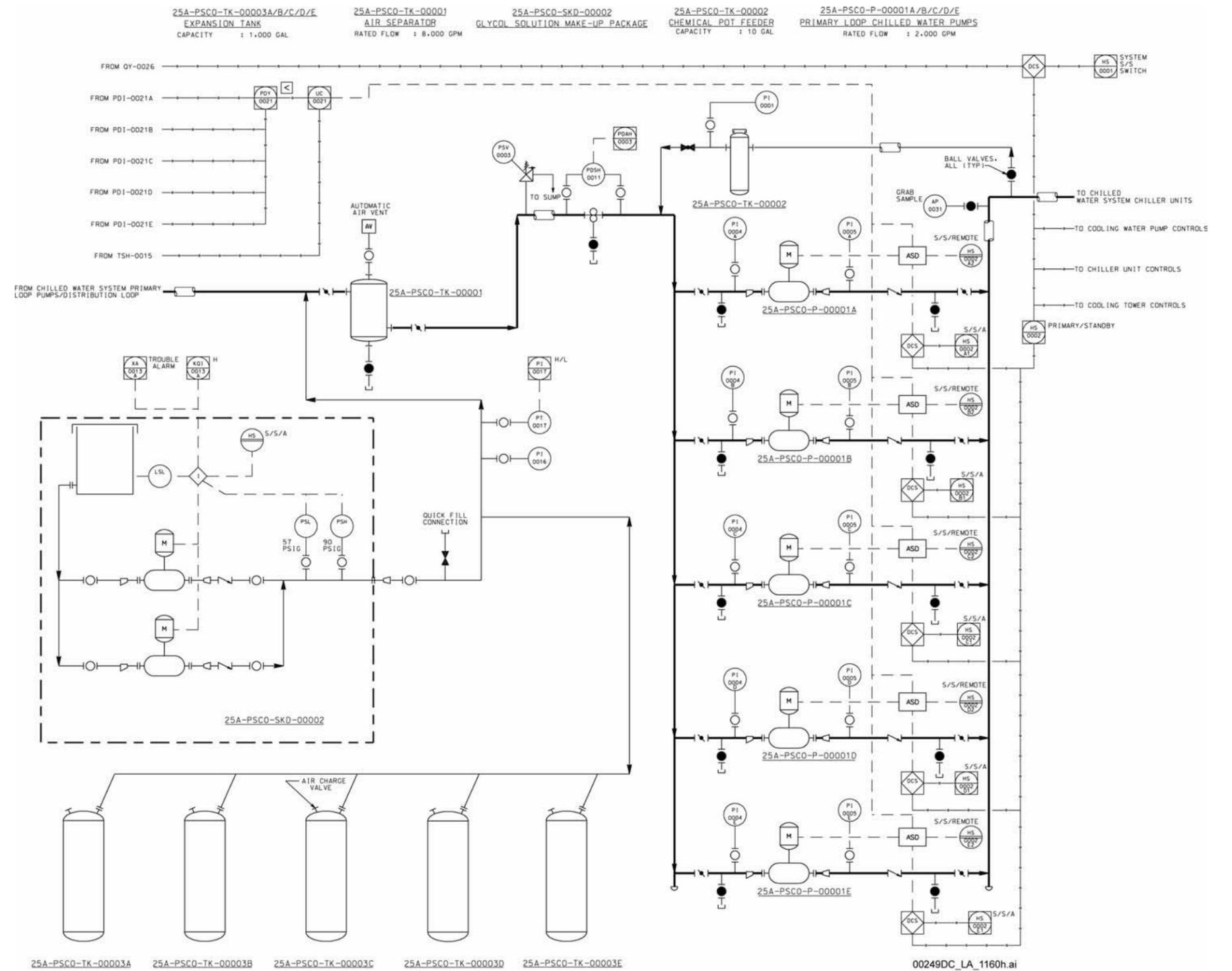
NOTE: ASD = adjustable speed drive; CHWR = chilled water return; CHWS = chilled water supply; FS = flow switch; TWR = cooling tower water return; TWS = cooling tower water supply.
