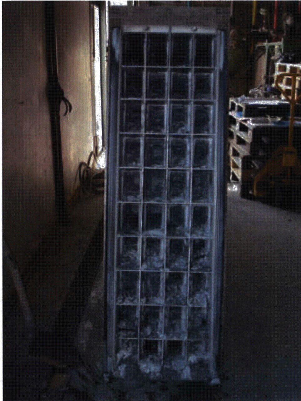
Photo 3o – 5 Test No. 4, Strainer Module after Dismounting
