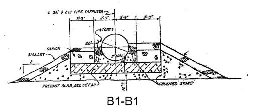
FIGURE 5.3-2 Cooling Tower Blowdown Diffuser Pipe
