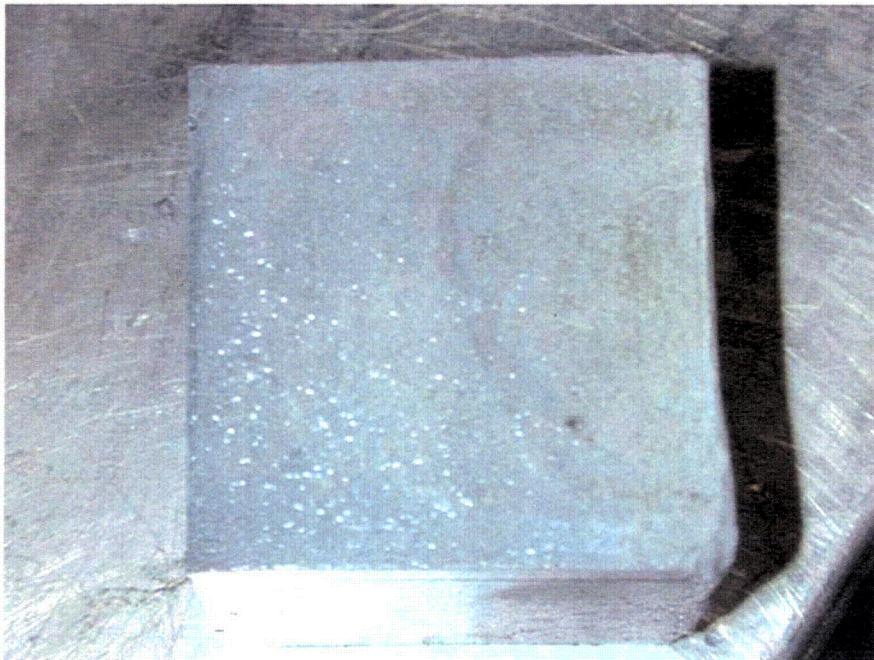
Figure 5.8 Cube specimen after 1 month in \text{Na}_2\text{HPO}_4 .
