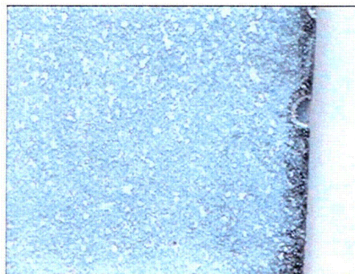
Figure 5.40 \text{CaCO}_3 deposits on surface of specimen cured in \text{Ca}(\text{OH})_2 .
