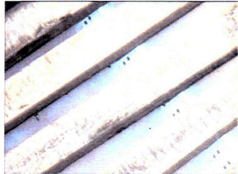
Figure 5.42 Close up of specimens after 18-month exposure in solution of \text{Na}_2\text{HPO}_4 .
