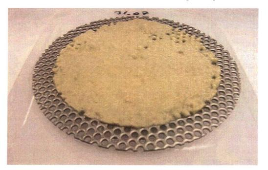
Figure 7.23. Incomplete Debris Bed from COBT5, Test 060510\_CO\_1763\_BP2. Target CalSil mass loading = 2175 g/m<sup>2</sup>, retrieved CalSil mass loading = 292 g/m<sup>2</sup>, 13% of target mass retained on screen, debris bed formed in the benchtop test loop.
