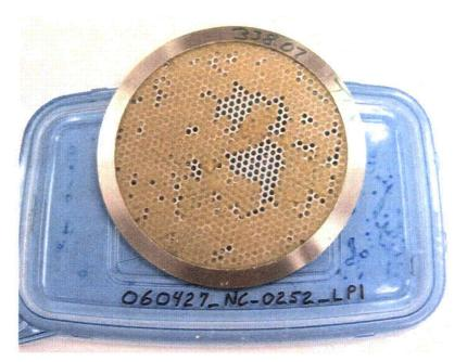
Figure 7.33. Incomplete Debris Bed Retrieved from Test NC1 with a Retrieved Mass Loading of 56.3 g/m<sup>2</sup>. The target mass loading was 108 g/m<sup>2</sup> NUKON, 27 g/m<sup>2</sup> CalSil, and 135 g/m<sup>2</sup> total.
