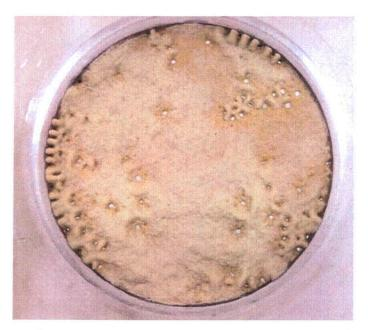
Figure 7.26. Incomplete Debris Bed from Test Condition CO1, Tests 060510\_CO\_8108\_LP1 Through LP3. Debris bed pictured within TTS, target CalSil mass loading = 4350 g/m<sup>2</sup>, retrieved CalSil mass loading = 434 g/m<sup>2</sup>, 10% of target mass retained on screen, debris bed formed in large-scale test loop.
