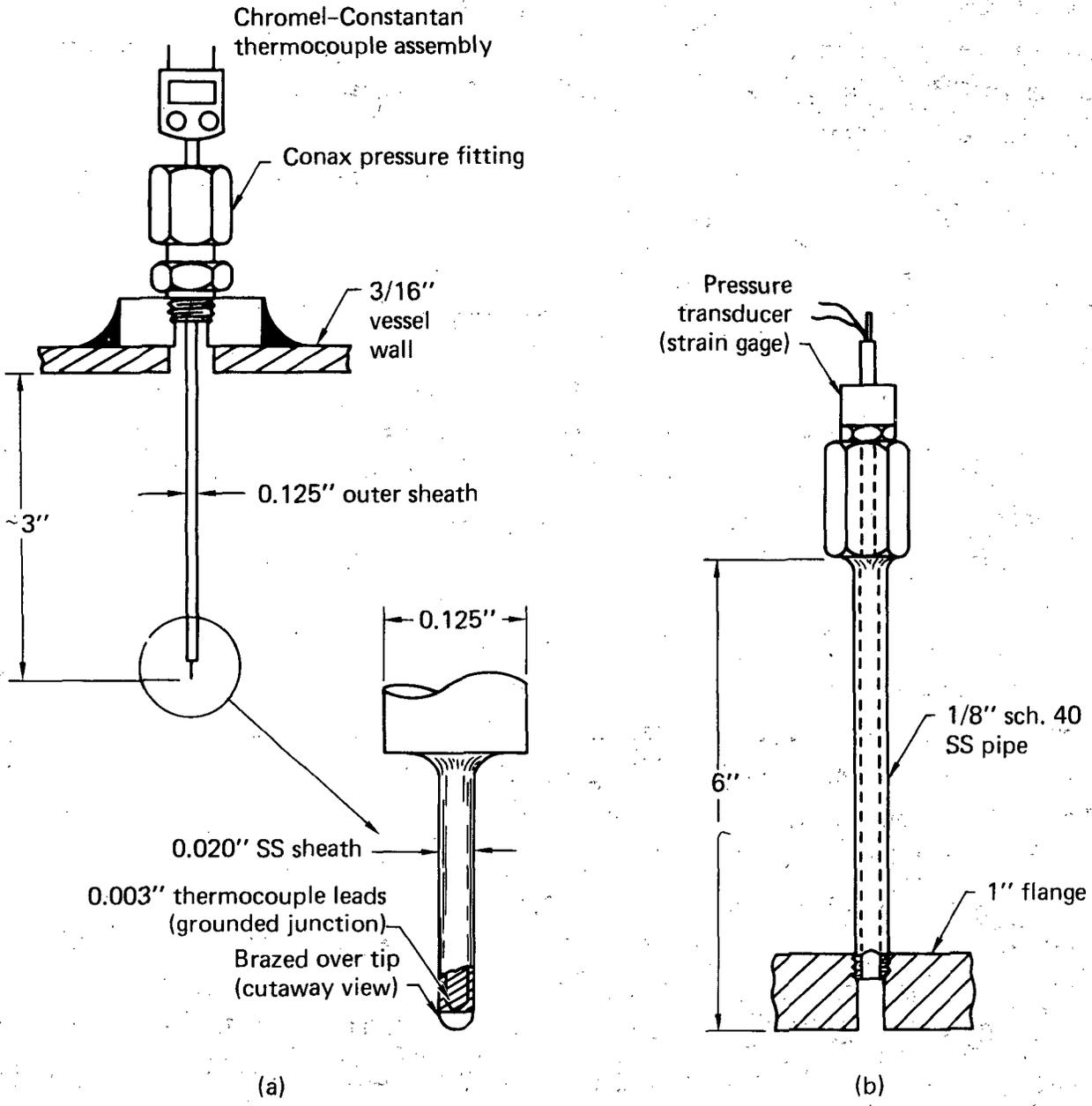
FIG. 6. (a) Vessel mixture temperatures were detected with thermocouples inserted through pressure fittings. (o) Pressure transducers were offset by 6-in. tubes to protect them from thermal transients.
