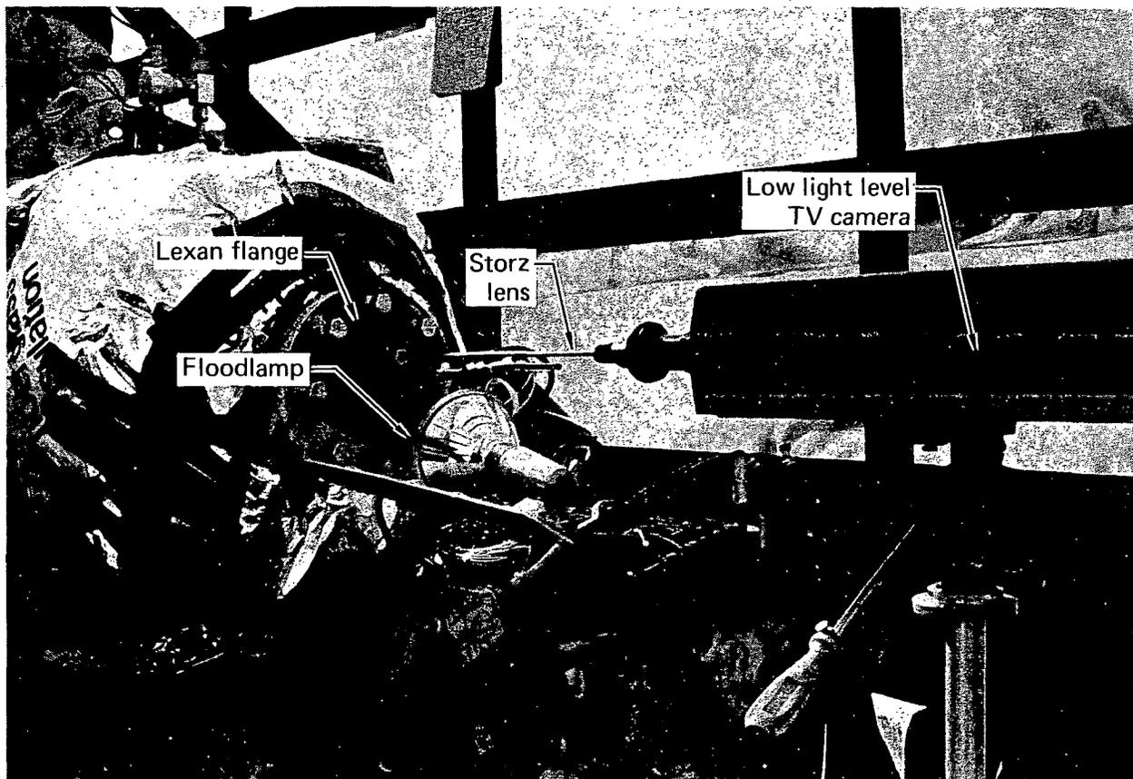
FIG. 15. A Storz lens in conjunction with a low light level television camera was used to film the condensation tests.
