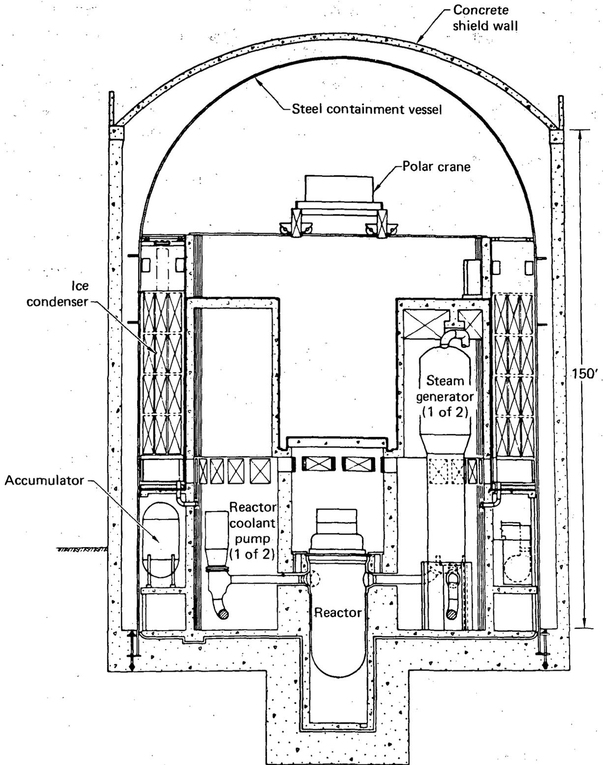
FIG. 1. The Sequoyah Unit 2 containment vessel encloses approximately 1 million cubic feet of free volume. Forty-five igniters are spaced throughout that volume.
