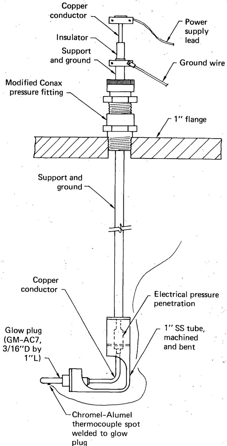
FIG. 4. The glow plug holder could place the plug at various elevations in the center of the vessel.
