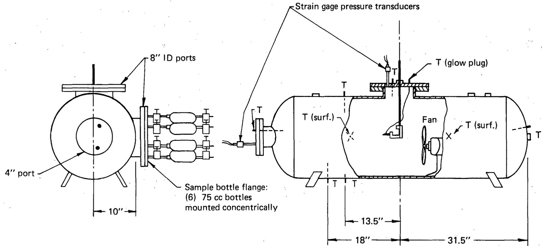
FIG. 5. Primary measurement locations are shown. Thermocouples are indicated by T's.
