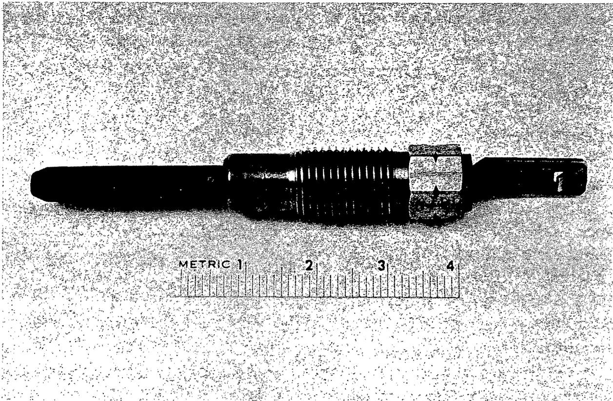
FIG. 2. TVA chose the GM AC-7G glow plug as the thermal ignition source in their Interim Distributed Ignition System (IDIS). The heating element is the 1-in.-long by 3/16-in.-diameter rod on the left.
