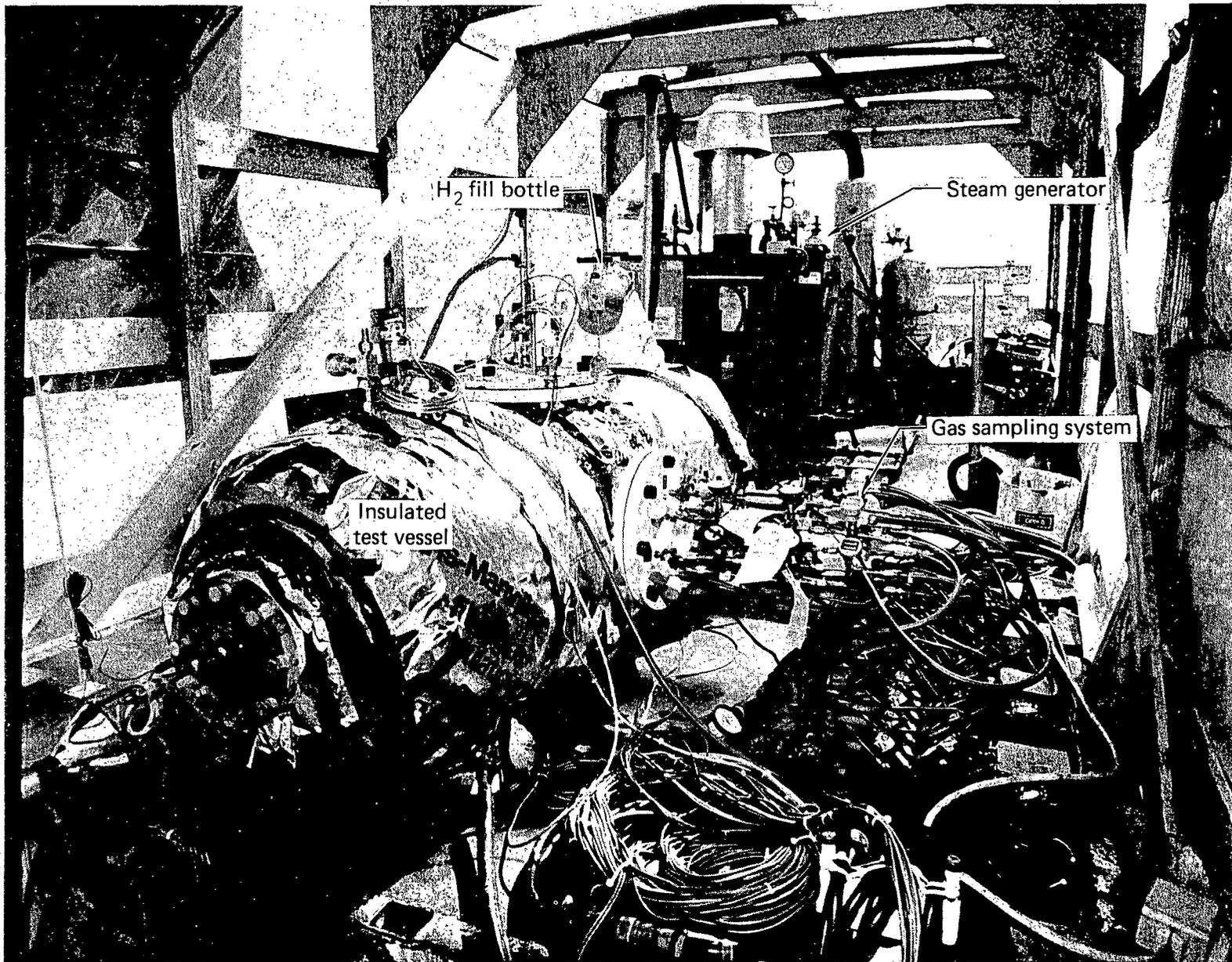
FIG. 8. The experimental assembly was mounted on a trailer and located on a firing table at the Site 300 high explosives test facility.
