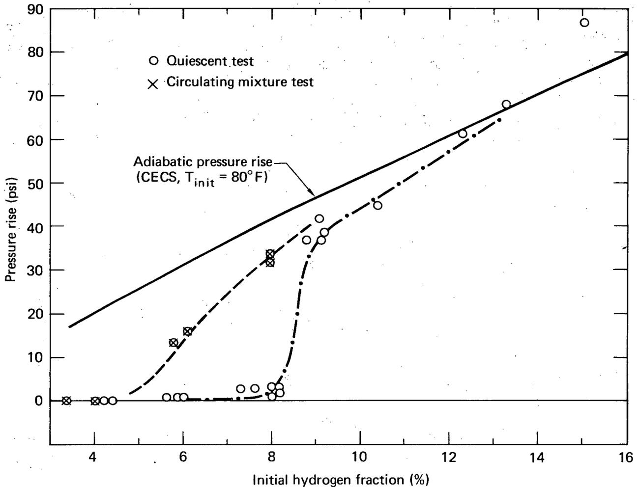
FIG. 9. Pressure rise is shown as a function of hydrogen concentration for dry H<sub>2</sub>/air tests.
