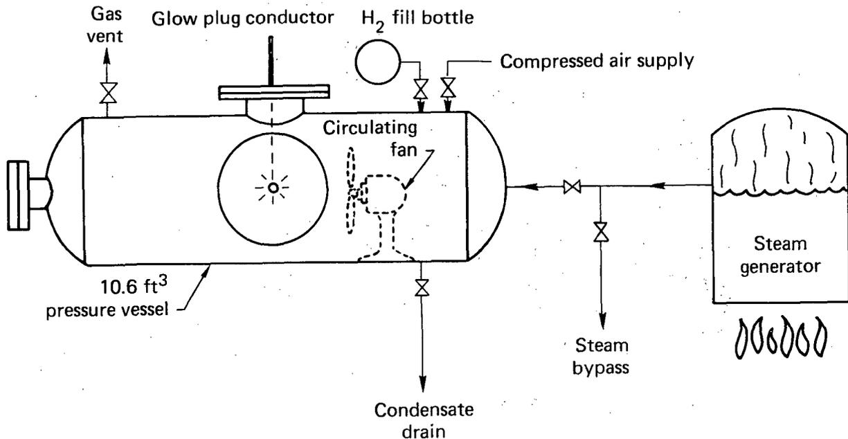
FIG. 3. The LLNL igniter tests were conducted in a modified compressed air storage vessel. The fluid and mechanical systems are shown in schematic form.
