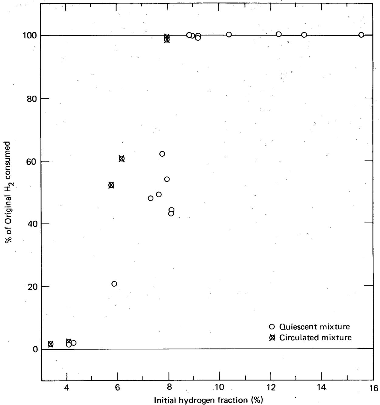
FIG. 11. Burn completion is depicted as percentage of original H<sub>2</sub> consumed for dry tests.
