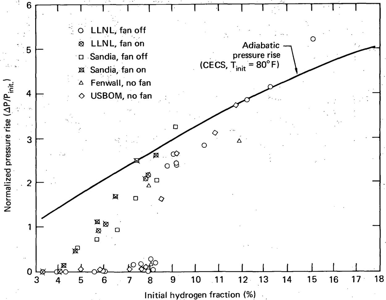
FIG. 10. To compare with results of other test programs, normalized pressure ( $\Delta P/P_{init}$ ) is plotted as a function of  $H_2$  concentration.
