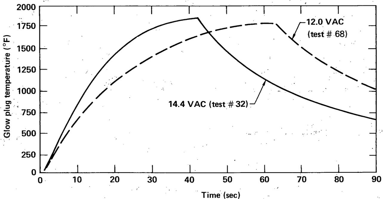
FIG. 12. Glow plug temperature traces are shown for 14.4 VAC and 12.0 VAC voltage levels.
