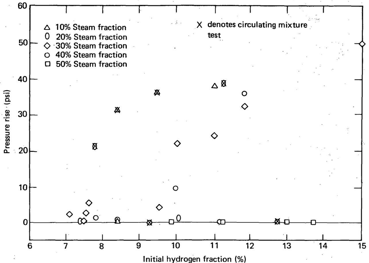
FIG. 13. Pressure rise is shown as a function of  $H_2$  concentration for steam tests.
