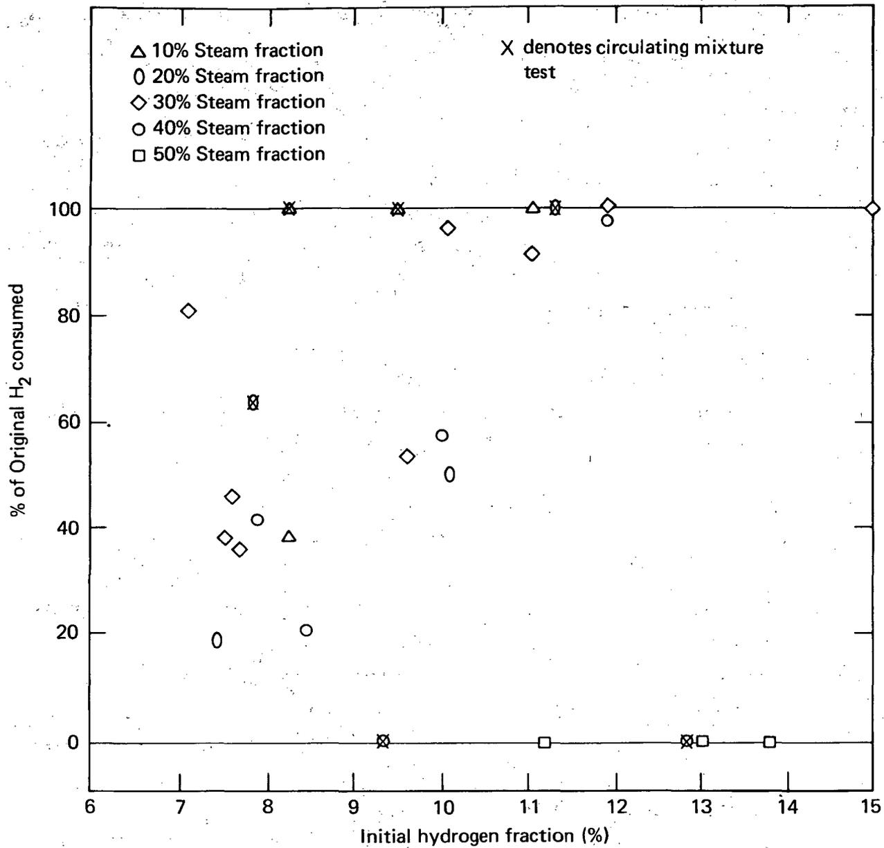
FIG. 14. Burn completion plotted vs. percentage of H<sub>2</sub> for standard steam tests.
