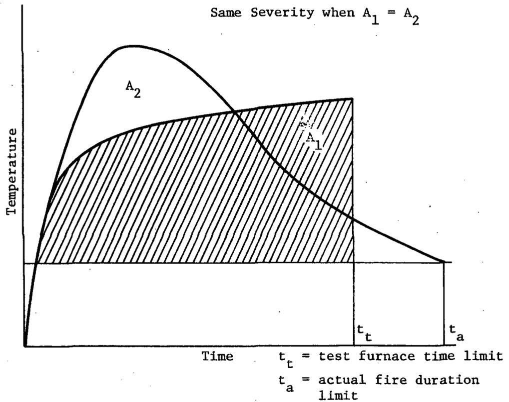
Figure 1. Illustration of Integrated Time-Temperature Curve Concept for Equating Fire Severities
