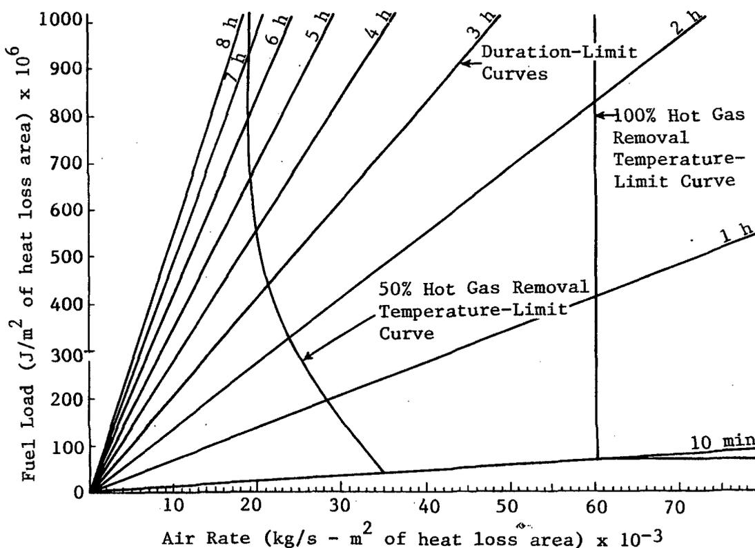
Figure 14. Acceptable Fuel Load and Ventilation Combinations Assuming Heat Loss Into Walls and Either 50% or 100% of Hot Gases Removed
