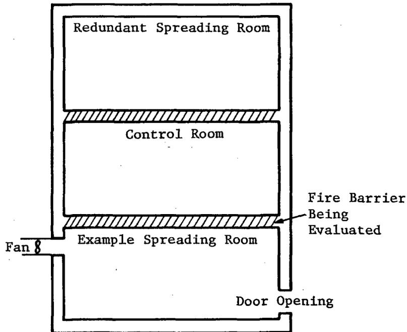
Figure 16. Layout for Fuel Load/Ventilation Barrier Analysis Example
