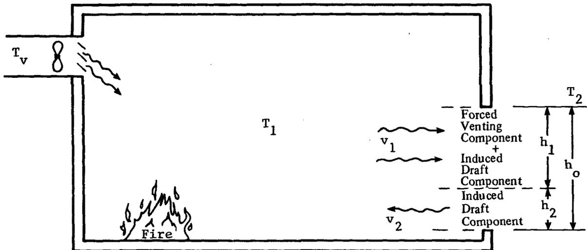
Figure A-1. Combined Case of Induced Draft Plus Forced Ventilation Air Supply
