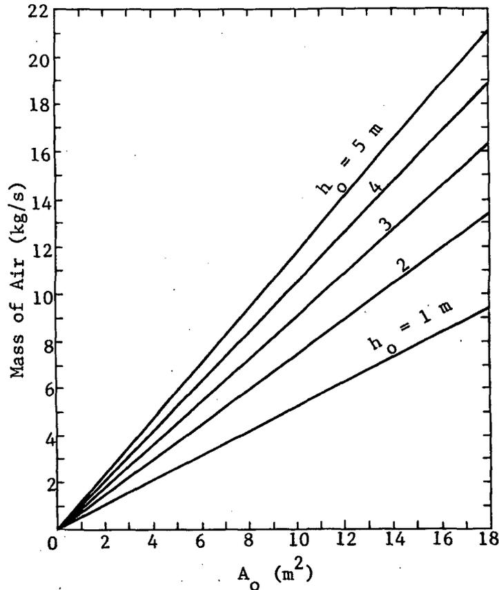
Figure 15. Airflow Rate Induced by a Fire in a Room Having an Opening of Height  $h_o$  and Area  $A_o$
