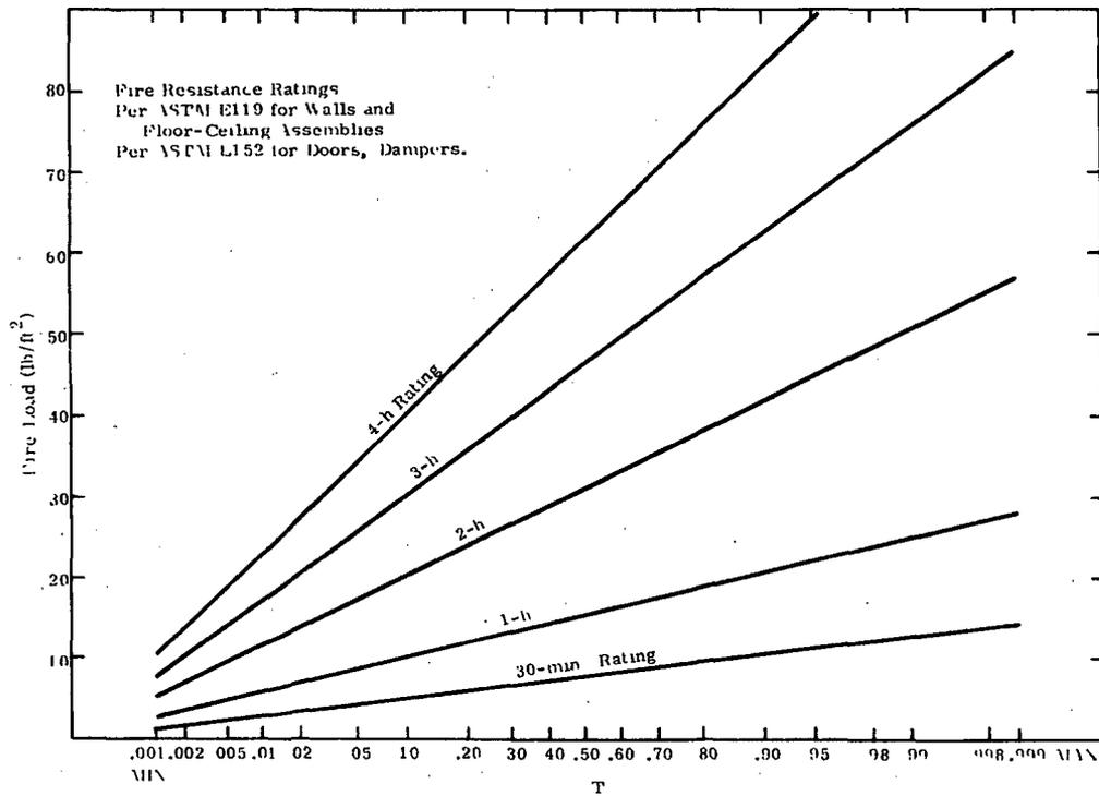
Figure 9. Event T, Fire Barrier "Wearout" Failure
