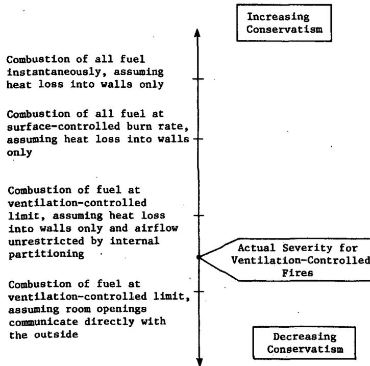
Figure 6. Comparison of Models for Assessing Fire Severity in Nuclear Power Plants
