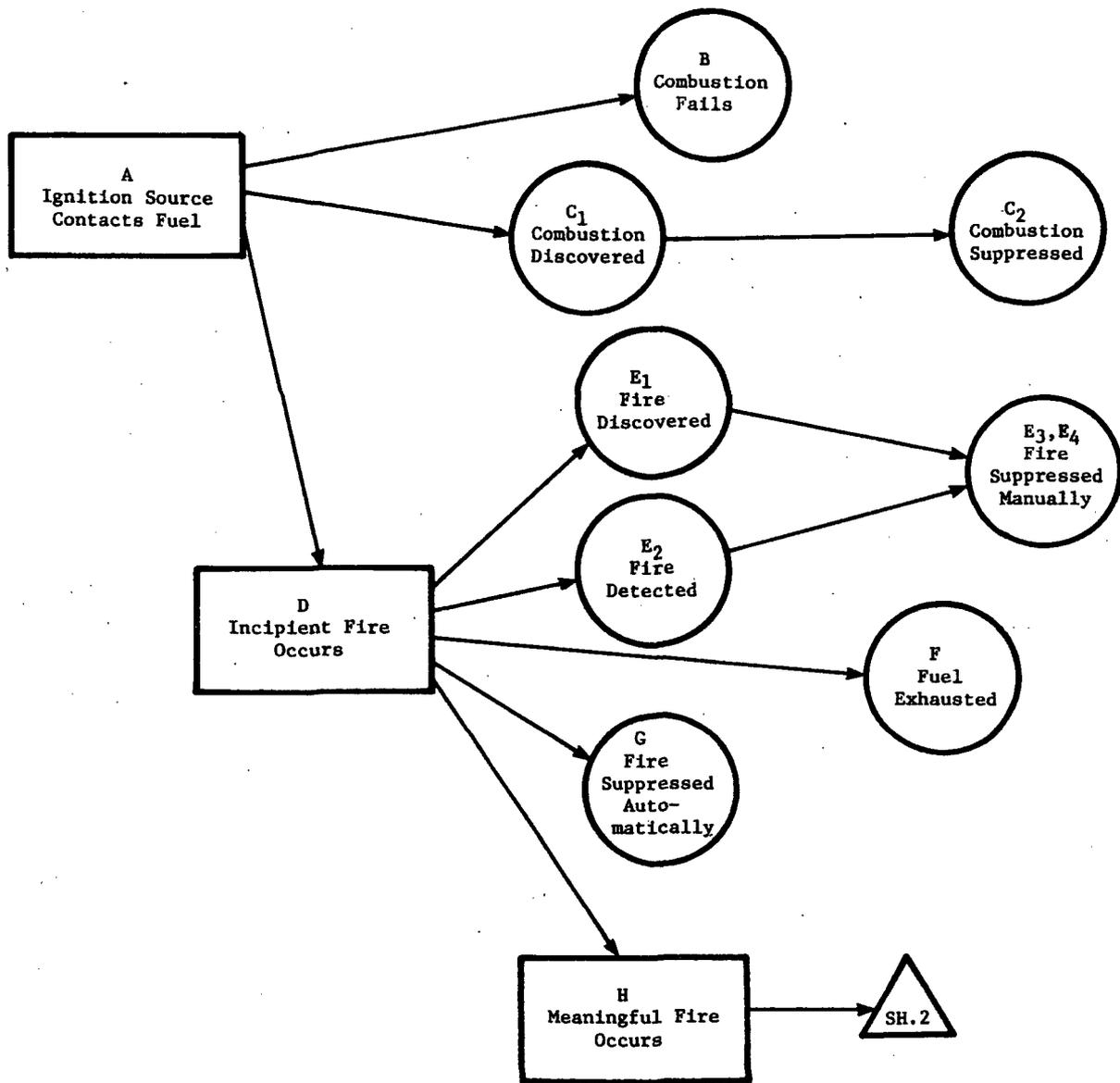
Figure 7. Critical Path Diagram for Fire Development in a Building
