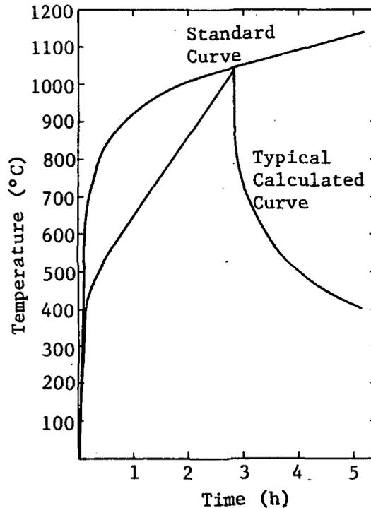
Figure 13. Typical Temperature Limitation for Calculated Time/Temperature Curves
