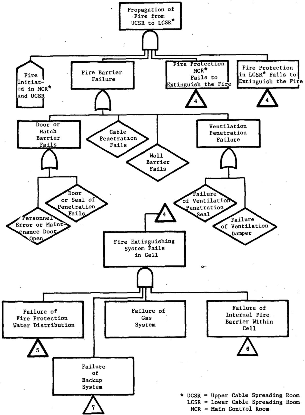
Figure 4. Typical Branches of a Fire-Hazards Analysis Fault Tree
