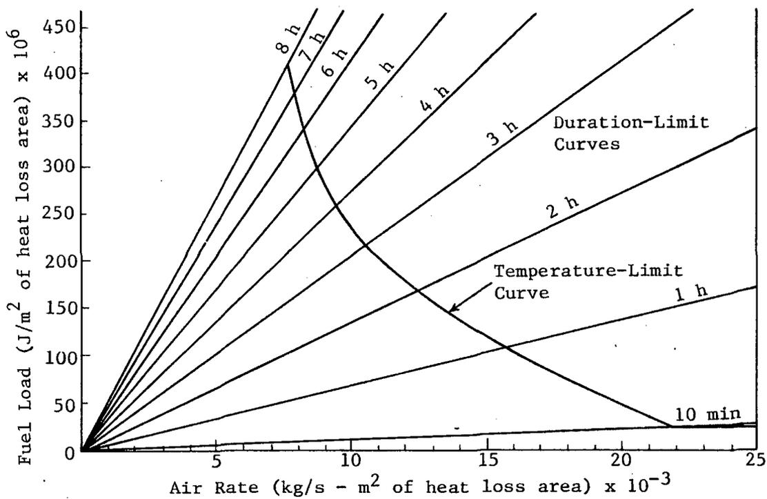
Figure 12. Acceptable Fuel Load and Ventilation Combinations Assuming Heat Loss Into Wall Only
