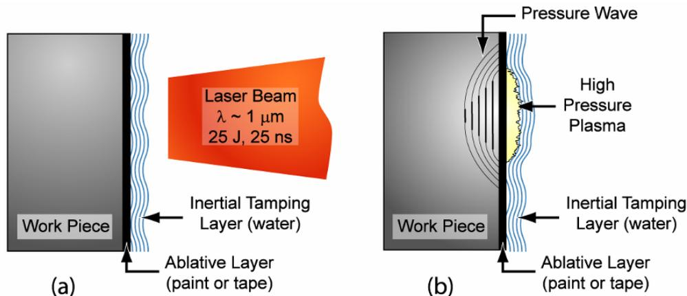
**Laser peening:** (a) Set up of work & (b) A high pressure plasma is generated by the laser impact, resulting in a pressure wave
