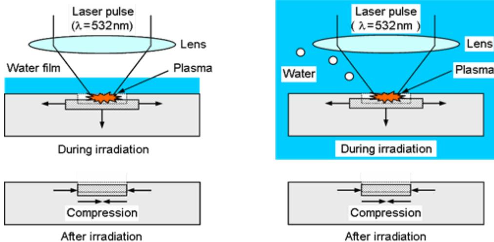
**Fiber laser peening:** Process in air (left) and under water (right)
